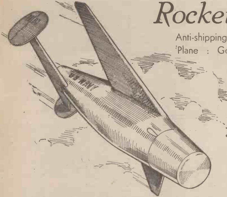
Fig. 73.—The "Bat." This was the first and only missile of the war to incorporate a radar "self-directing" scanner.
