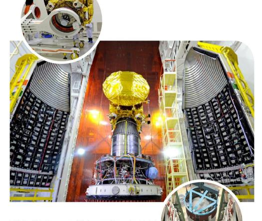
India's Mars Orbiter Mission spacecraft (top) is prepared for a prelaunch test at the Satish Dhawan Space Centre SHAR. Srihairkota in India. The MOM spacecraft (center) is attached to the fourth stage of PSLV-C25 and readied for heat shield closure. The second stage of the PSLV-C25 rocket (bottom) is hoisted into place within the spaceport's Mobile Service Tower.
