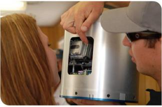
Two days before the launch, students could add critical materials to their experiments through an opening in the side of the payload canister.
