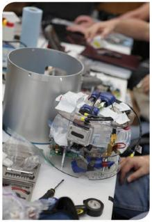
UP Aerospace personnel attached each student team's experiments to Plexiglas shelves that would fit in aluminum payload canisters.
