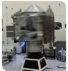
Inside the Payload Hazardous Servicing Facility at Kennedy Space Center in Florida. engineers and technicians perform a spin test of the MAVEN spacecraft. The operation is designed to verify that MAVEN is properly balanced as it spins during the initial mission activities.
