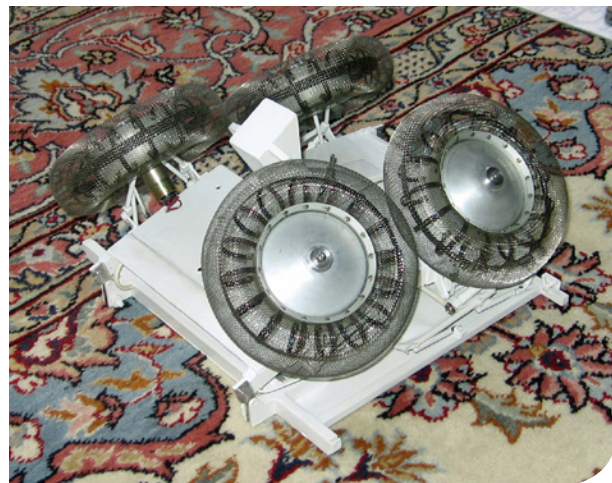
Ferenc Pavlics' original 1/6 scale Lunar Roving Vehicle model, which he drove across the floor of Dr. Wernher von Braun's Huntsville office. The model LRV is folded (right photo) to demonstrate how the full-size Rover could fit into the available space in the Lunar Module descent stage. Credit: David Clow
