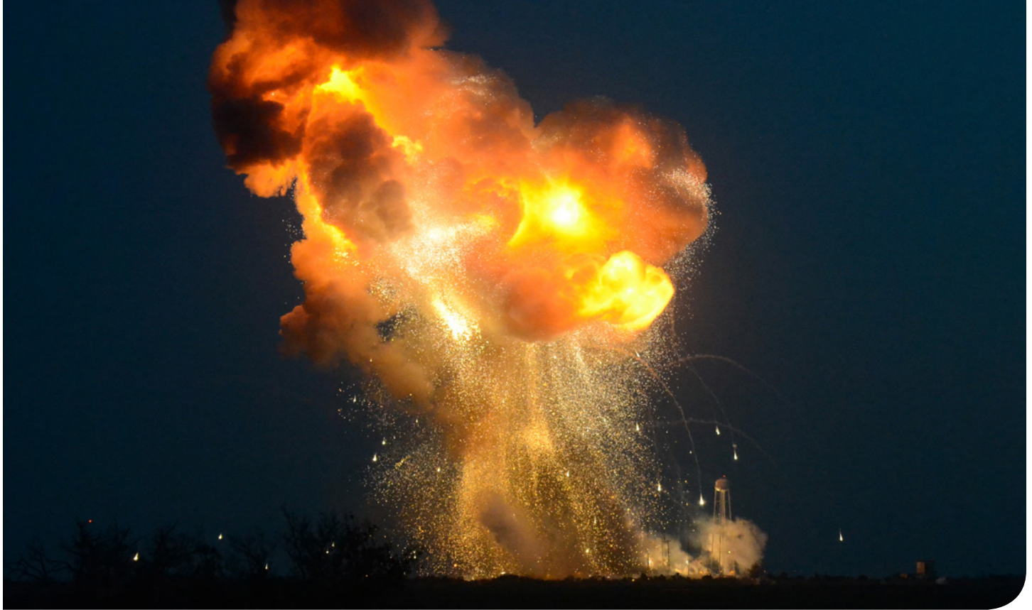
Seconds after liftoff, the ORB-3 Antares rocket fell near the launch pad due to an apparent failure in the turbopump supplying fuel to one of the two first-stage engines. Range Safety Officers engaged the Flight Termination System to stop the remaining engine. Credit: Elliot Severn
