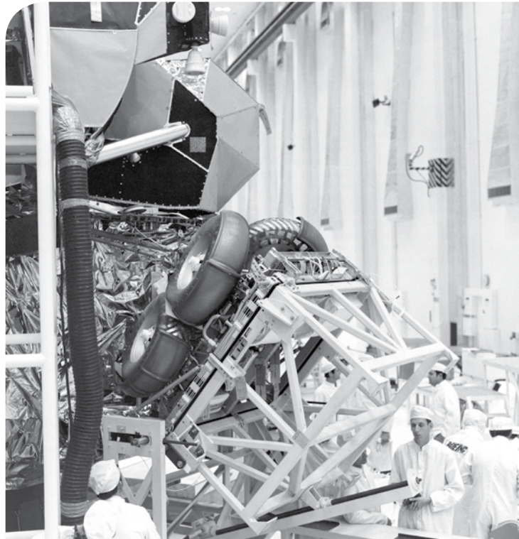
The Lunar Rover is folded up and being moved into its stored position inside the Apollo 15 Lunar Module, where it will remain until its deployment on the Moon's surface.
