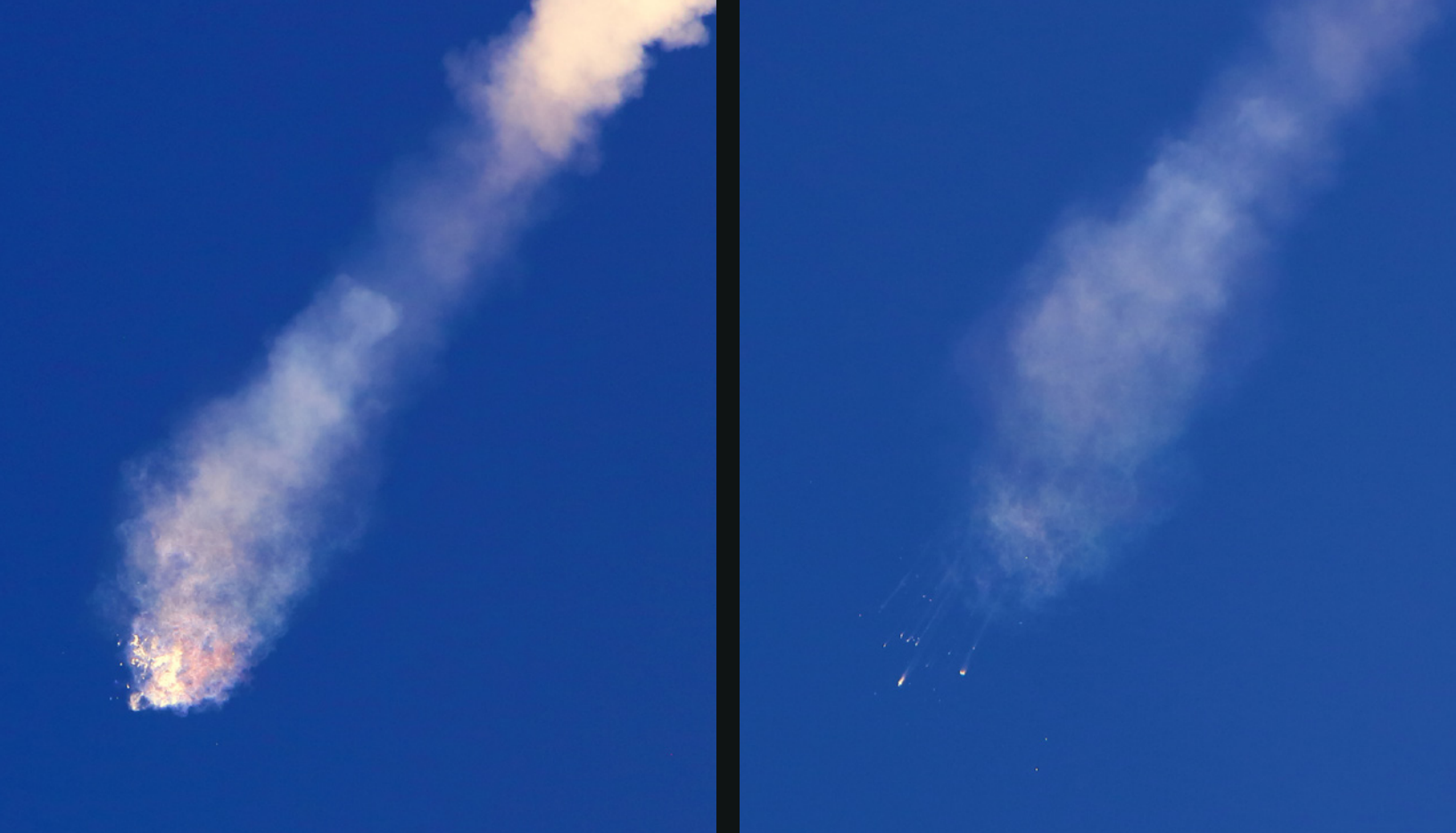
The SpaceX Falcon 9 rocket carrying the Dragon capsule on the CRS-7 resupply mission to the International Space Station suffered a failure of the second stage and disintegrated seconds after passing through maximum aerodynamic pressure. The rocket and cargo are presumed to be a total loss. Credit: Alan Waters/AmericaSpace
