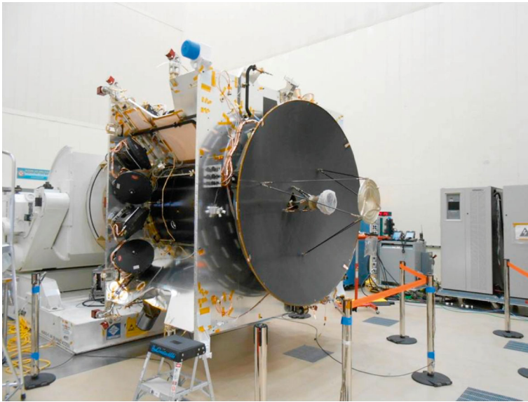
Fig. 8 Nearly completely assembled MAVEN spacecraft, showing the open-bay construction. The bay that is visible contains the four reaction wheels, oriented parallel to the four top faces of a pyramid
