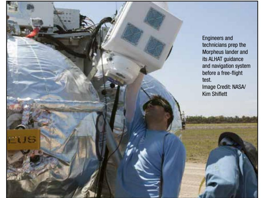
Engineers and technicians prep the Morpheus lander and its ALHAT guidance and navigation system before a free-flight test. Image Credit: NASA/Kim Shiflett
