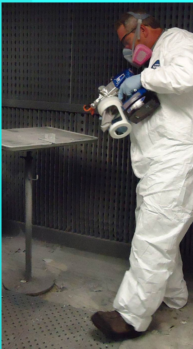
A technician sprays a protective coating on a sample panel for testing at the Beachside Atmospheric Test Facility at NASA's Kennedy Space Center. Photo credit: NASA/Jerry Curran
