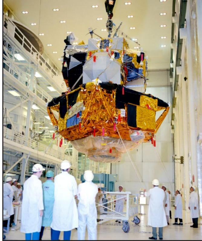
A crane is used to move the lunar module for the Apollo 12 mission on June 23, 1969. In November that year, Apollo 12 would complete the second mission to land humans on the moon. Photo credit: NASA
