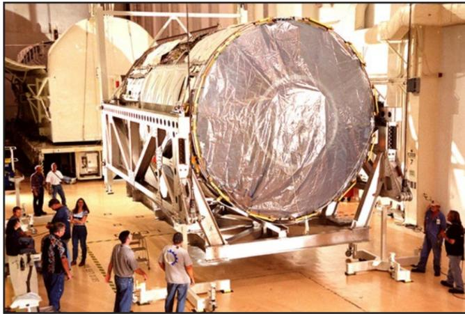
In the Operations and Checkout Building on June 30, 2000, the U.S. laboratory module, a component of the International Space Station, is lifted off the floor to be raised to a vertical position. The lab, named Destiny, underwent testing in the altitude chamber in the O&C. Photo credit: NASA
