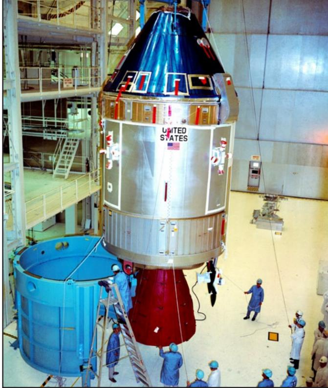
The Apollo 11 command/service module is being moved from a work stand during spacecraft processing in the high bay of the Manned Spacecraft Operations Building on April 11, 1969. Photo credit: NASA
