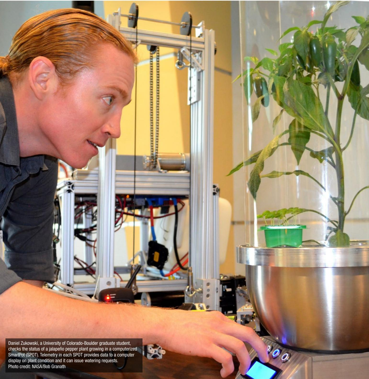
Daniel Zukowski, a University of Colorado-Boulder graduate student, checks the status of a jalapeño pepper plant growing in a computerized SmartPot (SPOT). Telemetry in each SPOT provides data to a computer display on plant condition and it can issue watering requests. Photo credit: NASA/Bob Granath
