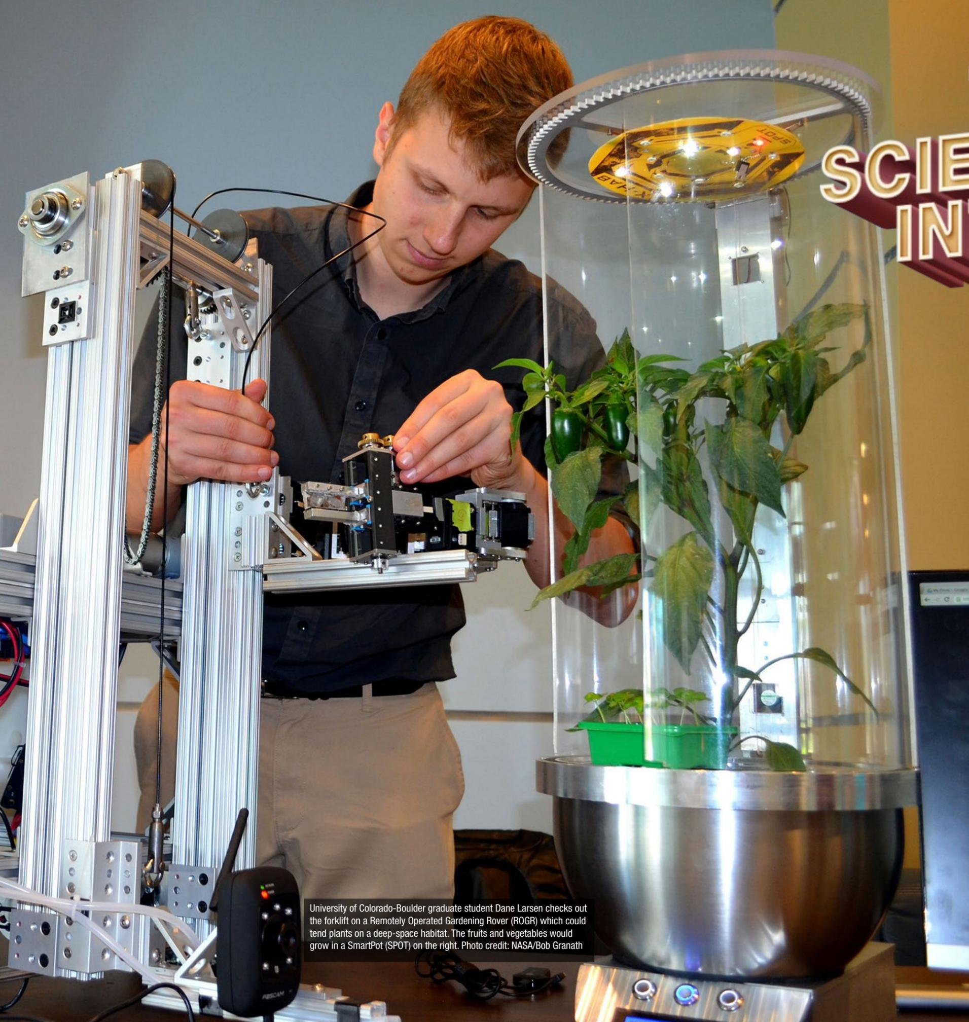
University of Colorado-Boulder graduate student Dane Larsen checks out the forklift on a Remotely Operated Gardening Rover (ROGR) which could tend plants on a deep-space habitat. The fruits and vegetables would grow in a SmartPot (SPOT) on the right. Photo credit: NASA/Bob Granath
