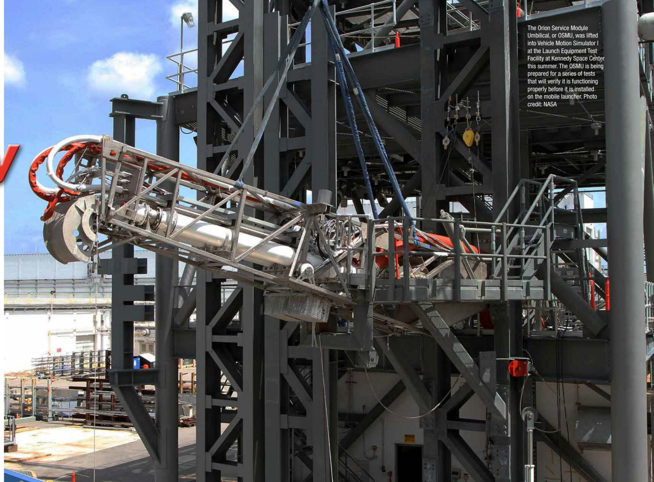
The Orion Service Module Umbilical, or OSMU, was lifted into Vehicle Motion Simulator 1 at the Launch Equipment Test Facility at Kennedy Space Center this summer. The OSMU is being prepared for a series of tests that will verify it is functioning properly before it is installed on the mobile launcher. Photo credit: NASA
