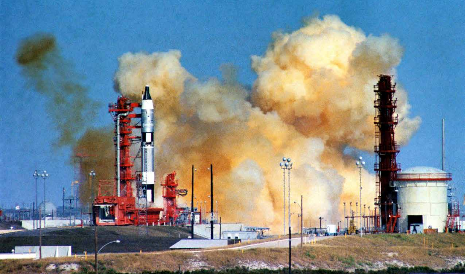
Gemini VI's Titan first stage engines shut down 1.5 seconds after ignition on Dec. 12, 1965 due to a premature release of a liftoff umbilical plug. Wally Schirra and Tom Stafford successfully launched to a rendezvous with Gemini VII three days later. Photo credit: NASA
