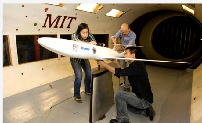
Professor Mark Drela, center, chief engineer of a Massachusetts Institute of Technology aircraft design team, helps undergraduate students Nina Siu, left, and Mike Lieu position a model of the D8 “double bubble” in a wind tunnel at MIT. The team, which includes Aurora Flight Sciences and Pratt & Whitney, designed the concept. The D8 series aircraft would be used for domestic flights and is designed to fly at Mach 0.74 carrying 180 passengers 3,000 nautical miles in a coach cabin roomier than that of a Boeing 737-800. Photo credit: NASA/MIT
