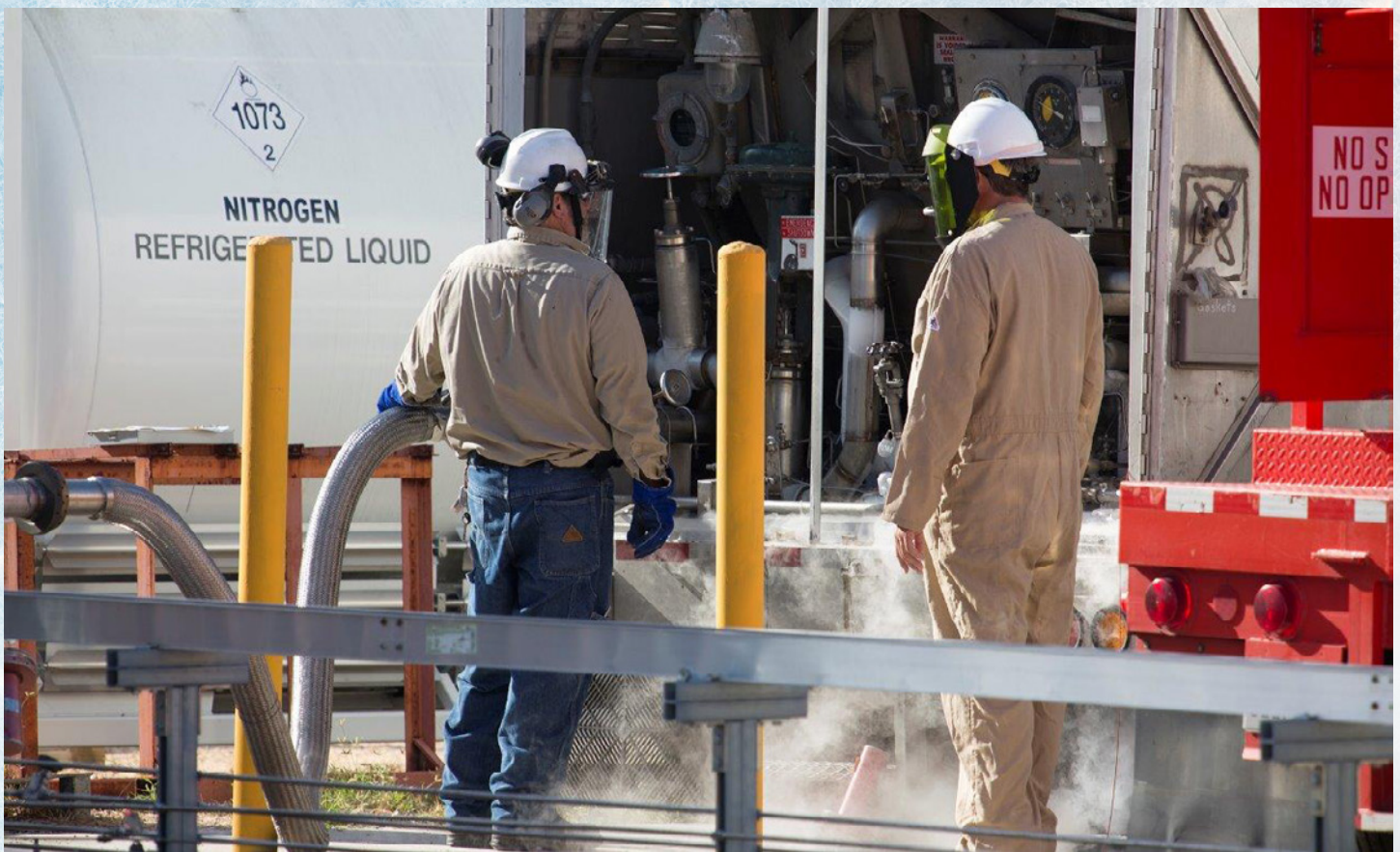
Technicians with Praxair pressurize the hydrogen trailer before offloading liquid hydrogen during a test of the Ground Operations Demo Unit for liquid hydrogen at Kennedy Space Center. The system includes a 33,000-gallon liquid hydrogen storage tank with an internal cold heat exchanger supplied from a cryogenic refrigerator. The primary goal of the testing is to achieve a liquid hydrogen zero boil-off capability. The system was designed, installed and tested by a team of civil servants and contractors from the center's Cryogenic Test Laboratory, with support from engineers at NASA's Glenn Research Center in Cleveland and Stennis Space Center in Mississippi. It may be applicable for use by the Ground Systems Development and Operations Program at Launch Pad 39B. Photo credit: NASA/Cory Huston
