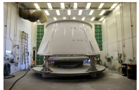
The right-hand aft skirt for NASA's Space Launch System (SLS) rocket has been refurbished, was painted Oct. 31, and is in a drying cell in a support building at Hangar AF at Cape Canaveral Air Force Station in Florida. Photo credit: NASA/Kim Shifflett
