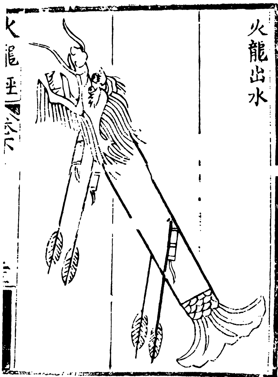
Fig. 214. The first of all multi-stage rockets, the 'fire-dragon issuing from the water' ( huo lung chhu shui ), a device from HLC , pt. 1, ch. 3, p. 23 a . It therefore belongs to the middle, perhaps to the beginning, of the +14th century. It was a two-stage rocket, for when the carrier or booster rockets were about to burn out they automatically ignited a swarm of smaller rocket-arrows which issued through the dragon mouth and fell down upon the enemy. The design seems to have been for use mainly in naval warfare, and as the trajectory was very flat the weapon may be regarded as an ancestor of the modern 'Exocet'
