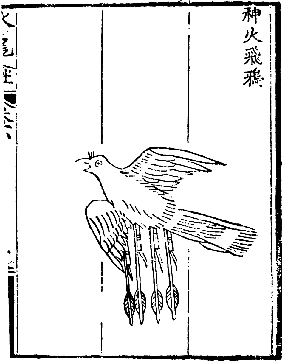
Fig. 208. A winged rocket-bomb, the 'flying crow with magic fire' ( shen huo fei ya ) from HLC , pt. 1, ch. 3, p. 18a, and therefore at least as early as +1350, probably a century earlier. The idea was doubtless derived from the use of expendable birds (Fig. 38) carrying glowing tinder wherewith to set on fire the roofs of the enemy city. But the provision of wings or fins for increasing aerodynamic stability long preceded anything of the same kind elsewhere in the world. And the provision of an explosive payload was also a new development.
