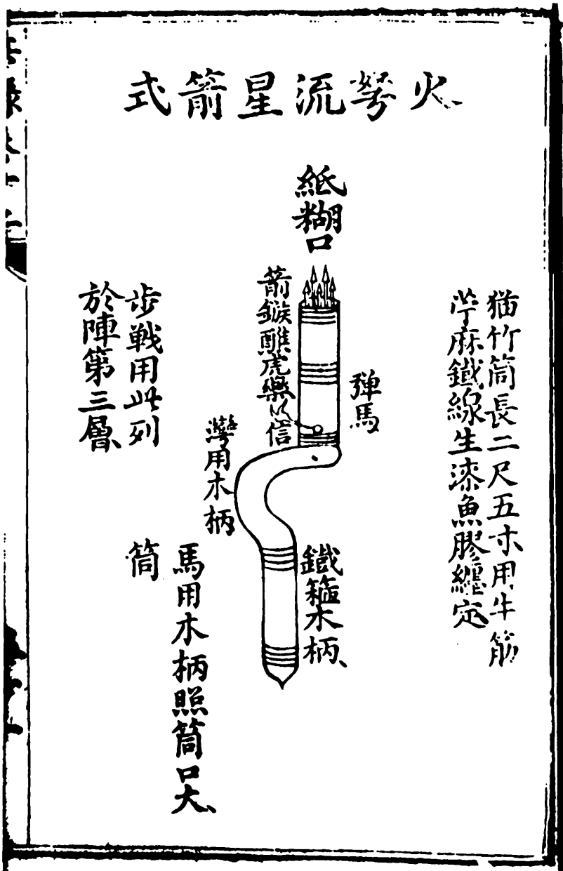
Fig. 217. Another example of a weapon which though called 'meteoric' had nothing to do with rockets, the 'fire-crossbow meteoric arrow-shooter' ( huo nu liu hsing chien ), nor did it have anything to do with crossbows either. It was a bamboo fire-lance or proto-gun which shot forth arrows as co-viative projectiles. PL , ch. 12, p. 51a.
