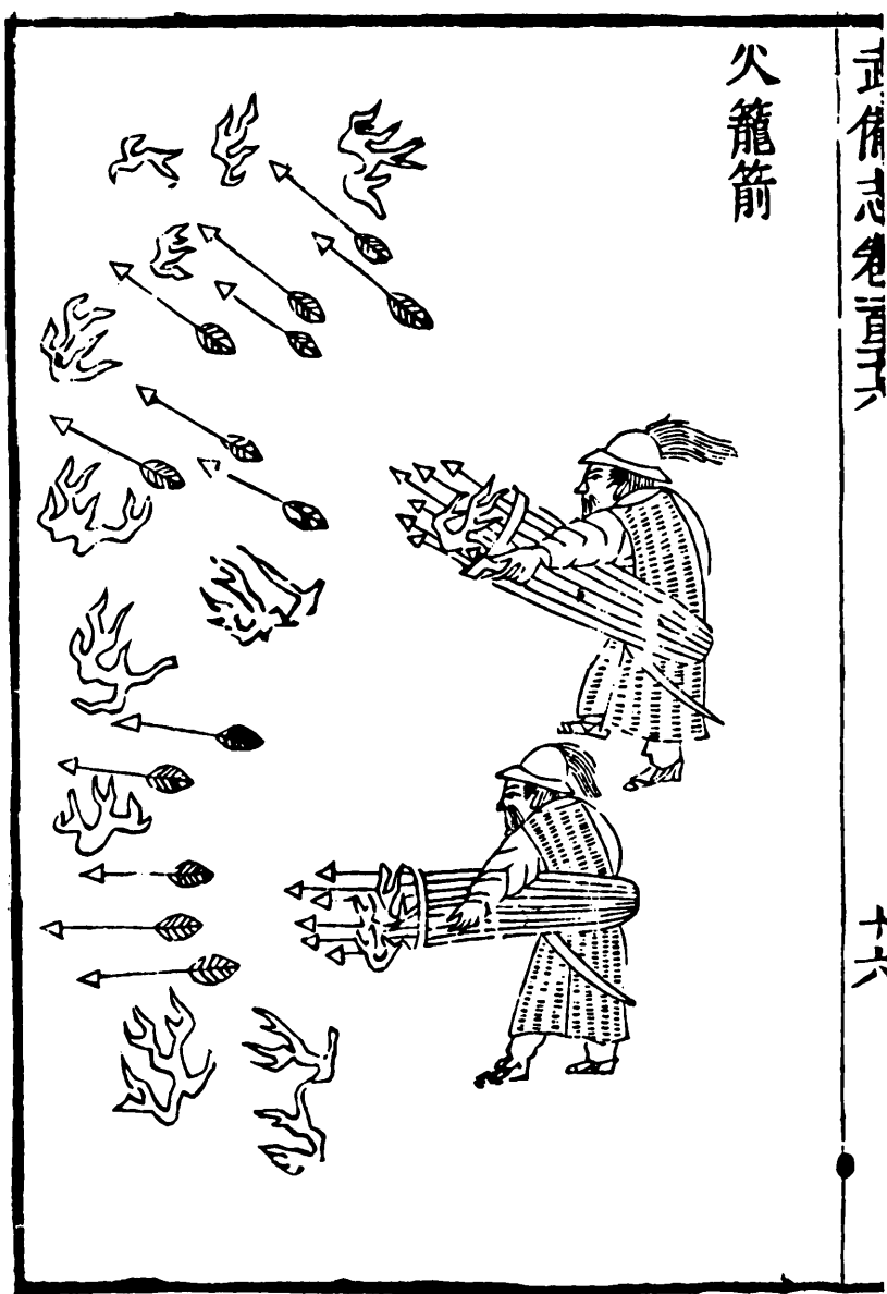
Fig. 198. Conical rocket-arrow launchers made of basketwork ( WPC , ch. 126, p. 166).
