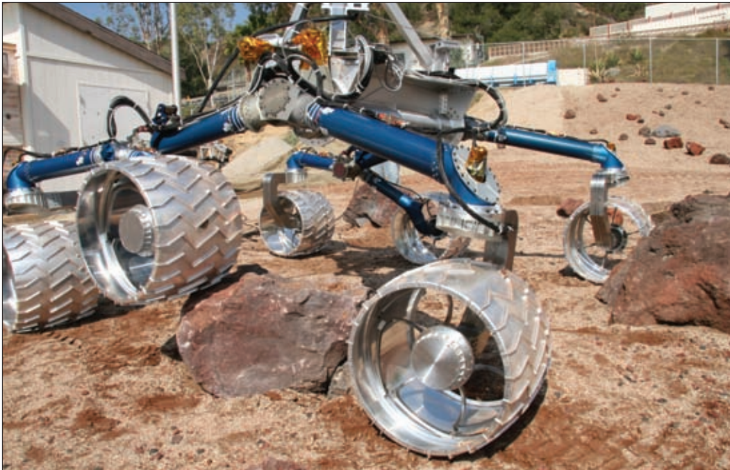
Engineers took the MSL rover for a test drive in the lab. The “Scarecrow” engineering model, so named because it was still missing its computer brain, easily traversed large rocks in JPL’s “Mars Yard.”
