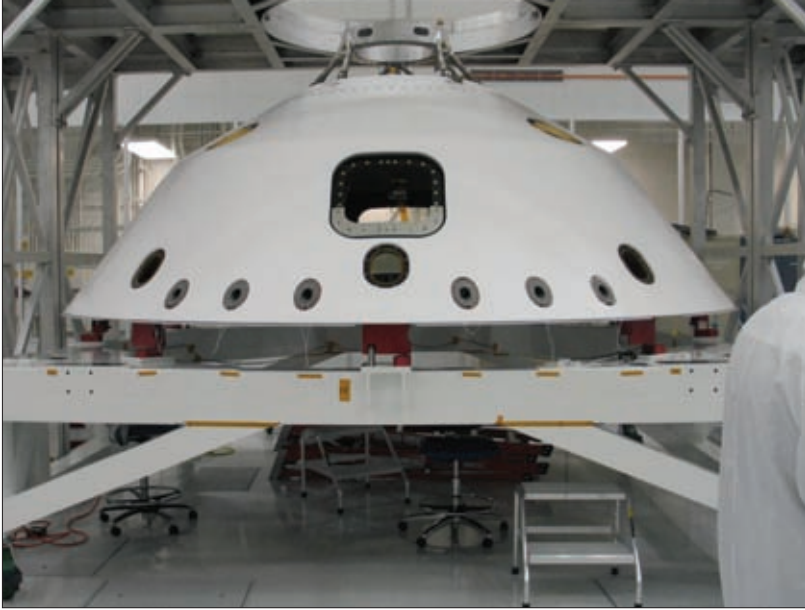
Like two pieces of a giant clam, the aeroshell's backshell (above) and heat shield (below) come together to protect the rover and the propulsion stage that safely delivers it to the surface of Mars.
