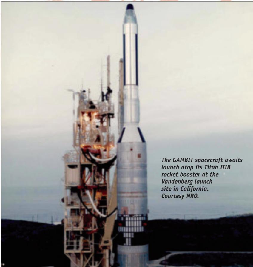
*The GAMBIT spacecraft awaits launch atop its Titan IIIB rocket booster at the Vandenberg launch site in California. Courtesy NRO.*
