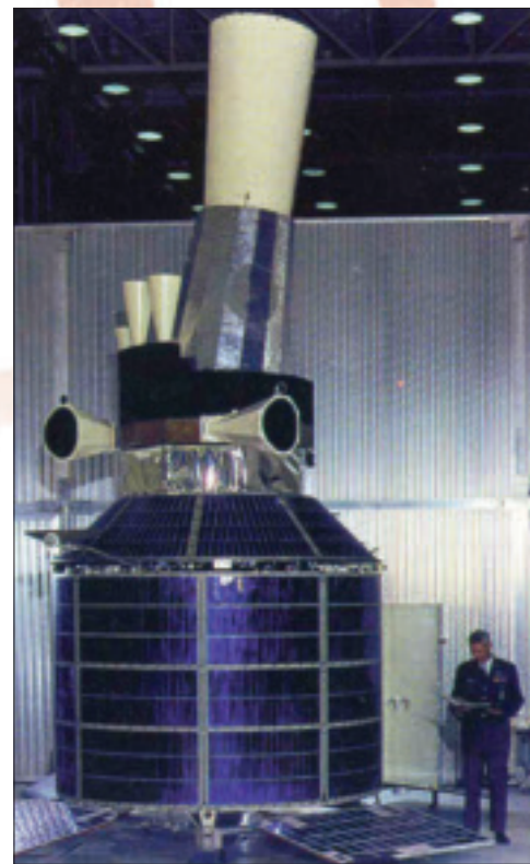
A DSP satellite, also known as Project 647, undergoes testing on the manufacturer's premises in southern California. The long telescope tube contained the infrared sensor that tracked, as well as registered, rocket and missile launches from Tyuratam and elsewhere. This photograph depicts Flight 1, the vehicle that recorded the entire June 1971 SL-X launch failure from Tyuratam—from the rocket's launch to its crashing back on the steppe. The telescope tube pointed down at the Earth. At the base of the satellite are solar panel arrays that helped to power the spacecraft. Courtesy USAF.
