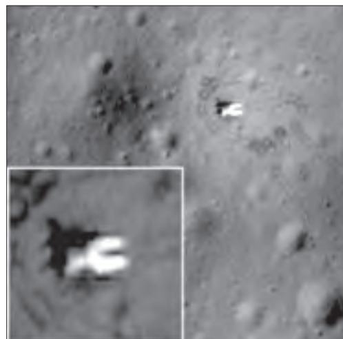
Missing on the Moon for 42 years, the Lunokhod 1 lunar rover and the Soviet Luna 17 lander that carried it to the lunar surface in 1970 were found by LRO. Note the fork-like ramps on which the rover descended to the surface and the rover tracks surrounding the lander. LRO found Lunokhod 1 about 6.5 mi. from the lander near the center of the Imbrium Basin. Credit NASA Goddard/Arizona State.
