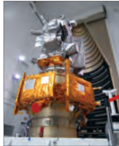
The Lunar Reconnaissance Orbiter, wrapped in silver insulation, sits atop the gold insulation wrapped LCROSS impact spacecraft before both were attached to Atlas V Centaur upper stage at Cape Canaveral. Credit: NASA KSC.
