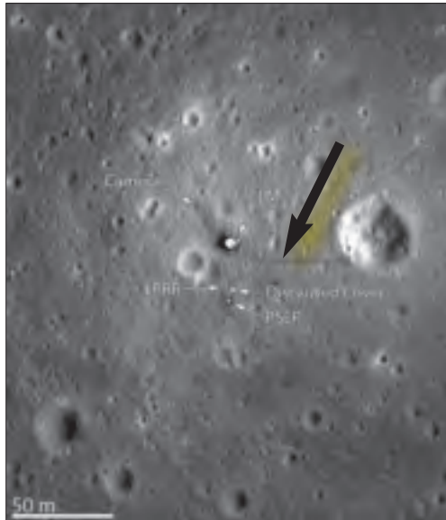
LRO image of the Apollo 11 landing site from an altitude of only 12 mi., with an 8-in. resolution, shows the tracks of Neil Armstrong (dark arrow) created when he walked 200 ft each way to the 80-ft-diam. Little West crater. Visible are Eagle's descent stage, the lunar ranging retroreflector, and the passive seismometer experiment.
