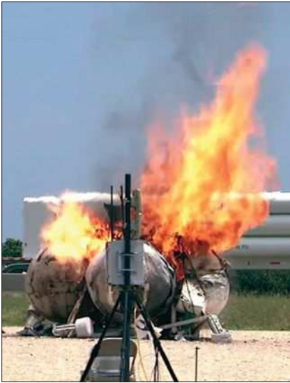
The Morpheus lander was built to carry the ALHAT equipment. On August 9 it rose a short distance, veered off course, and crashed.
