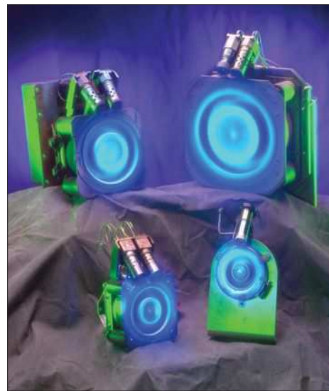
Various Soviet and Russian SPT Hall thrusters have been developed over the years.
