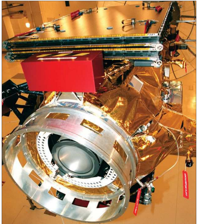
Three heritage Deep Space 1 ion propulsion engines were used to power the Dawn spacecraft.
