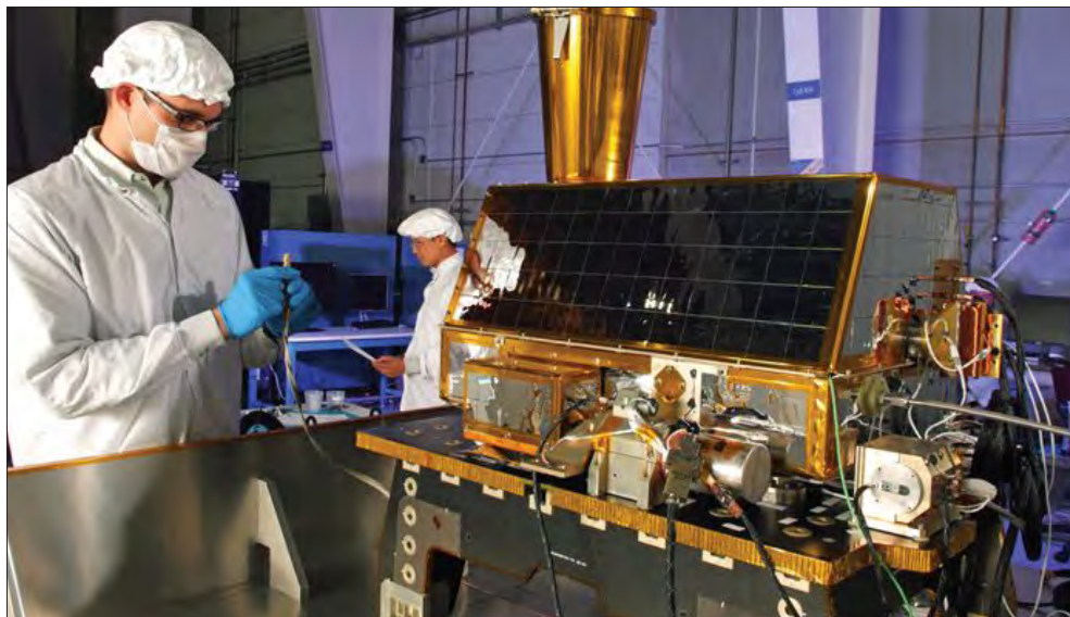
CHIRP (commercially hosted infrared payload) was installed on the SES-2 commercial satellite. Credit: SES Government Solutions.
