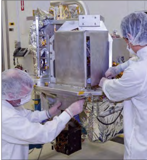
Technicians prep the OCO-2 instrument for shipping. Credit: NASA/JPL-Caltech
