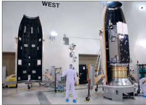
The two large segments of OCO-2's fairing, or outer shell. Credit: NASA
