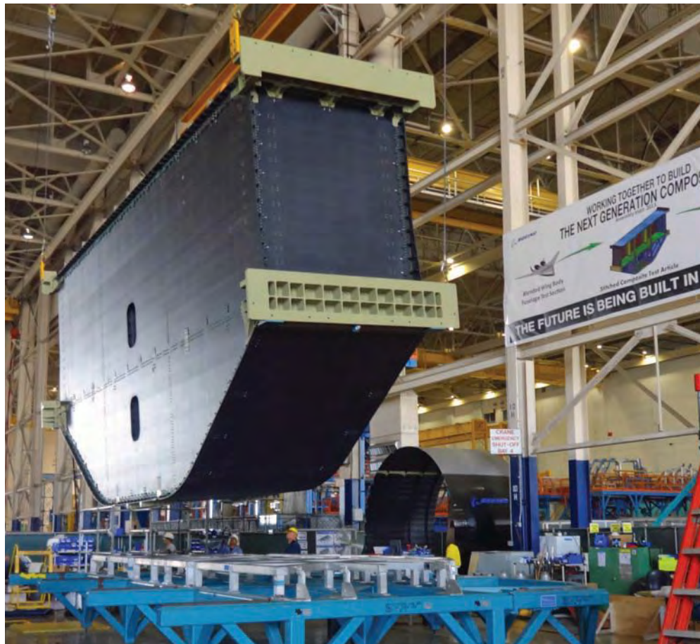
A cross-section of a blended wing body, built at Boeing's facility in Long Beach, California, will be used to test stitched construction.
