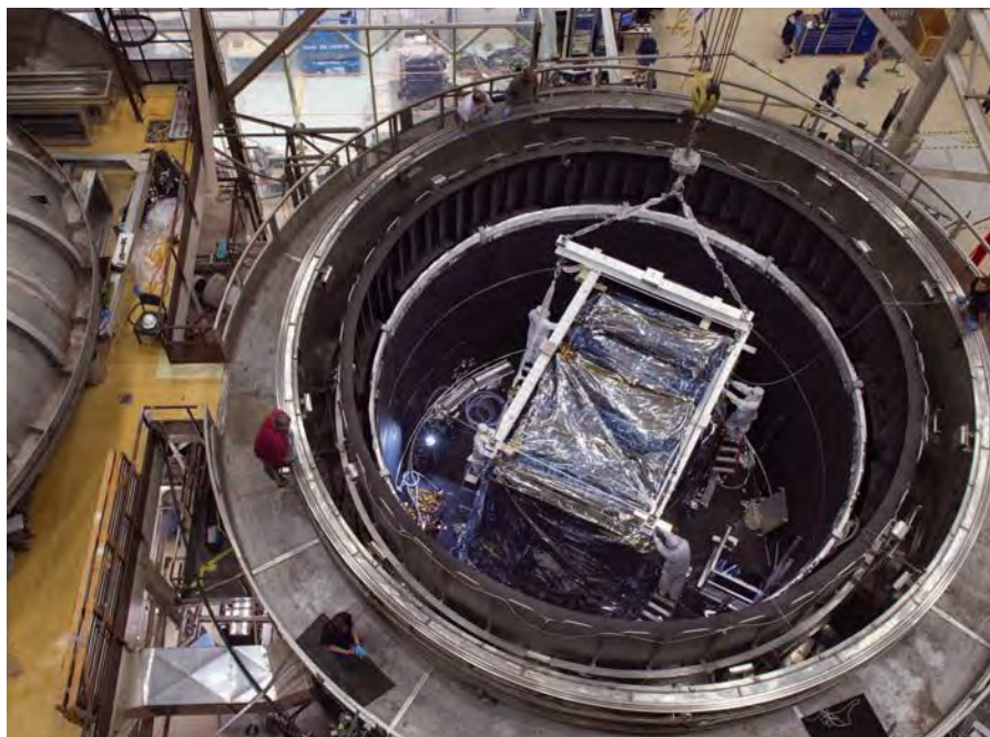
The James Webb Space Telescope’s science instrument module undergoes cryogenic vacuum testing at NASA’s Goddard Space Flight Center in Maryland in 2014.
