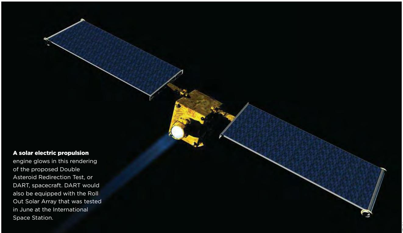
**A solar electric propulsion** engine glows in this rendering of the proposed Double Asteroid Redirection Test, or DART, spacecraft. DART would also be equipped with the Roll Out Solar Array that was tested in June at the International Space Station.
