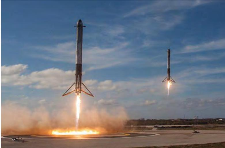
▲ **Reusing rocket components**, like the two SpaceX Falcon Heavy side boosters that landed in Florida in February, promises dramatic reductions in launch costs for the communications satellite industry. SpaceX recovered two of three boosters in the Falcon Heavy's debut. The center core rocket was lost at sea when its drone-ship landing failed.
