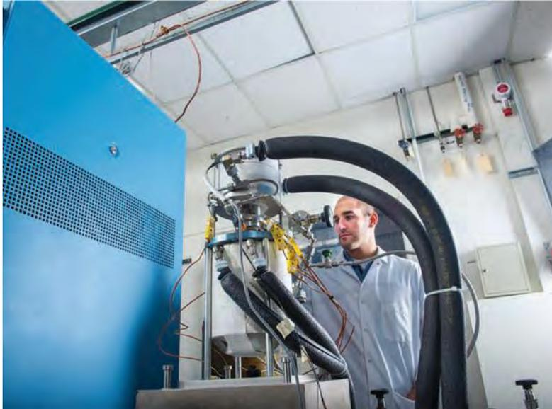
▲ **This experimental Stirling engine** has operated at full power for nearly 13 years at NASA's Glenn Research Center in Ohio.
