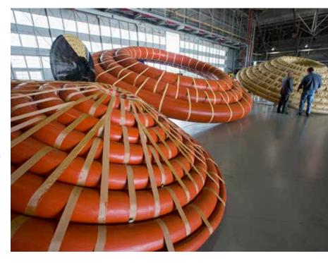
ifornia. Engineers pumped compressed water into the doughnutlike tubes while they were submerged in a pool of water to test how much pressure they could withstand.
