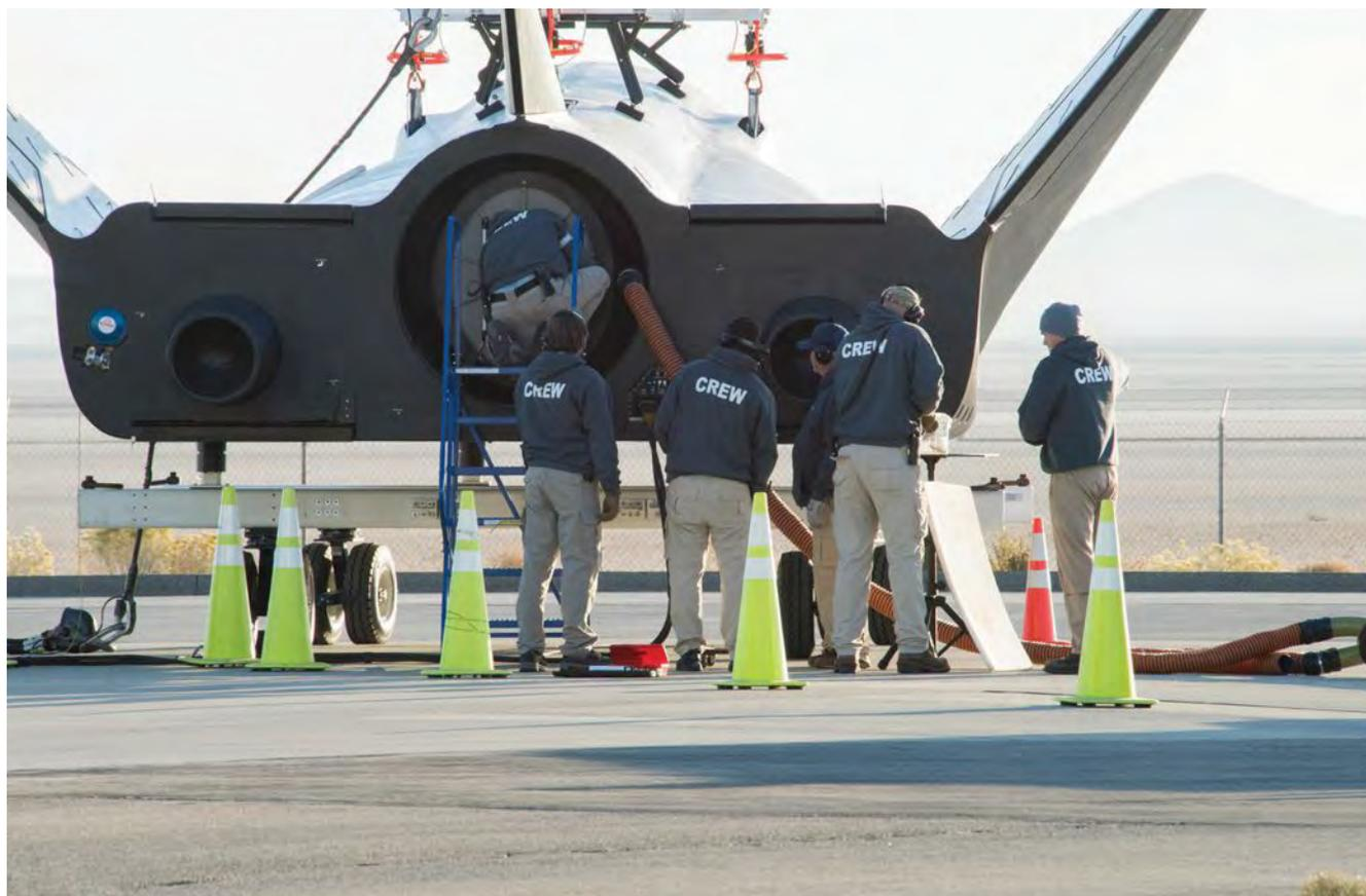
The HL-20's lifting-body design — lift is generated by the spacecraft's body instead of wings — meant it could land on a runway.
