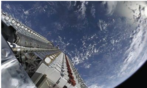
◀ A frame from the video feed of SpaceX Falcon 9 upper stage shows a stack of 60 Starlink smallsats moments before they're deployed. SpaceX
