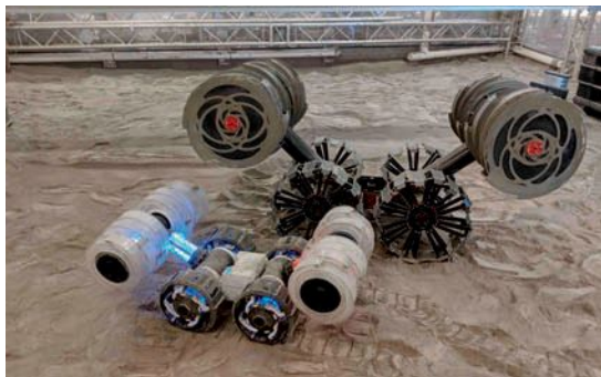
◀ The MiniRASSOR and the larger RASSOR 2.0, low-gravity excavators designed for educational outreach. NASA
