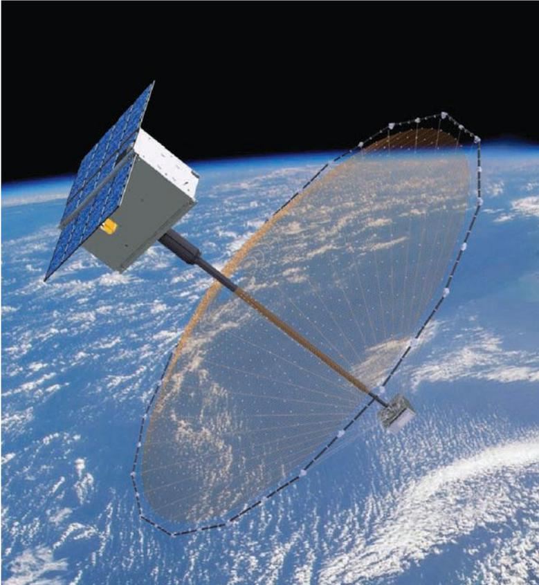
▲ **Artist's rendering of** L3Harris' 5-meter-diameter High Compaction Ratio antenna. The design scales from a 1-meter-diameter dish that fits into a cubesat volume to the 5-meter-diameter dish shown here, which in stowed form takes up one-tenth of a cubic meter, a fraction of a small-satellite volume.
