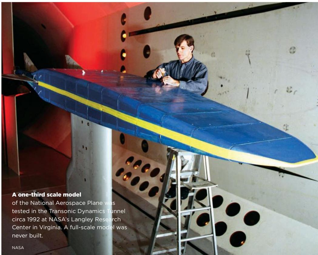
**A one-third scale model** of the National Aerospace Plane was tested in the Transonic Dynamics Tunnel circa 1992 at NASA's Langley Research Center in Virginia. A full-scale model was never built.
