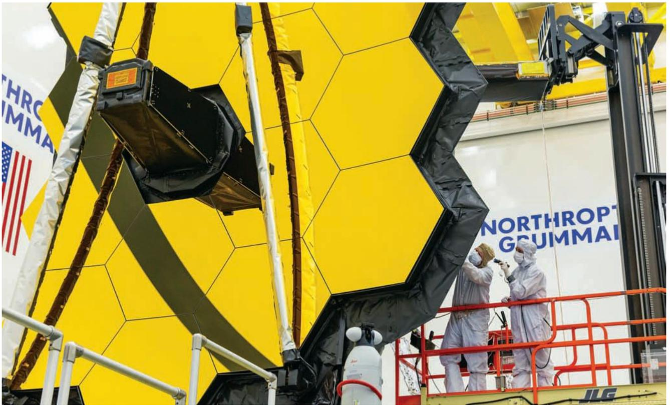
the sunshield must pack perfectly, folding onto itself rather like a parachute. All these parts and pieces must then unfold and interlock with precision for Webb to see objects at unprecedented distances and as they existed billions of years ago.
