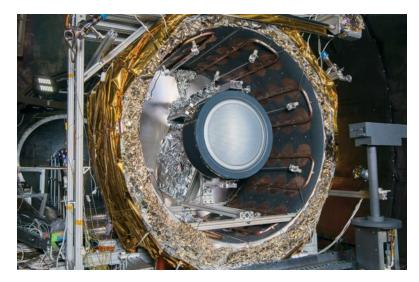
▲ NASA's Evolutionary Xenon Thruster-Commercial, NEXT-C, thruster completes thermal tests in a vacuum chamber at Glenn Research Center ahead of its November 2021 launch aboard the Double Asteroid Redirection Test spacecraft. The experimental gridded ion thruster propelled the spacecraft intermittently toward its impact with the asteroid Dimorphos in September.
