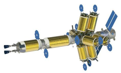
This rendering shows a Mars Transport Vehicle with two nuclear thermal propulsion engines on the left side and a habitat on the right side adjacent to eight liquid hydrogen drop tanks, although not all are visible. Aeroiet Rocketdyne
