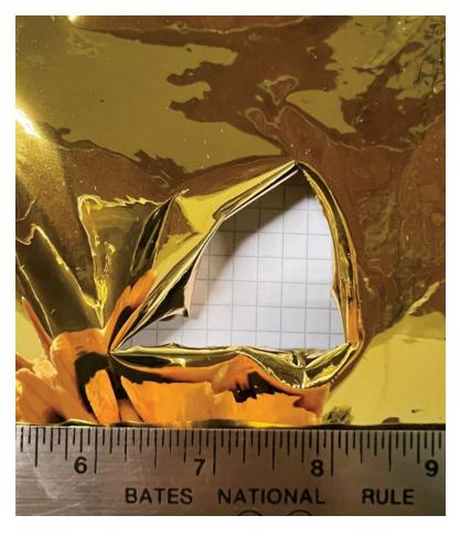
▲ U.S. Air Force Institute of Technology researchers fired an Air Force Research Laboratory cold gas gun at this gold membrane mirror sample to simulate impacts of space debris fragments.
