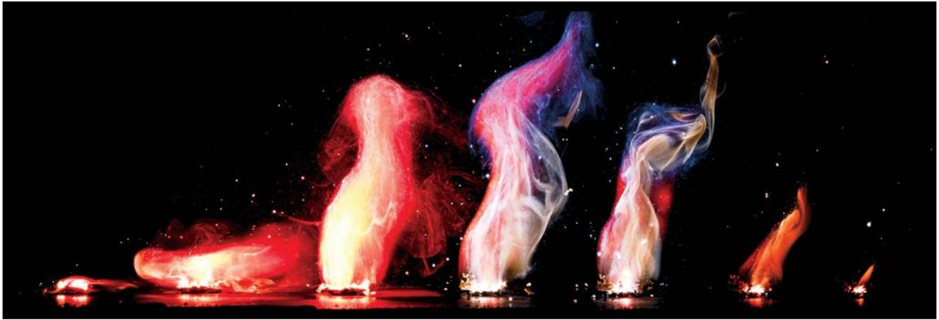
▲ Purdue University students tested a mix of 60% calcium perchlorate and 40% magnesium perchlorate to simulate how a solid propellant created from Martian soil might burn. As shown in this time-lapse image, their “Mars propellant” created red, white and blue flames.
