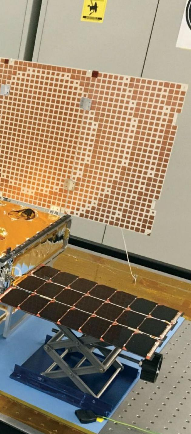
◀ NASA's Mars Cube One spacecraft are one example of how Mars could be explored via less expensive means. The pair of cubesats, pictured here in 2018 at NASA's Jet Propulsion Lab in California, relayed X-band signals from NASA's InSight lander, providing mission controllers real-time status updates about the InSight lander's November 2018 entry, descent and landing on Mars.
