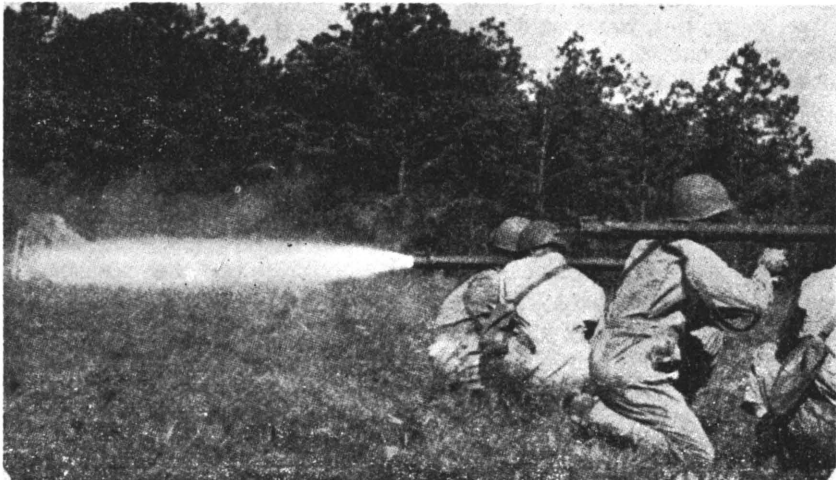
Driving Power —All burning of the projectile's rocket charge takes place within the launcher tube, thus preventing injury to the Bazookaman.
