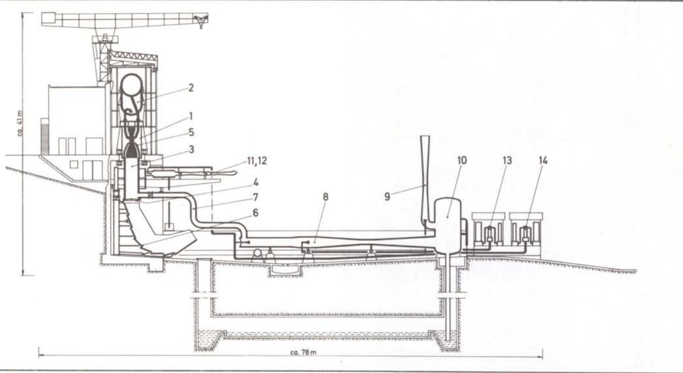
An 800 mm pipe (7) connects the diffuser to the steam ejector (8 and 9), which draws off the engine gases during the start-up phase. Part of the steam is condensed in an injection cooler (10) and the condensate falls into an underground sump.
