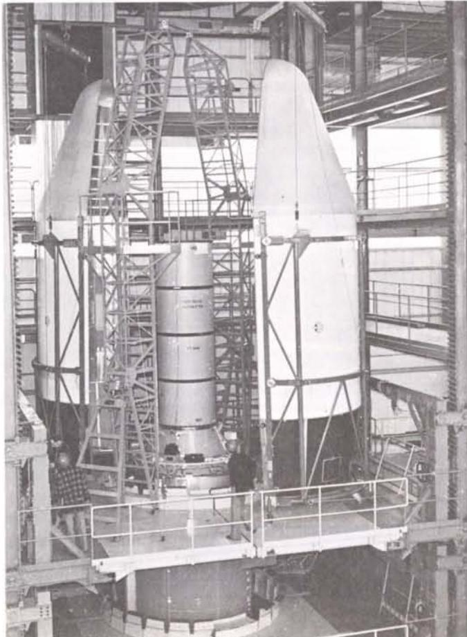
Figure 1 – Ariane fairing during integration for dynamic test.
