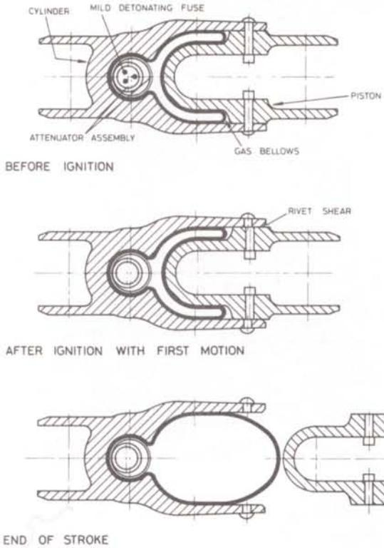
Figure 4 – Fairing vertical separation system (VSS).
