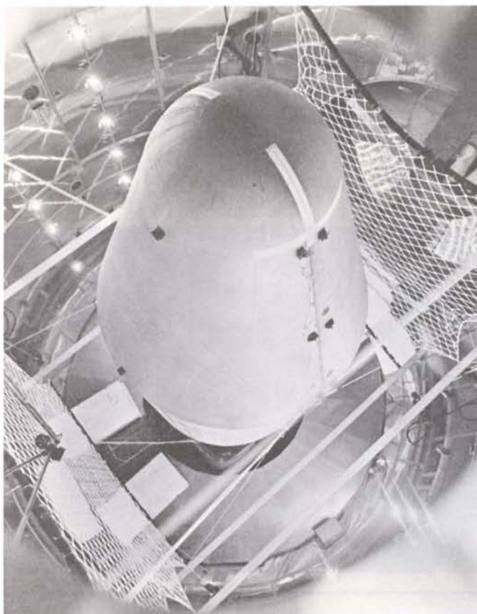
Figure 7 – First fairing separation test (SM1A) in the Dynamic Test Chamber (DTC) at ESTEC.
