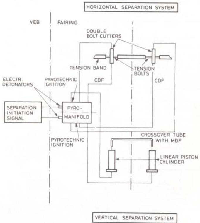
Figure 5 – Schematic of overall fairing separation system (VSS and HSS).
