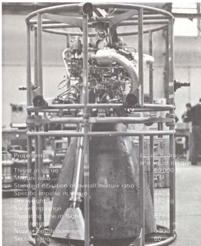
Figure 2 – An HM-7 engine assembled for test and, superimposed, its main operating characteristics.
