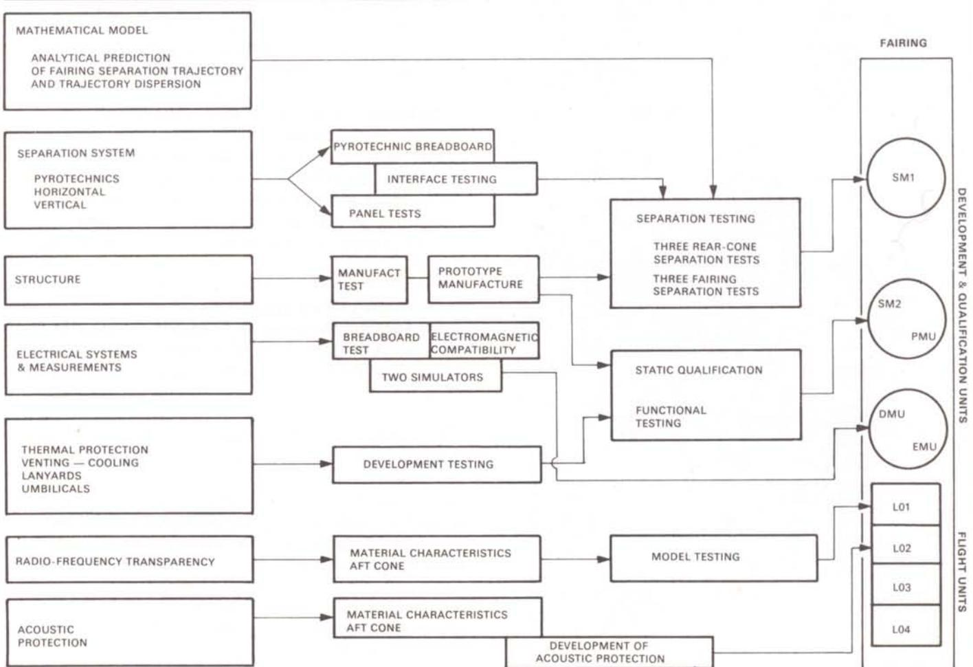
Figure 3 – Development logic for the Ariane fairing. (PMU = Propellant Mock-Up; DMU = Dynamic Mock-Up; EMU = Electrical Mock-Up).
