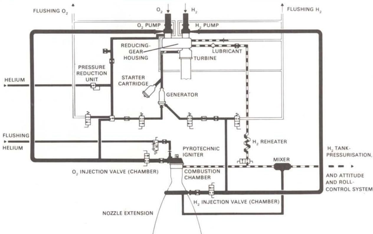
Figure 3 – Schematic of the operating cycle of the HM-7.
