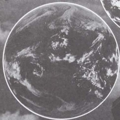
Pictures in the thermal infrared band show the differences in surface temperatures of clouds, seas and earth. The coldest areas appear white in these images (clouds at high altitudes) and warm gas are darkest (African Gulf, here). The seas, gray in the daytime image are therefore cooler than the land. Nighttime images show a reversal with sea darker or warmer than the continents.
