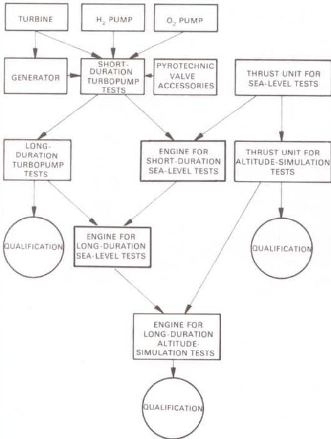
Figure 7 – Scheme for the main engine development tests.
