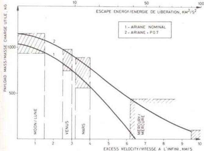
Figure 5 – Performance profiles for interplanetary missions
