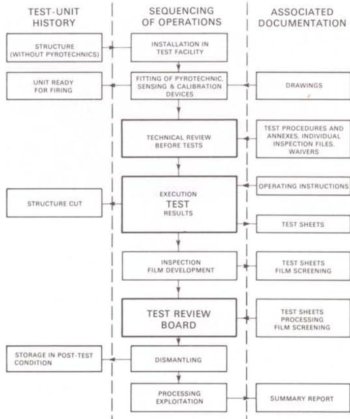
Figure 1 – Planning and documentation for stage-separation integration tests.
