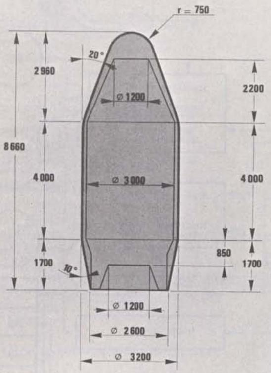
Figure 2 – Overall design and 'free volume' of the Ariane fairing.
