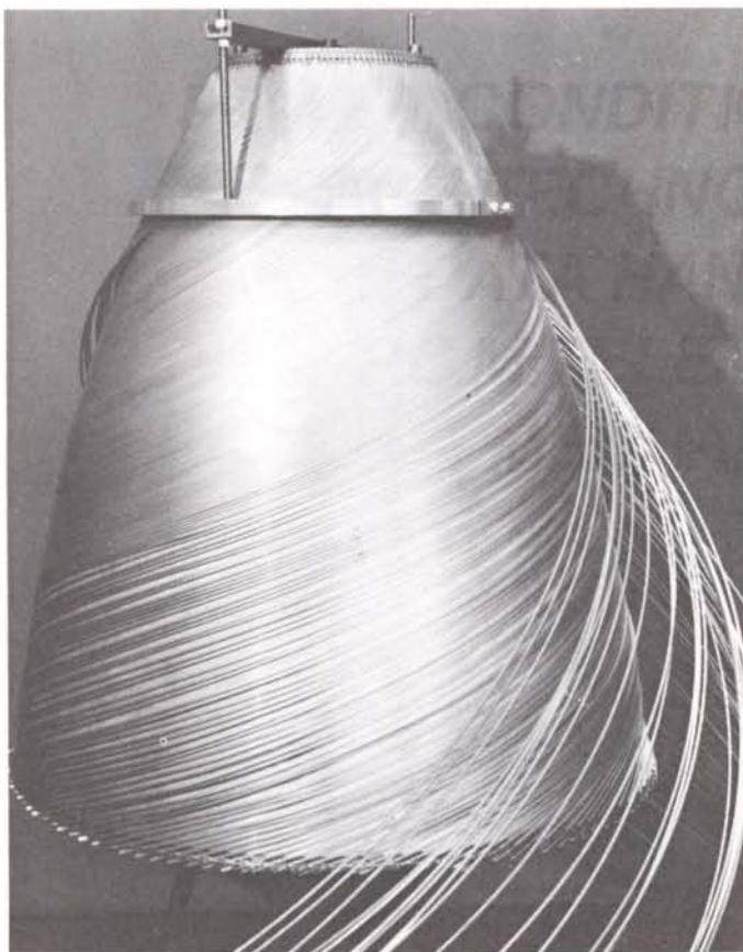
Figure 5 – Detachable nozzle extension used for testing under normal atmospheric conditions.
