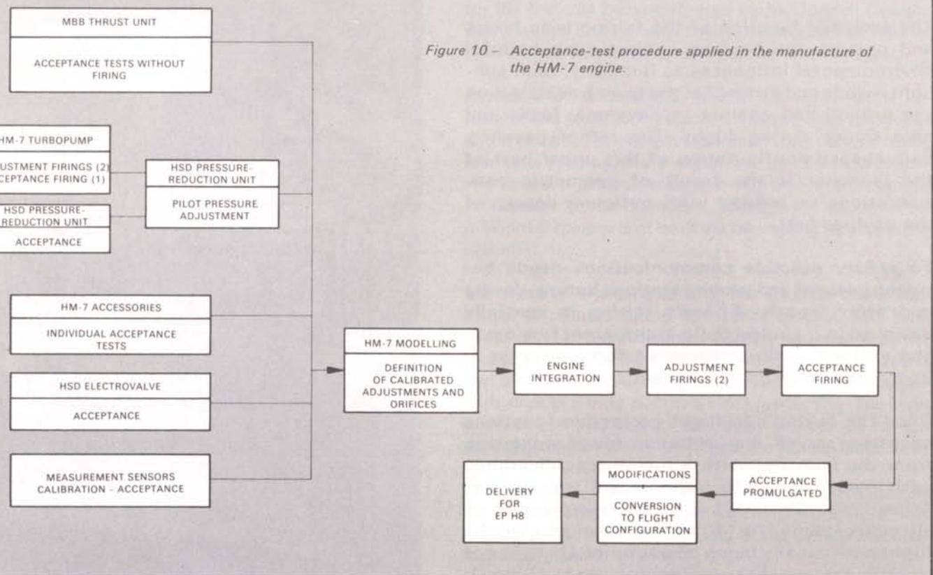
Figure 10 – Acceptance-test procedure applied in the manufacture of the HM-7 engine.
