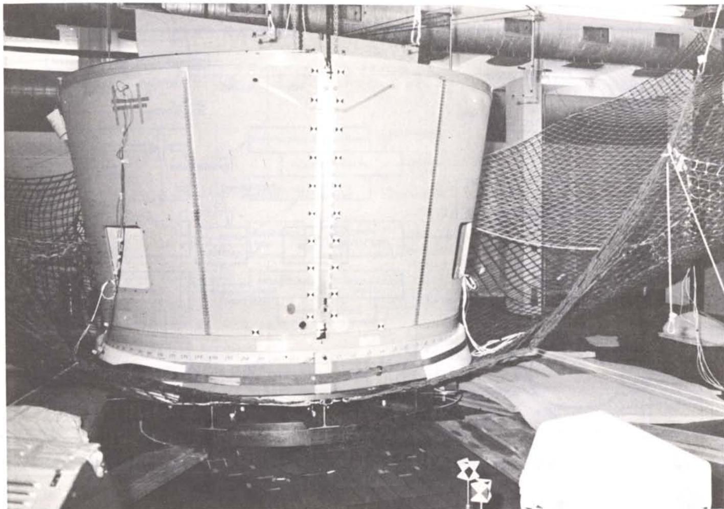
Figure 6 – Rear fairing cone installed on VEB, ready for separation test.
