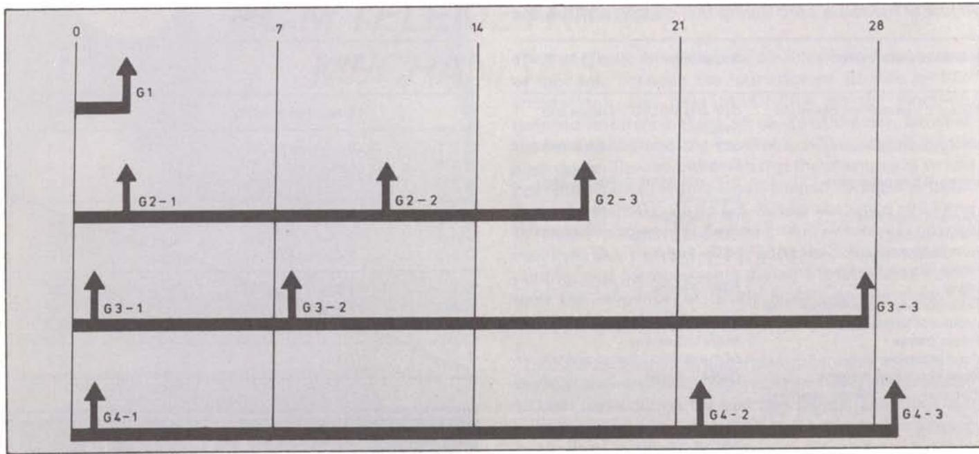
Figure 3 – Timing of 'cluster' or 'G' tests after  $N_2O_4$  loading (scale in days).
