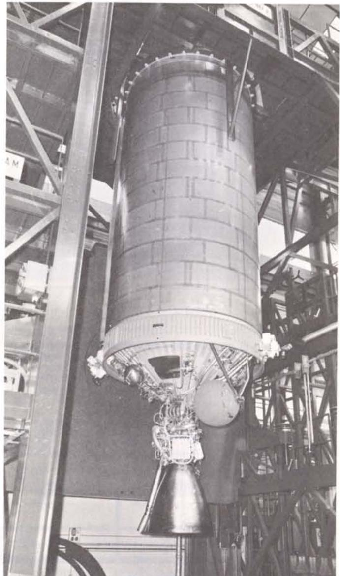
Figure 1 – The HM-7 engine mounted on the third-stage thrust frame.
