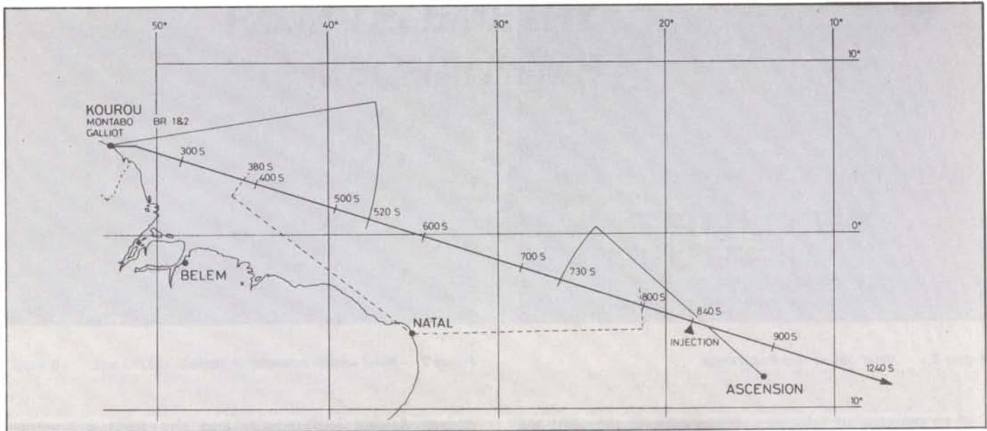
Figure 8 — Locations of ground tracking stations, with indications of radar visibility.
