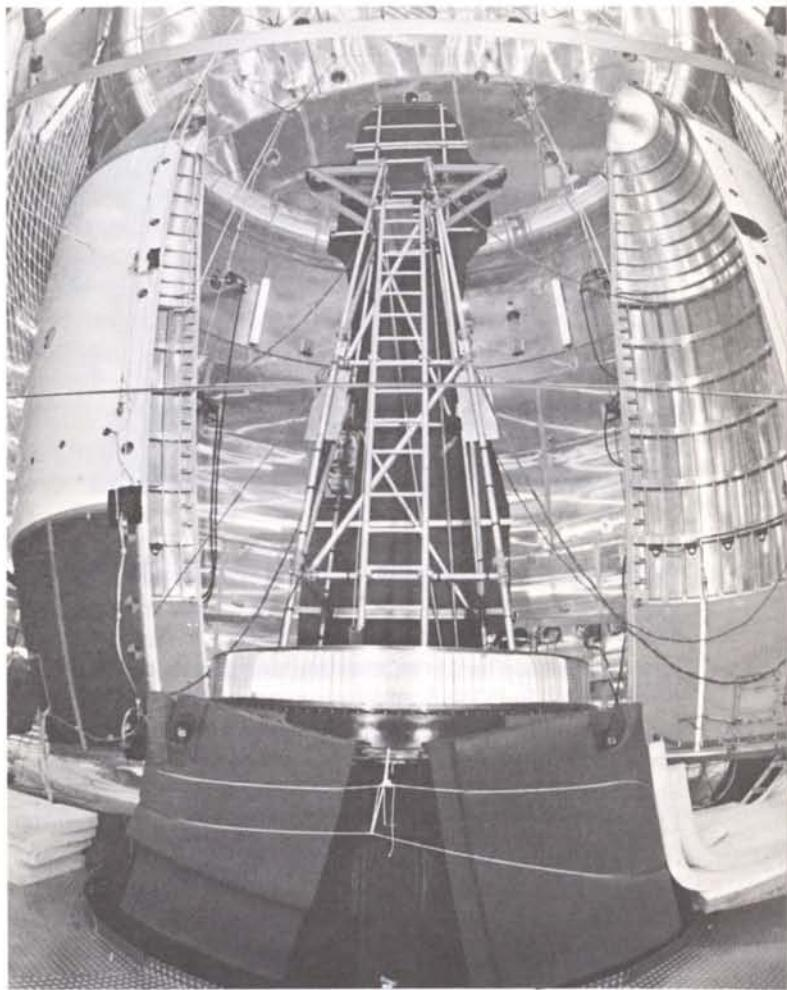
There followed two more successful qualification tests using the European-developed VSS, the first on 20 October 1977, the second on 7 April 1978. The second of these tests had the supplementary objective of proving that one-sided initiation of the VSS would still result in trouble-free separation.
