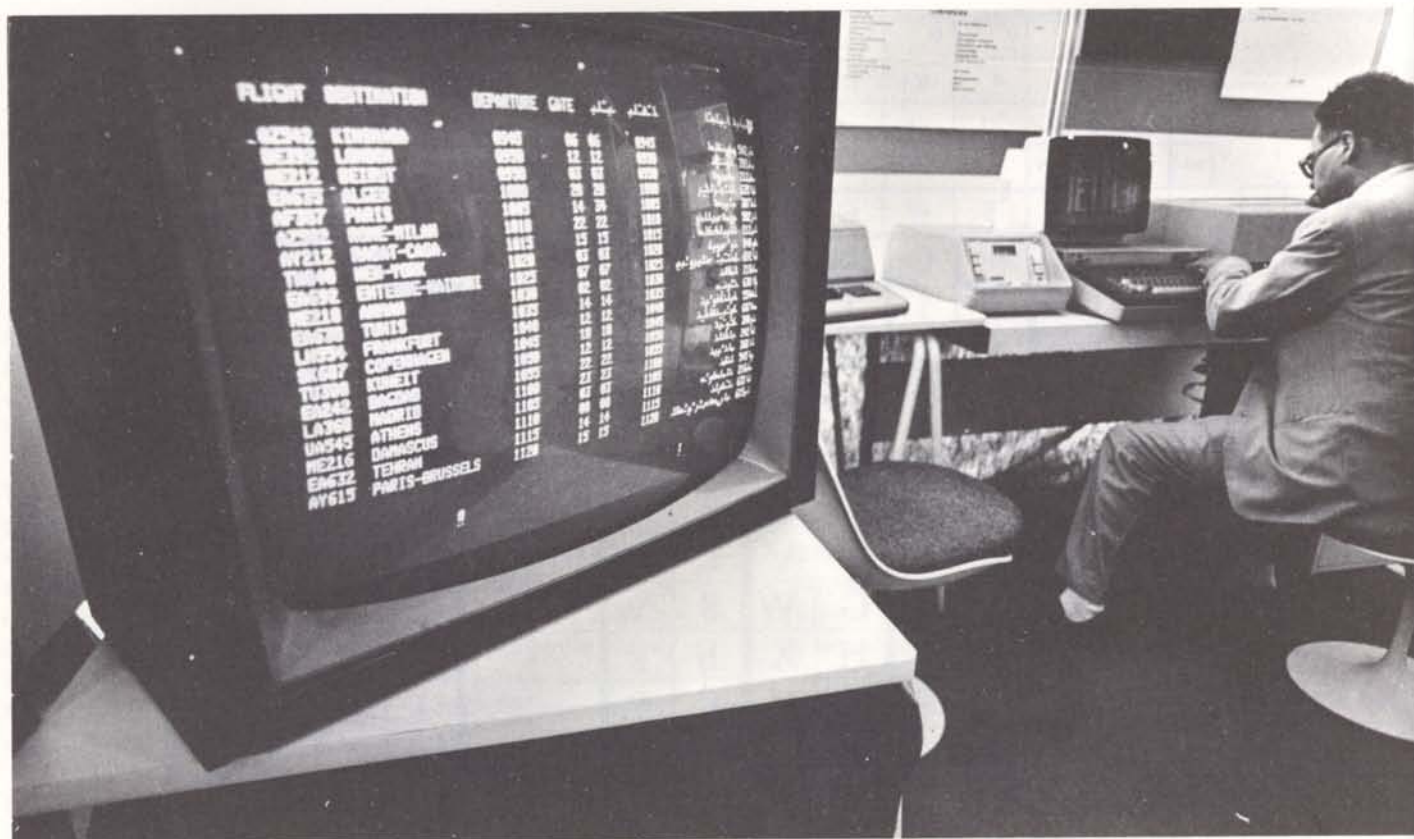
Figure 4 – Screen display of airport flight information in both Latin and Arabic characters.
