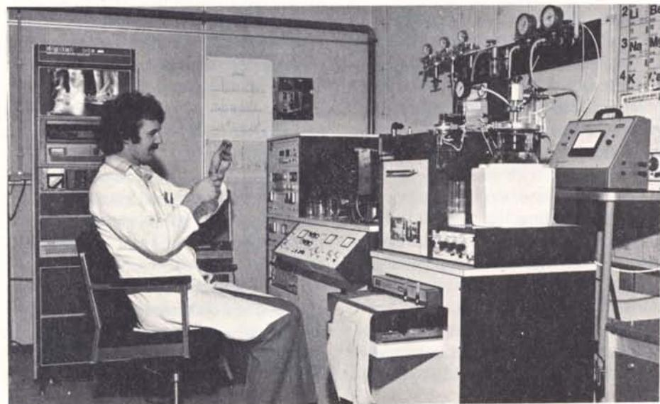
Figure 4 – Chamber for unit-level testing containing a commercial motor under test for the First Spacelab Payload. This chamber, which can be both heated and evacuated, has a volume of approximately 150 l.
