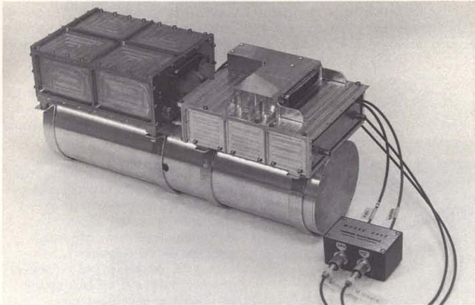
Figure 8a – Development model of Hipparcos' Main Detector Assembly (MDA). The Image Dissector Tube (IDT) focussing and deflection coils and preamplifiers are located in the cylindrical housing. The Pulse Amplifier and Discriminator (PAD) is located in the housing at the rear, the high-voltage power supply (CRI) in that at the front (courtesy of Netherlands Space Research Laboratory)
