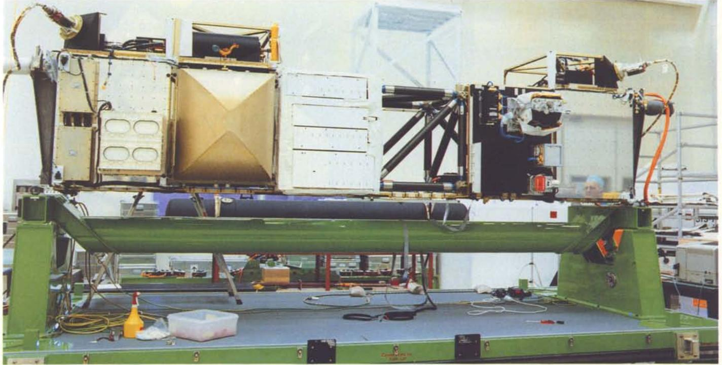
Figure 2 — The Solar-Cell Calibration Experiment in place on SPAS-01
