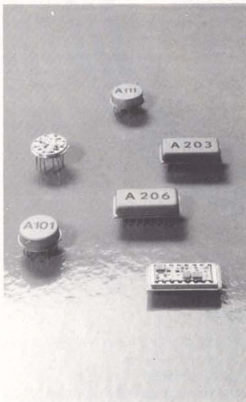
Models A-101 and A-111 are Charge Sensitive Preamplifier-Discriminators developed especially for instrumentation employing photomultiplier tubes, channel electron multipliers (CEM), microchannel plates (MCP), channel electron multiplier arrays (CEMA) and other charge producing detectors in the pulse counting mode.
