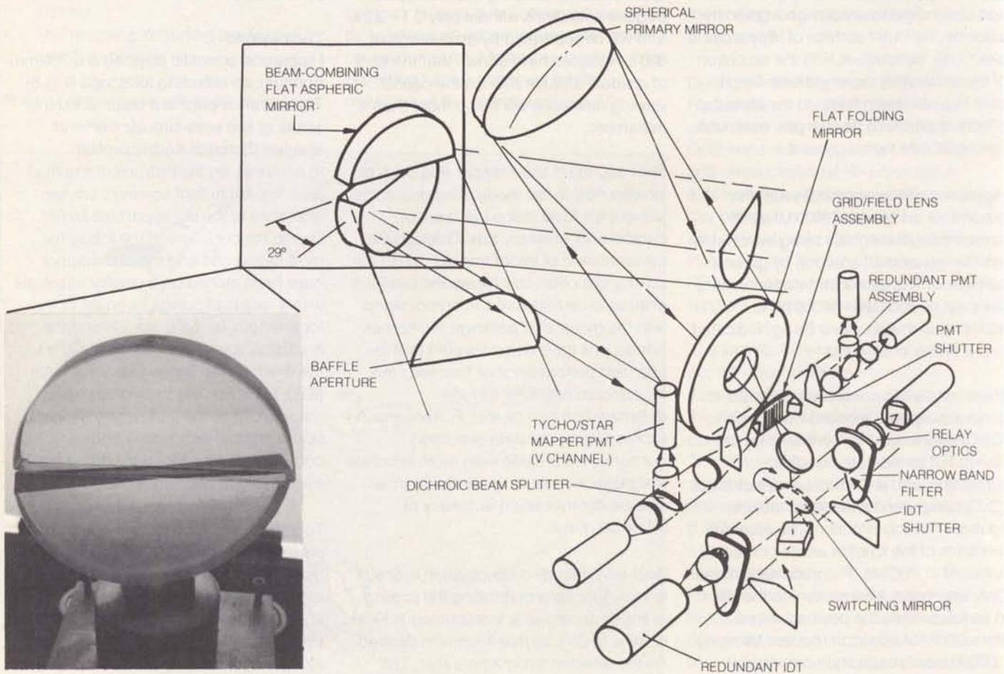
Figure 7 — Alignment testing of the Hipparcos beam combiner, at Matra (Toulouse), as part of the Optical Support Programme
