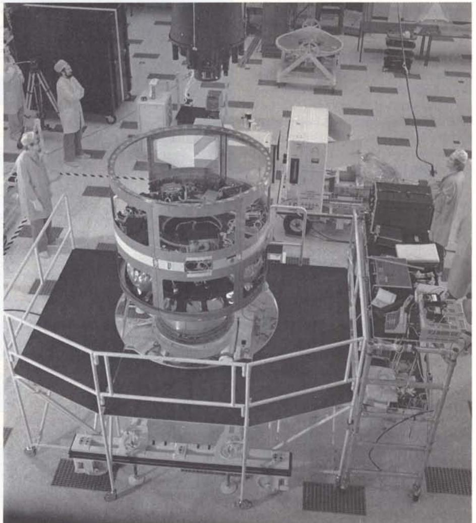
Figure 5 – Cos-B under test in the Heat-Balance Facility at ESTEC
