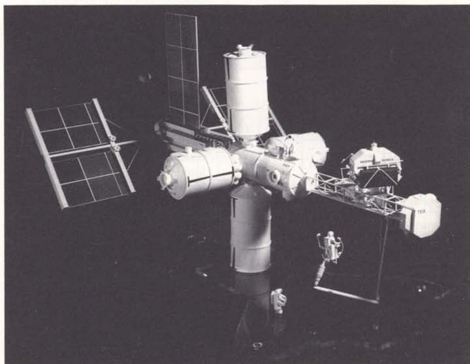
Figure 12 – Columbus elements: Manned service vehicle docked to free-flying pressurised laboratory
