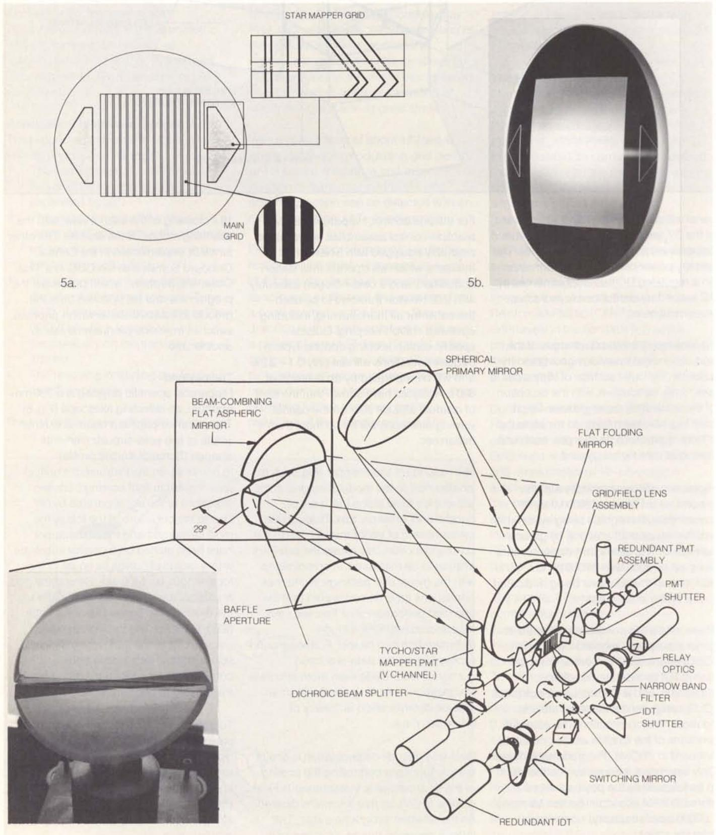
Figure 7 — Alignment testing of the Hipparcos beam combiner, at Matra (Toulouse), as part of the Optical Support Programme
