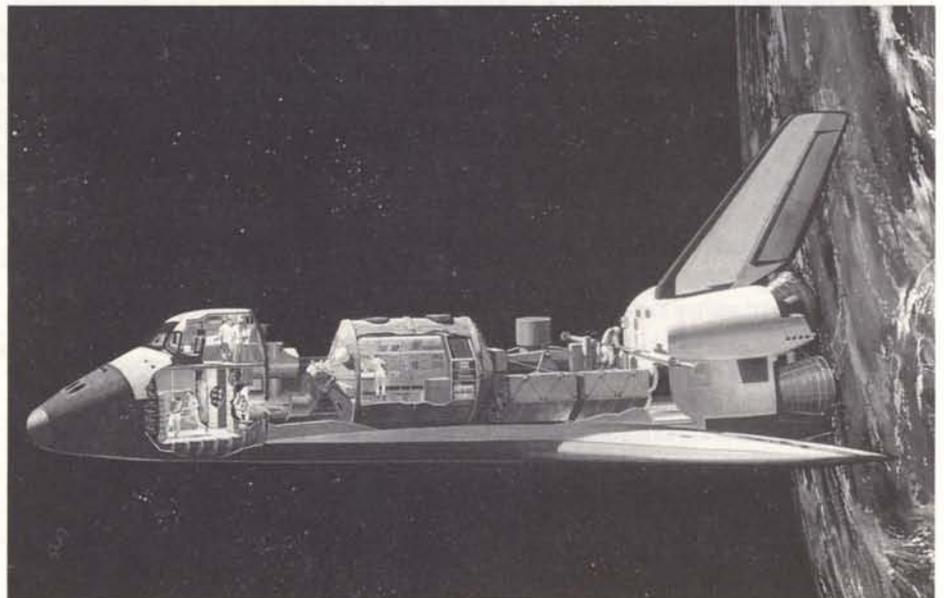
*Figure 1 – Spacelab in the Shuttle's payload bay (Spacelab-1 configuration)*
