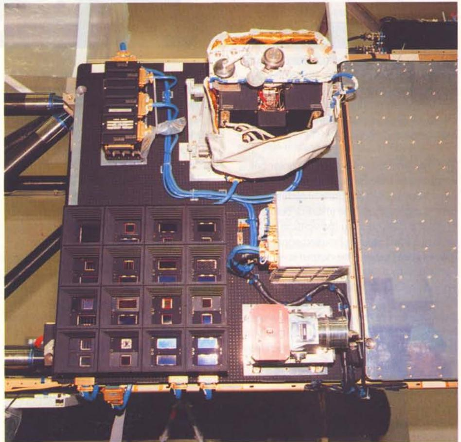
Figure 3 – The SCCE mounted on the experiment support plate on the SPAS, with the baffle subassembly in place
