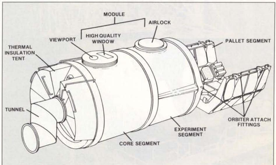
Figure 4 – Typical Spacelab flight configurations
