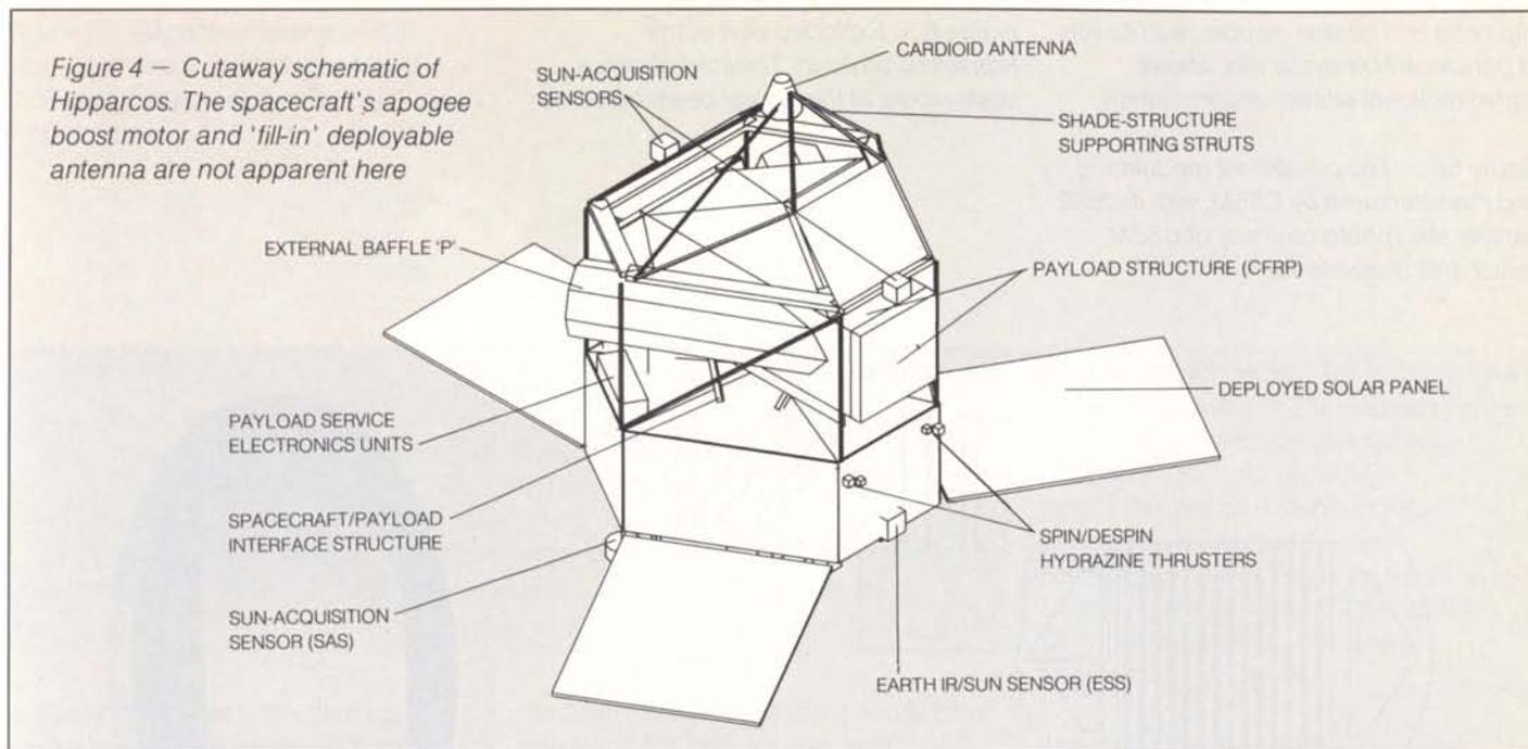
panel will deliver about 120 W at the end of the 2½ year mission. Nickel-cadmium batteries will provide power in eclipse. The primary power-distribution system relies on a regulated DC bus, supplemented by AC secondary distribution to individual equipment items.
