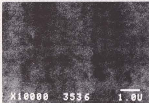
MYLAR film, Al Metallized, BEFORE being exposed to the flux of ATOX
