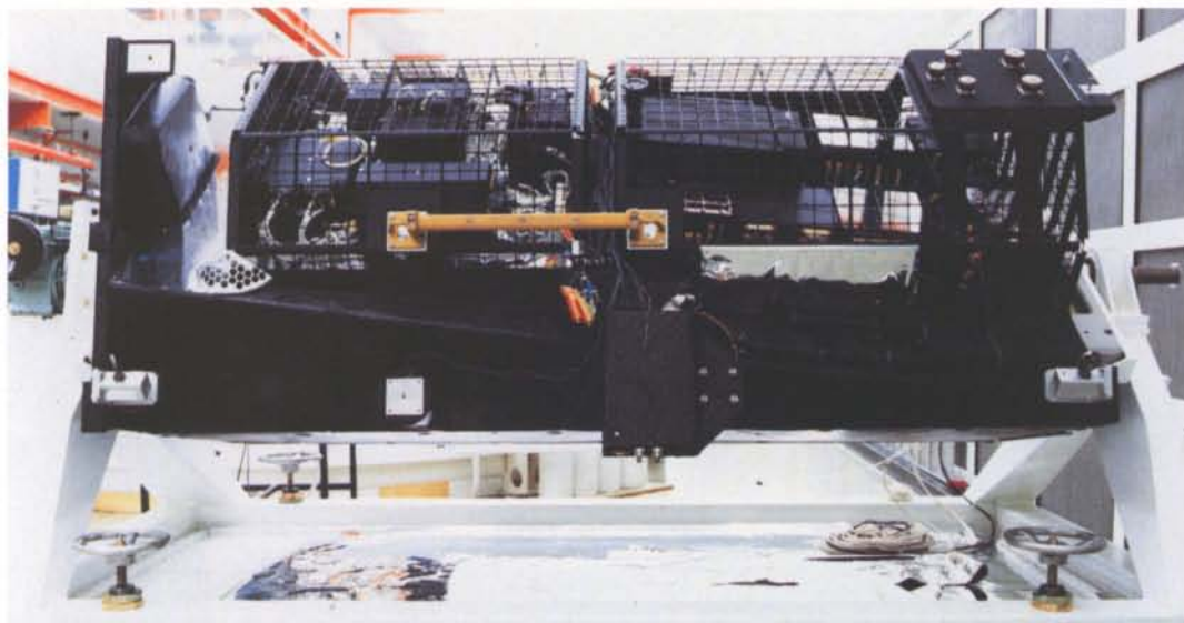
Figure 3. The assembled Faint Object Camera (FOC). The yellow handles are to assist the astronauts in handling the instrument in orbit
