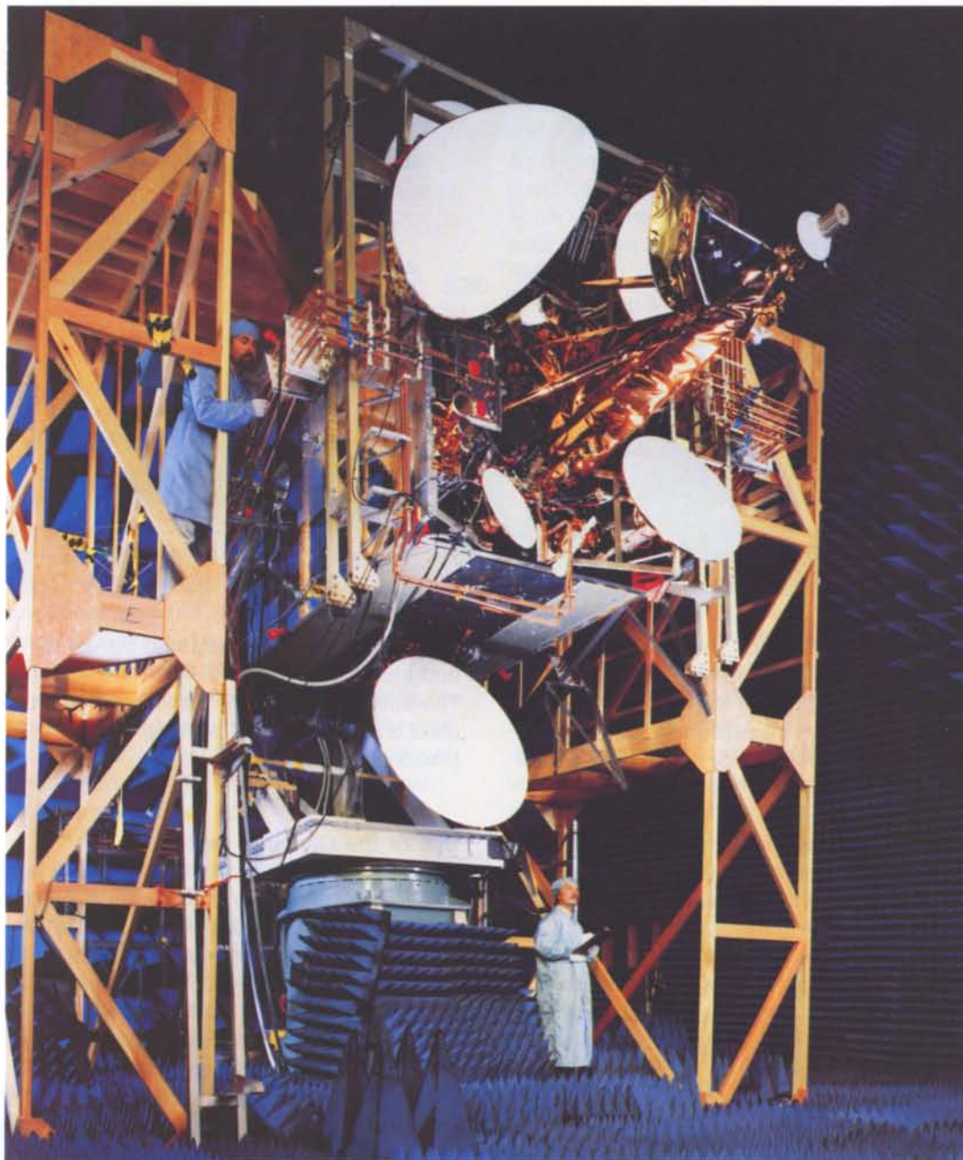
Figure 6. The Olympus satellite undergoing testing in the anechoic chamber at David Florida Laboratories in Ottawa, Canada
