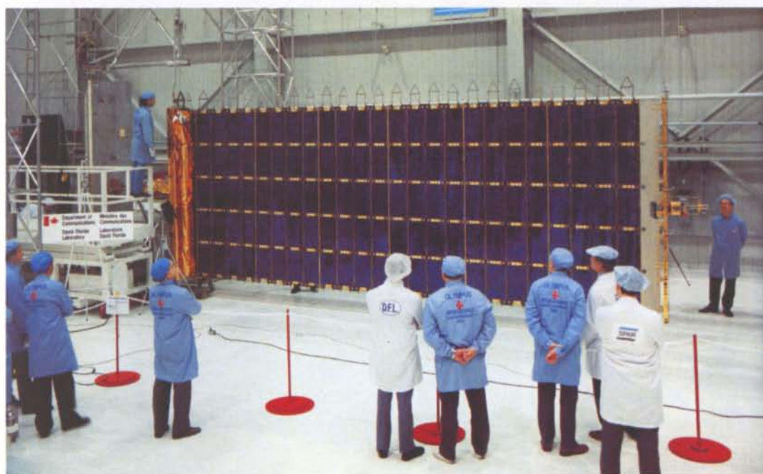
Figure 2. One wing of the Olympus solar array during deployment testing at the David Florida Laboratories in Ottawa, Canada. The array is supported by complex ground equipment that simulates the zero-g deployment environment in space (photo courtesy of CRC, Ottawa)
