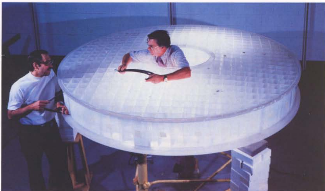
Figure 5. The 2.4-m diameter primary mirror blank of the HST. Its reflecting surface is figured to an accuracy of better than five millionths of a centimetre (courtesy of Perkin-Elmer)
