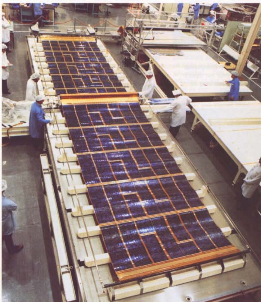
Figure 4. One of the ESA-supplied HST solar arrays undergoing testing. HST has two such arrays, which together provide 4.5 kW of power to the spacecraft
