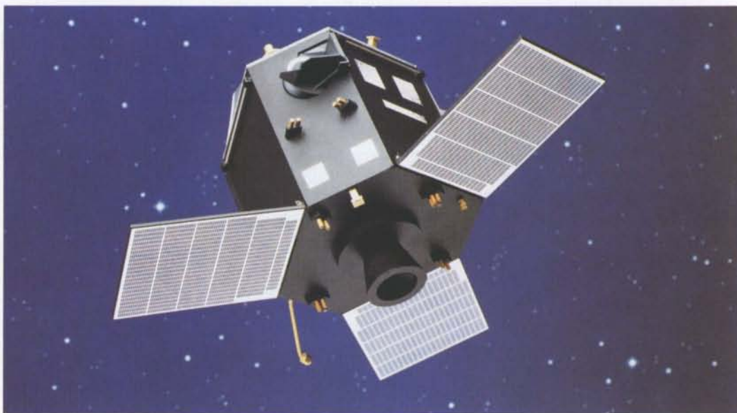
Figure 2. Artist's impression of the Hipparcos satellite. The solar panels, pointing towards the Sun, the apogee boost motor, the antennas linking the satellite to the control centre on Earth, and the entrance apertures of the telescope are all visible
