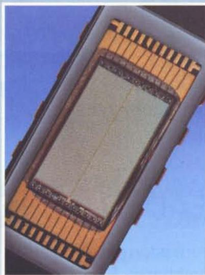
Silicon on Sapphire process. The Silicon on Sapphire eliminates the risk of latch-up and is the only commercially available technology that offers uncompromising performance in all aspects of hostile radiation environments.
