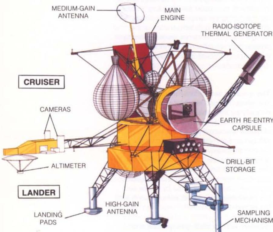
**Figure 2. The Rosetta/CNSR space segment: carrier, lander and aerocapsule**
