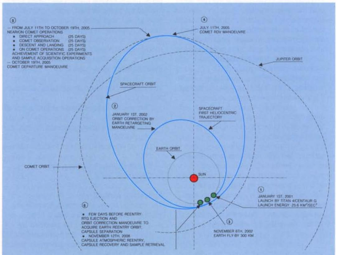
**Figure 3. Baseline Rosetta/CNSR trajectory to Comet Churiumov-Gerasimenko**
