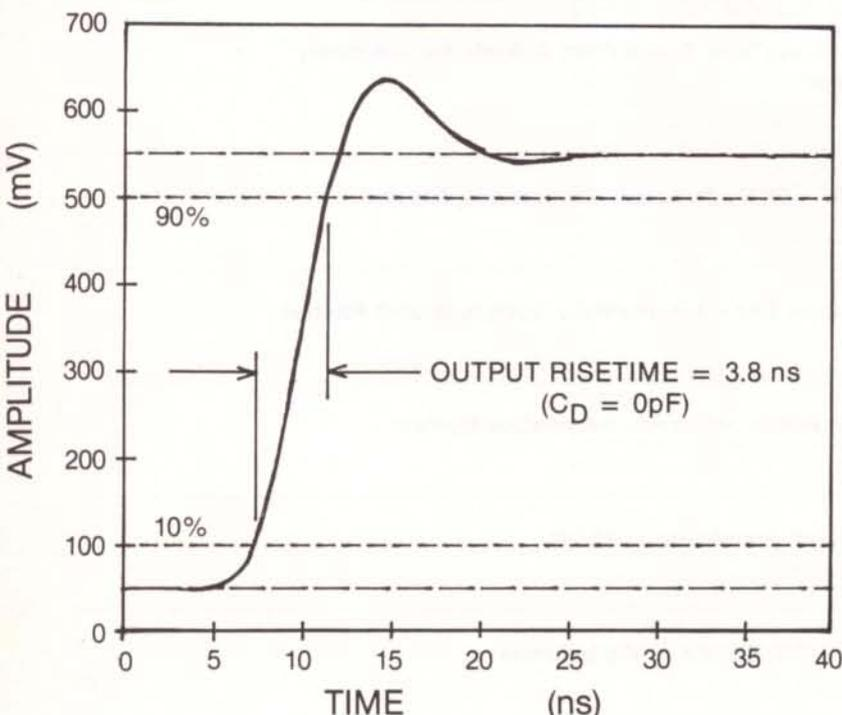
**A NEW STATE-OF-THE-ART**
