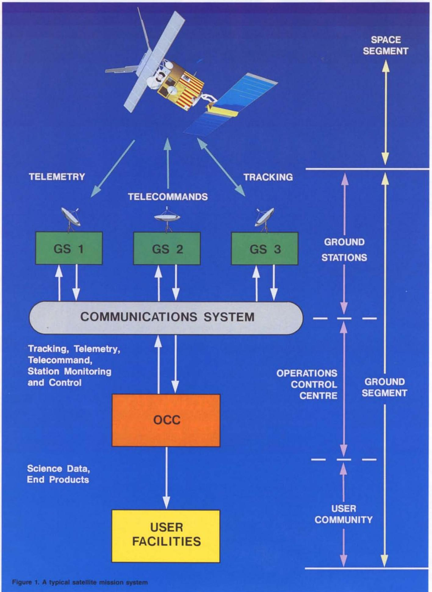
Figure 1. A typical satellite mission system
