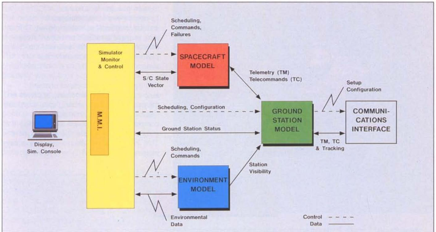
The ground-station model, the communications interface and the simulator monitoring and control function are, to a very large extent, spacecraft-independent and therefore common to all simulators. It was therefore possible to group them into a standard package, which provides a general framework to all simulator designers and ensures that a certain level of commonality is maintained in the end-user interface throughout the various simulator implementations.
