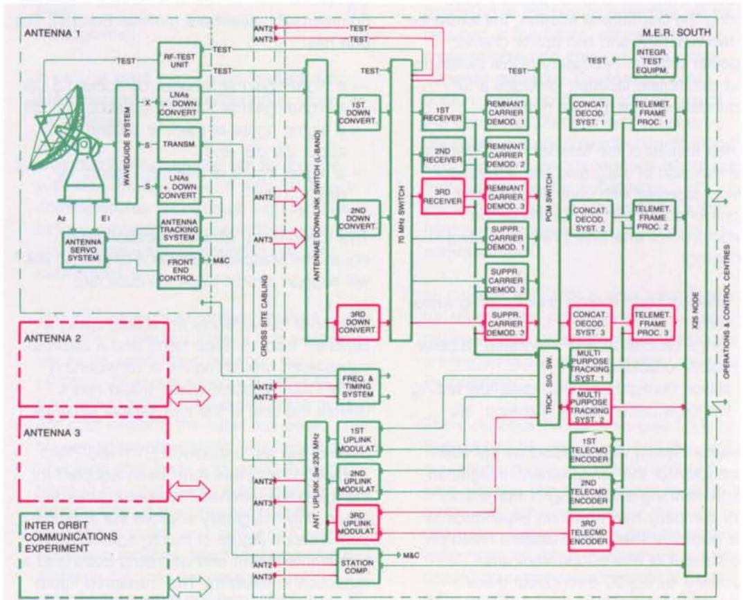
remnant carrier demodulator has been developed by Bell (Belgium) to function with the extremely poor signal-to-noise ratios found with encoded data. It is an improved version of the 'High-Performance Demodulator' used during the Giotto project.
