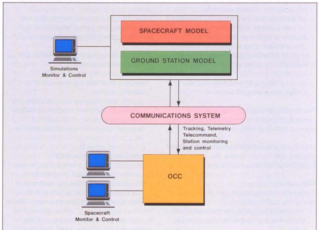
Figure 4. A typical simulation configuration at ESOC
