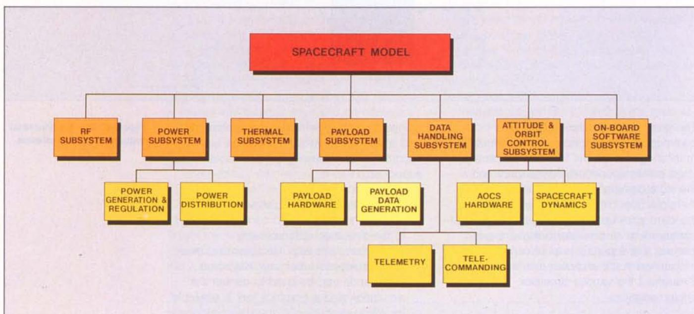
**Figure 6. A typical spacecraft-model breakdown**
