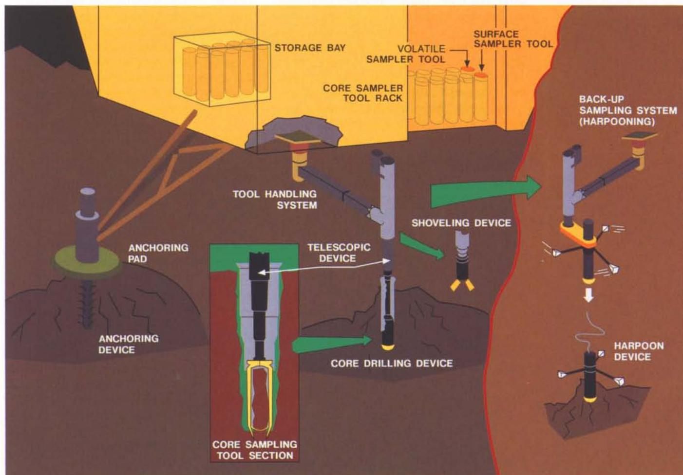
be automatically adjusted to fit the soil characteristics and a sample cutter mechanism, mounted at the end of each sampling tube, will be activated when the drill tool has reached maximum depth. A period of ten days has been planned for the sampling operations.
