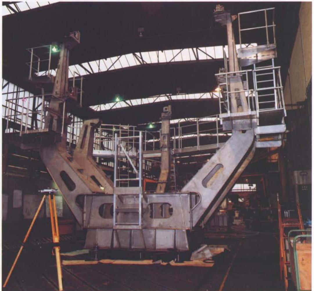
Figure 7. The large test adaptor constructed to support the IRIS structural/thermal model in the LSS at ESTEC
