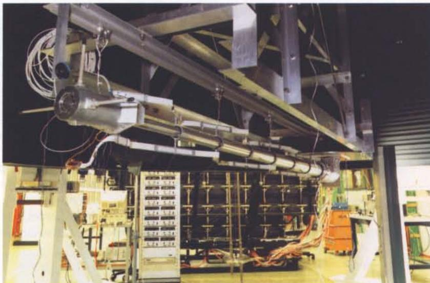
**Figure 11. The Deployable/Retrievable Boom System (DRBS) for the Tethered Satellite (TSS-S)**
