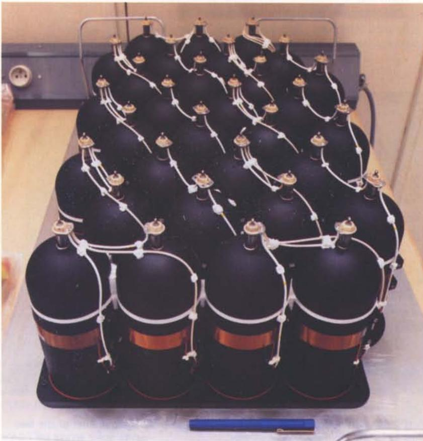
**Figure 5. Nickel-cadmium batteries for the Olympus spacecraft**
