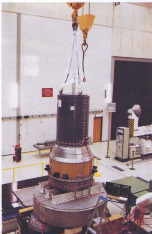
**Figure 4. Vibration testing of the IRIS propulsion stage (ISS) and payload at ESTEC**
