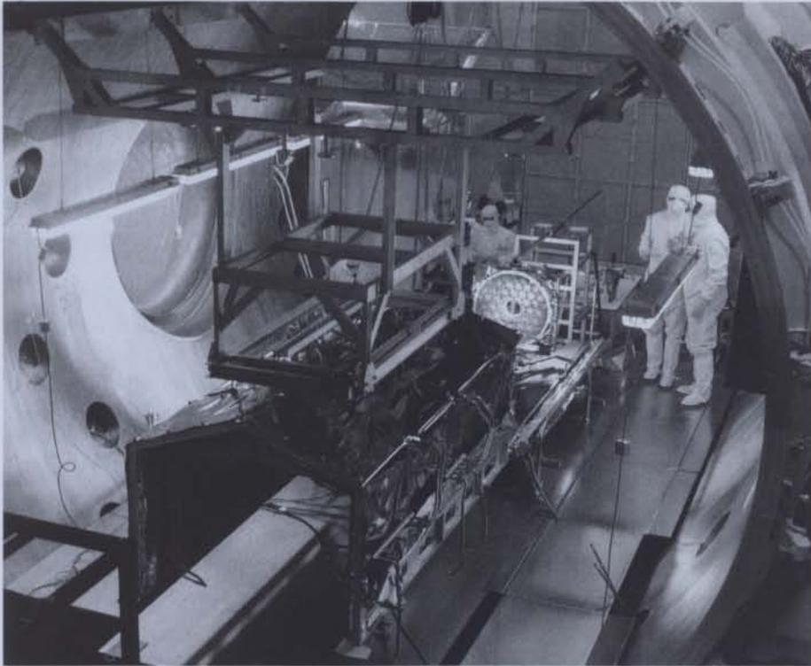
*Test set-up at Institut d'Astrophysique de Liège (B) for the ISO satellite's primary mirror*
