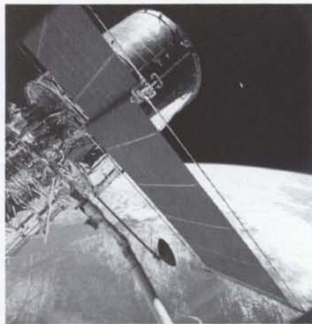
Cover: Hubble Space Telescope suspended in space from Space Shuttle Discovery's remote manipulator system, with one of the two ESA-provided roll-out solar arrays deployed in the foreground (see page 94)
