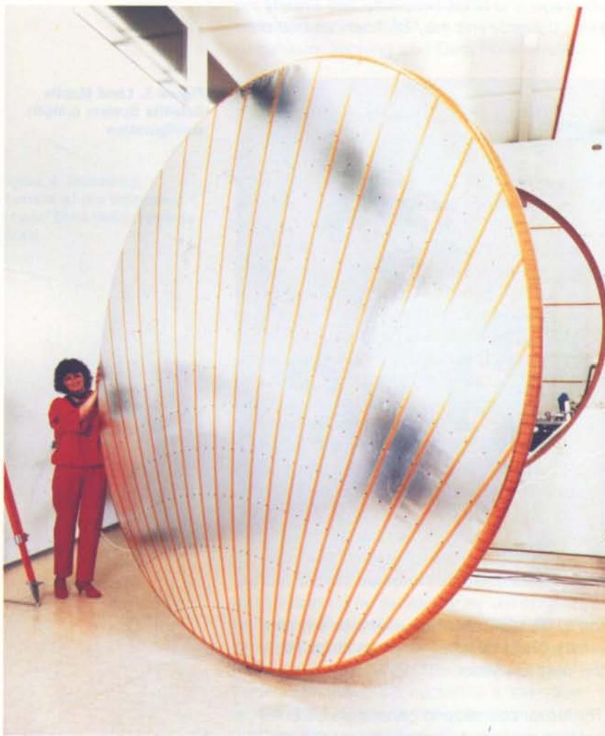
**Figure 6. A space-rigidised inflatable satellite reflector (courtesy of Contraves)**
