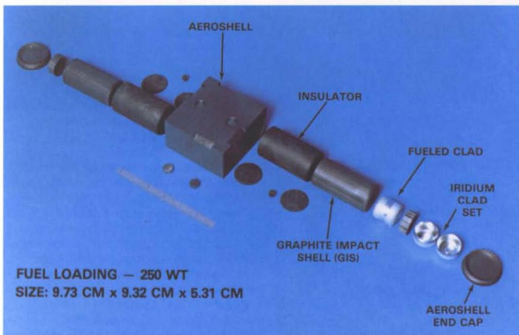
Figure 2. The General-Purpose Heat Source (GPHS)
