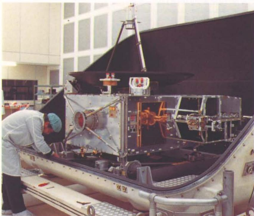
**Figure 4. The Ulysses spacecraft structure photographed at ESTEC in 1983, without its thermal cladding**
