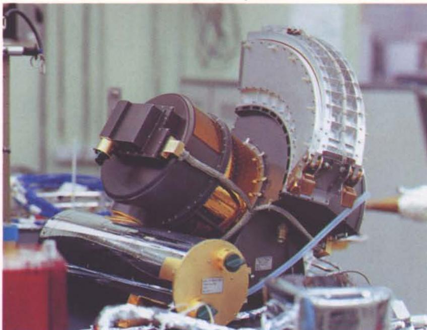
**Figure 5. The Solar-Wind Ion-Composition Spectrometer (GLG-2)**
