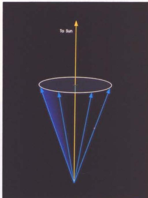
Figure 7. Possible spin-axis pointing directions knowing the solar aspect angle
