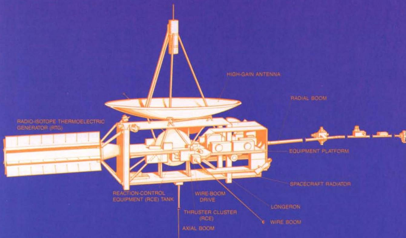
Figure 1. Flight configuration of the Ulysses spacecraft
