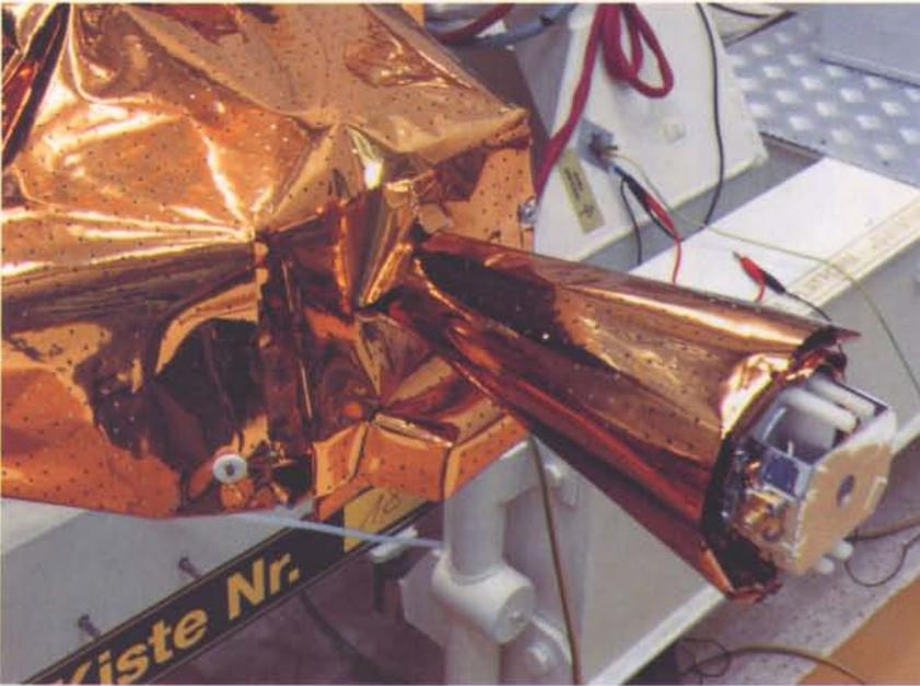
**Figure 7. One of the tip masses (bottom right) used to deploy the wire-boom antennas by centrifugal force**
