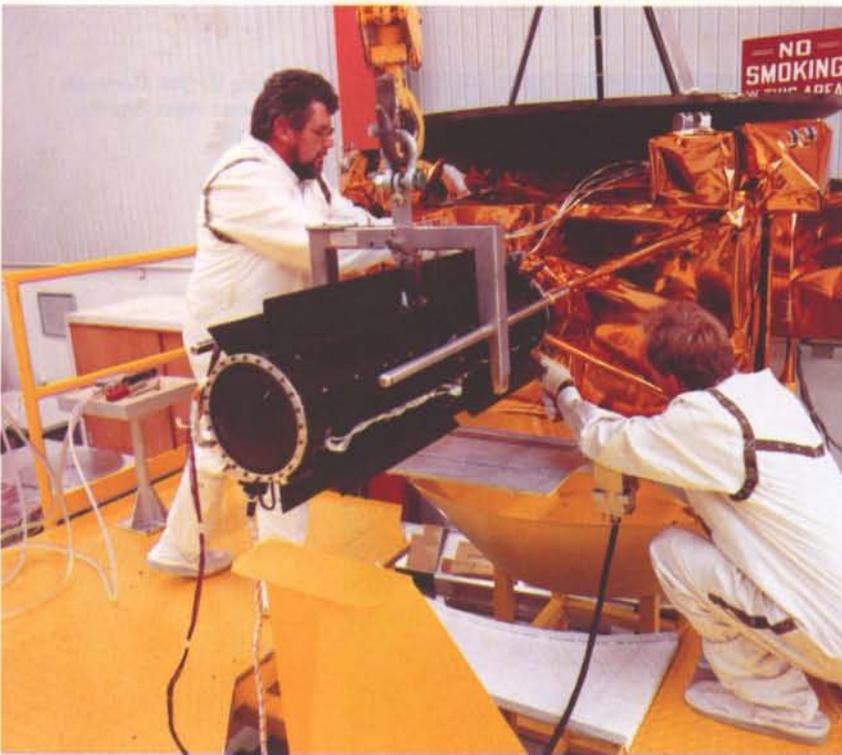
**Figure 3. RTG fit-checking in progress at ESTEC, Noordwijk (NL)**
