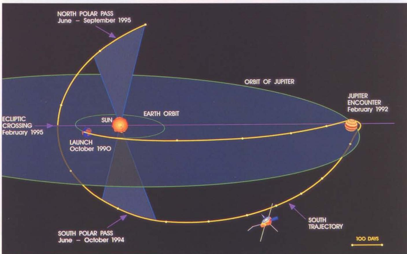
**Figure 7.** Ulysses' trajectory viewed from 15° above the ecliptic plane. The blue segments show regions in which the heliographic latitude of the spacecraft exceeds 70°. The dots plotted along Ulysses' trajectory are at 100 d intervals.
