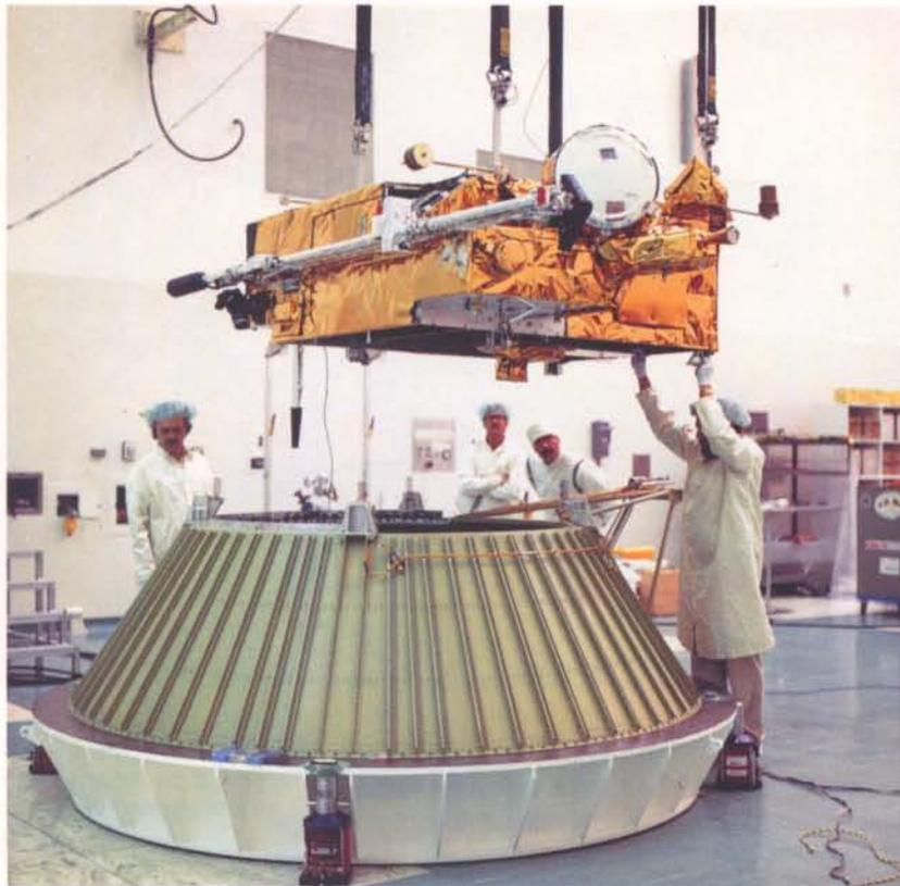
**Figure 3. Ulysses spacecraft/launcher-adapter fit-check in progress at KSC in February 1986**
