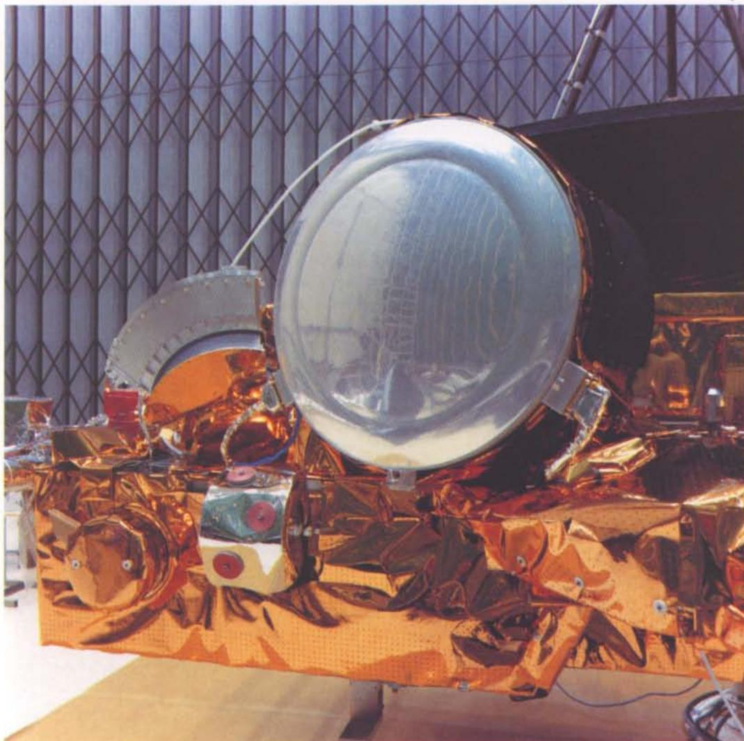
Figure 11. A view of the -X wing of the Ulysses spacecraft, dominated by the large circular cover of the Cosmic Dust Experiment (GRU). Also visible are the KEP and GLG packages enclosed in their thermal blankets
