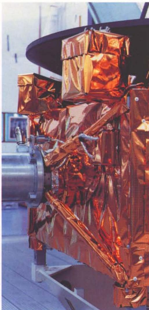
Figure 5. Mounting of the Radio-isotope Thermoelectric Generator (RTG)
