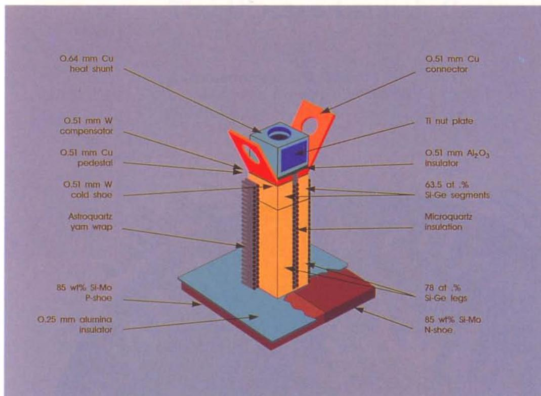
Figure 4. The Thermo-electric Unicouple
