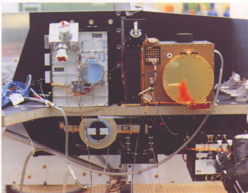
**Figure 9. The Cosmic-Ray and Solar-Particle Experiment (SIM) mounted on the spacecraft platform. In this view, three of the five instrument packages are visible: SIM-1 (above left), SIM-2 (above right) and SIM-3B (below left)**
