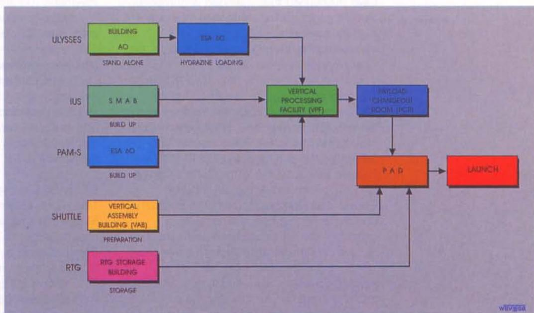
Figure 1. Launch processing flow
