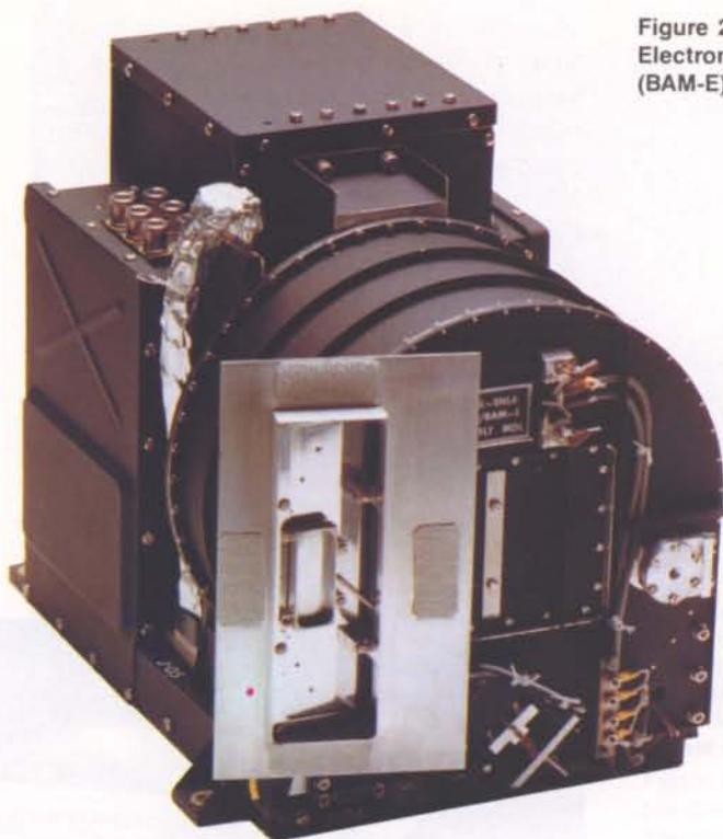
Figure 2. The Solar-Wind Electron Experiment (BAM-E) package
