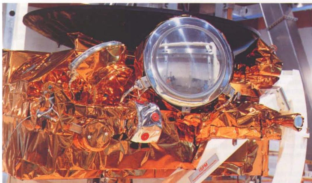
**Figure 8. Ulysses' gold-coloured high-efficiency thermal blanket**
