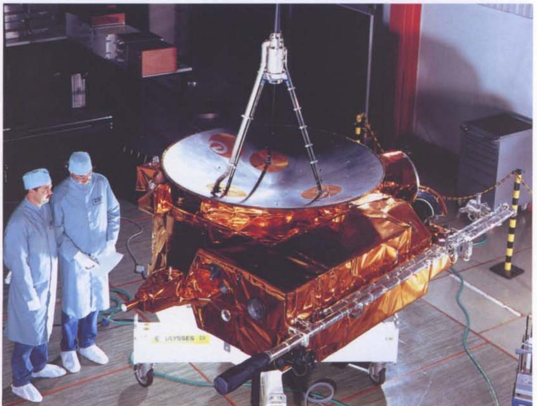
Figure 3. Ulysses flight-model spacecraft, with the radial boom folded in launch configuration
