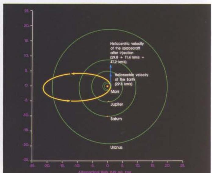
11.4 km/s, the maximum ecliptic inclination that can be reached is  $23^\circ$ , the effective initial heliocentric velocity when the launcher is standing on the launch pad being 29.8 km/s in the ecliptic plane (Fig. 3).
