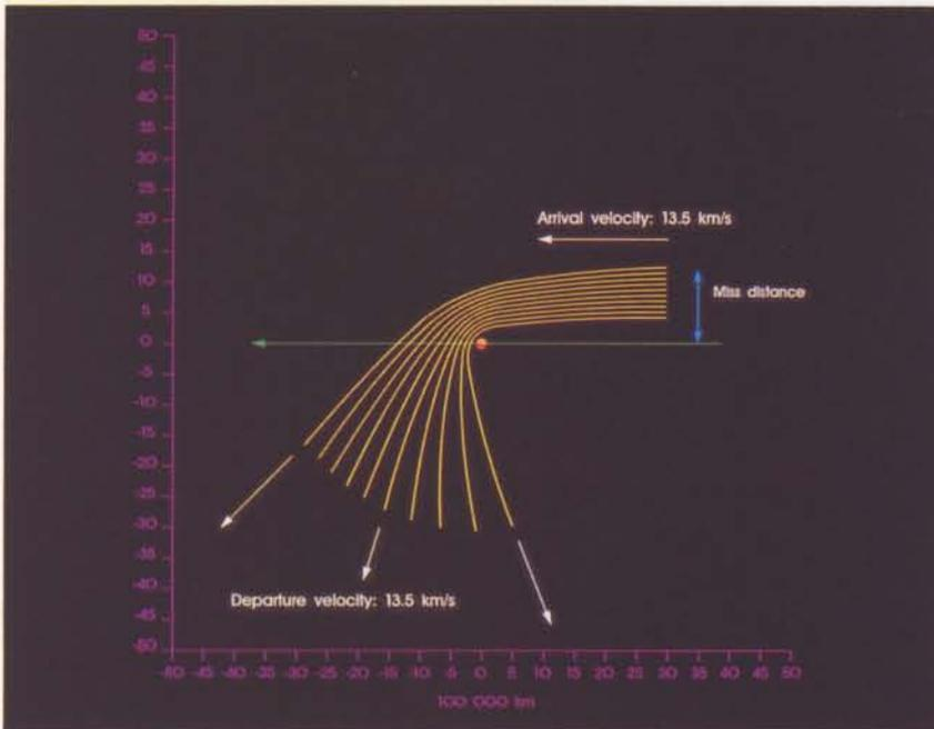
**Figure 5.** Possible deflections at Jupiter for a spacecraft arriving with a velocity of 13.5 km/s. The most deflected orbit has a miss-distance of 500 000 km and a pericentre radius of 2.26 Jupiter radii. The least deflected orbit has a miss-distance of 1 400 000 km and a pericentre radius of 12.2 Jupiter radii (1 Jupiter radius = 71 398 km).
