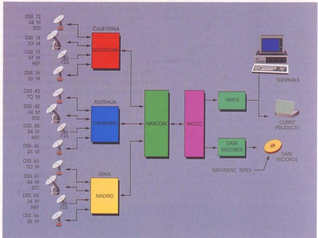
one path flowing to the ESA data-processing computer (UMCS) where it will be processed in real-time, and the other to the Data Records System, where the incoming data will be processed in non-real-time.
