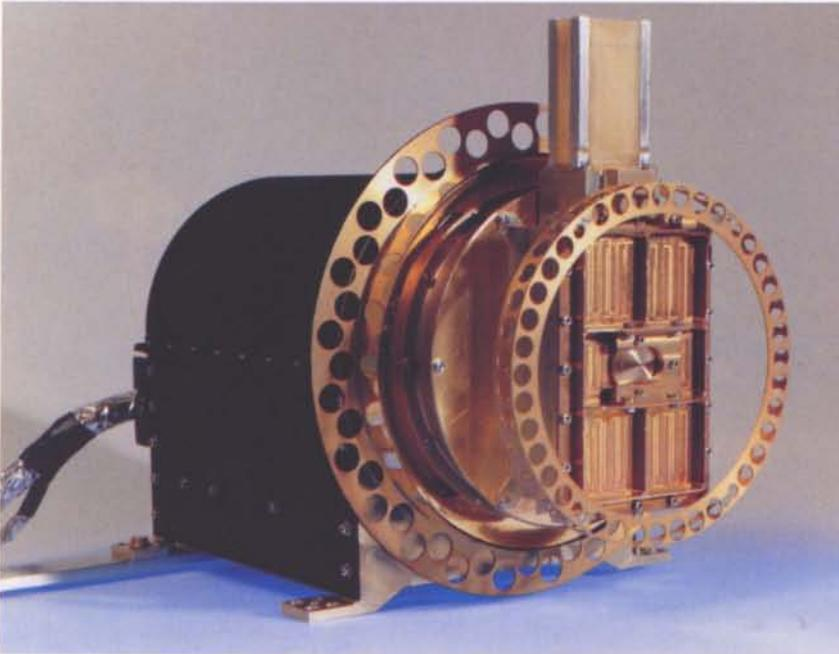
**Figure 7. The Interstellar Neutral Gas Experiment (KEP-3) mounted on its rotating platform. The circular frames are thermal-blanket supports**
