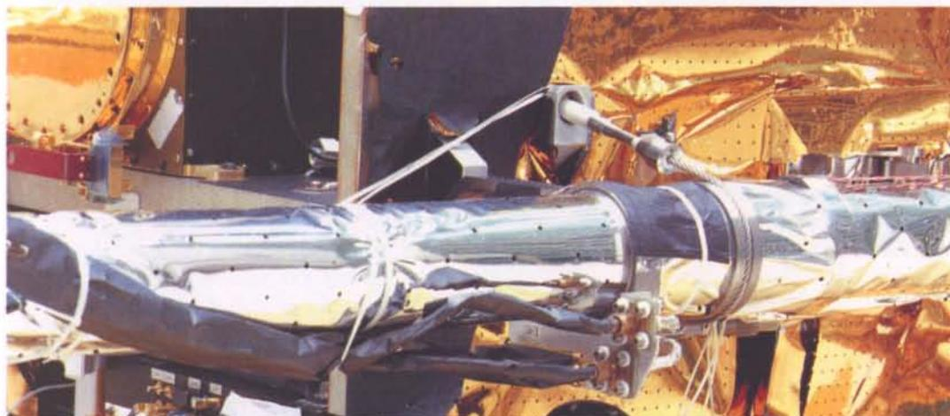
Figure 6. One of the two radial-boom hold-down points
