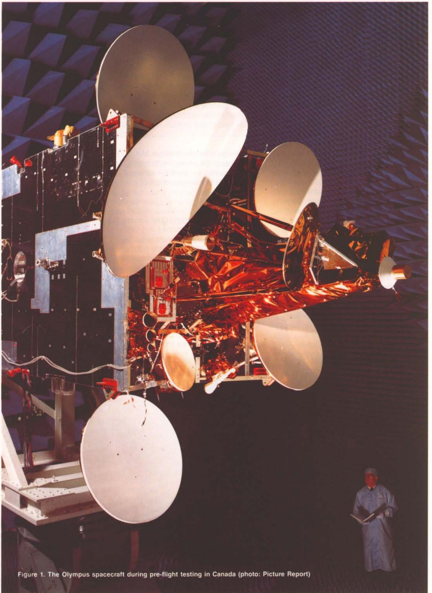
Figure 1. The Olympus spacecraft during pre-flight testing in Canada (photo: Picture Report)
