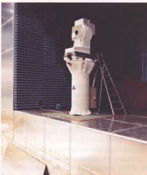
Figure 9. The feedhorn support in the CPTR
