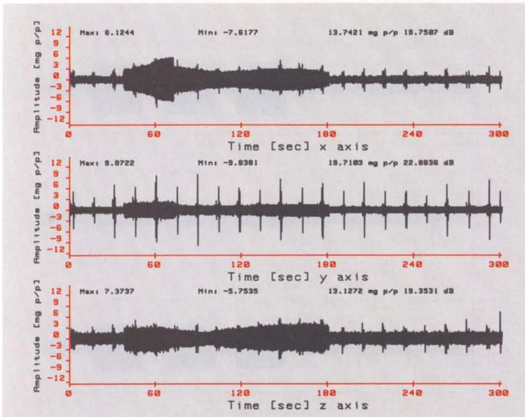
Figure 7. Typical PAX time-domain plot. This run lasted 5 min and all three accelerometer outputs are plotted in parallel
