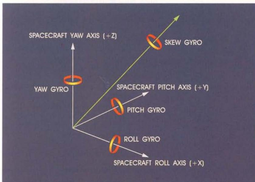
Figure 1. Gyroscope alignment
