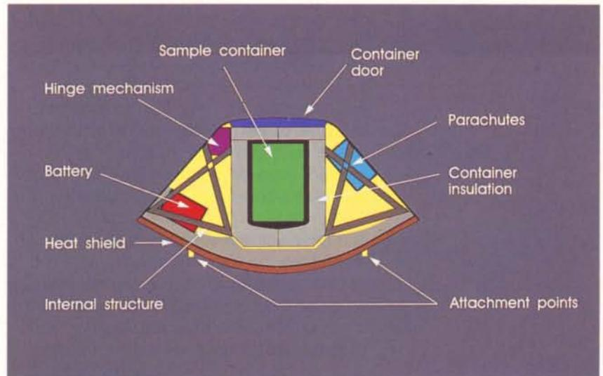
Figure 4. The aerocapsule configuration for the Rosetta mission
