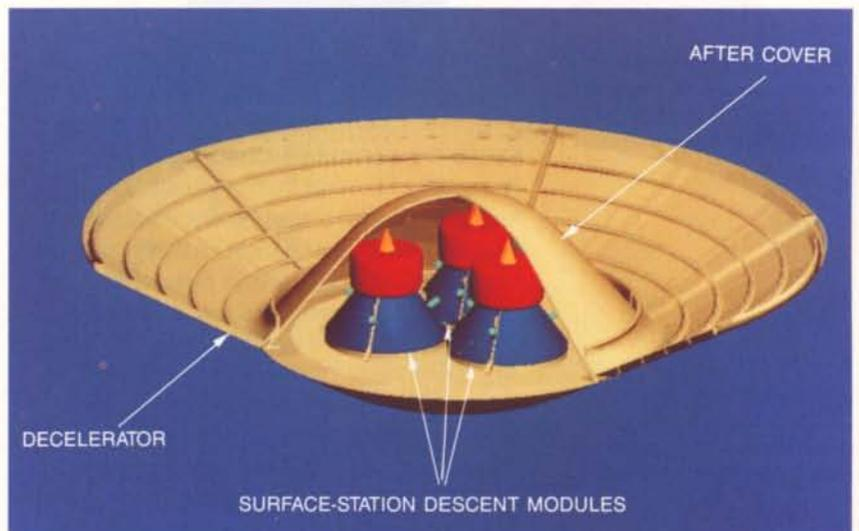
Figure 6. Concept for a surface-station ballistic entry vehicle for the Mars mission
