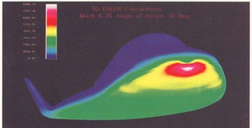
Figure 14. Computed surface-pressure distribution for the Hermes vehicle. Red represents high-, and blue low-pressure areas
