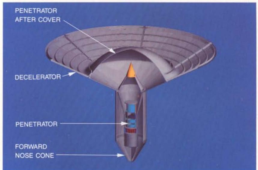
Figure 5. Concept for the penetrator entry-module for the Mars mission
