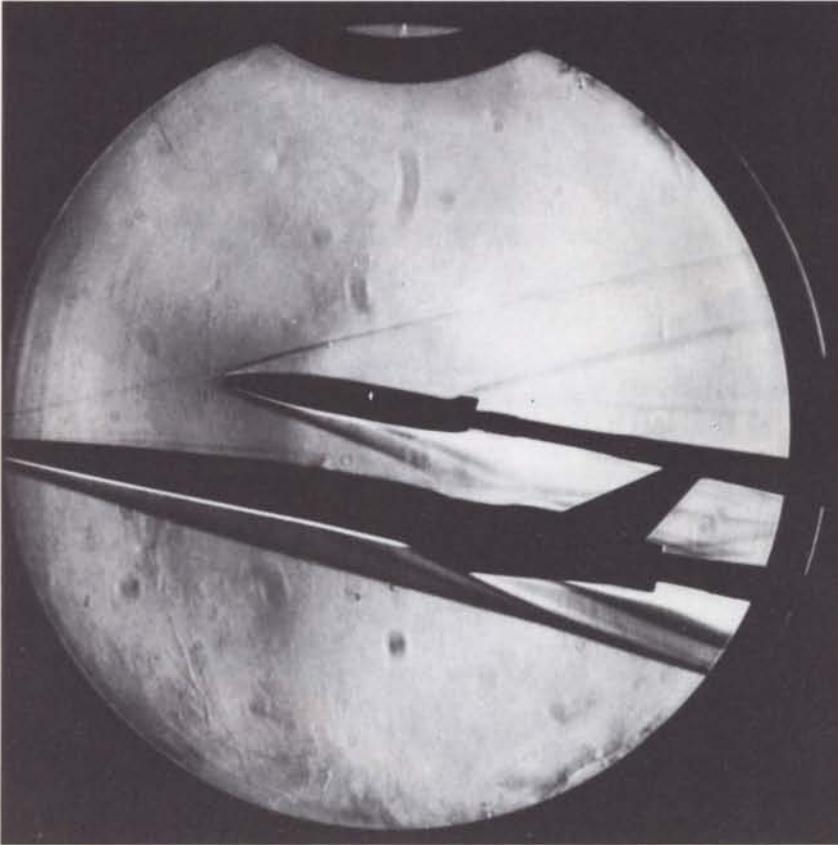
Figure 16. Wind-tunnel testing of a model of Säger (1:160 scale) (courtesy of DLR and MBB)
