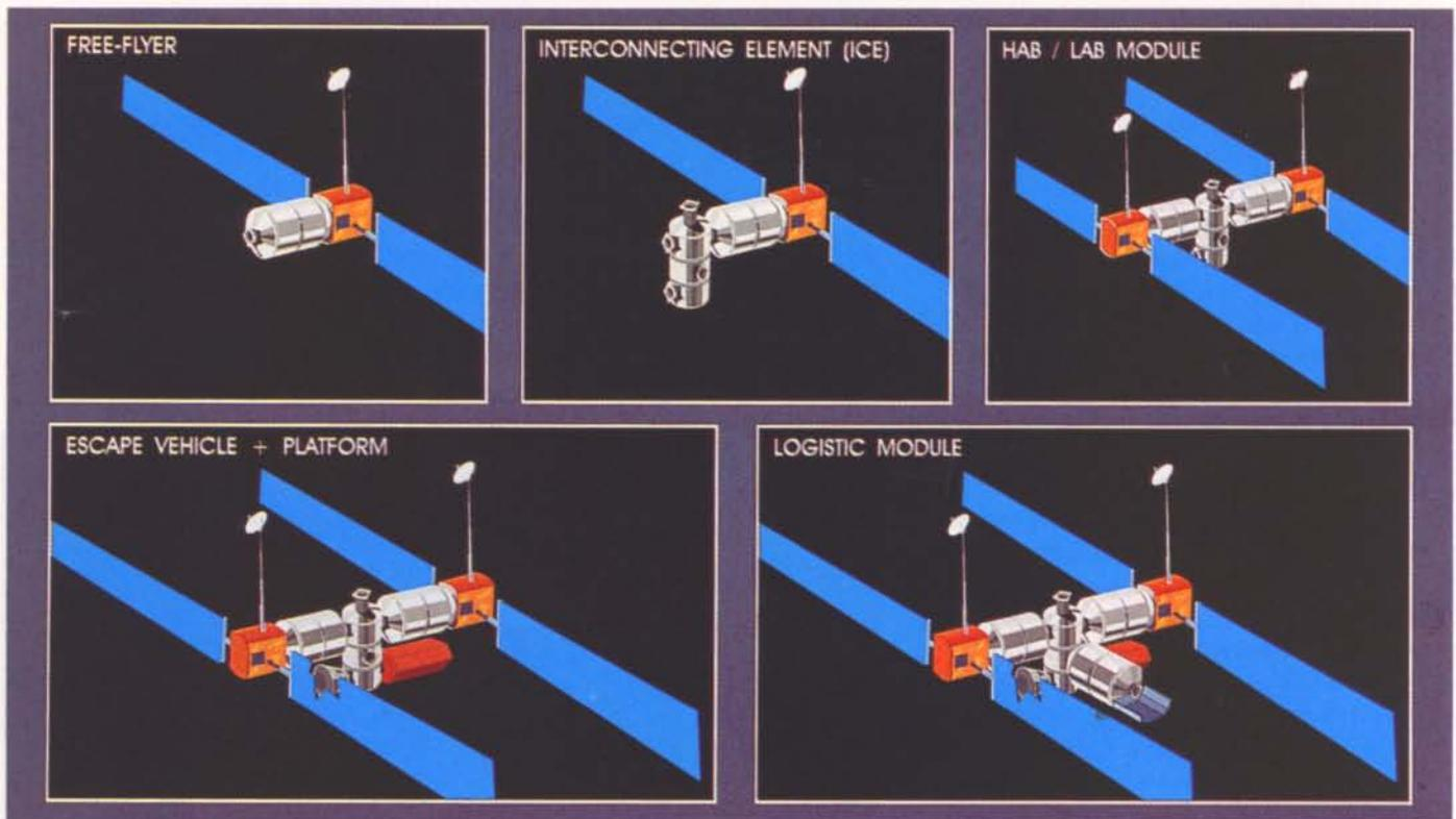
**Figure 3. Study concept for the future European Manned Space Infrastructure (EMSI), showing a five-stage build-up to a permanently manned European Space Station, using Habitation and Laboratory Modules based on the Columbus Free-Flying Laboratory**
