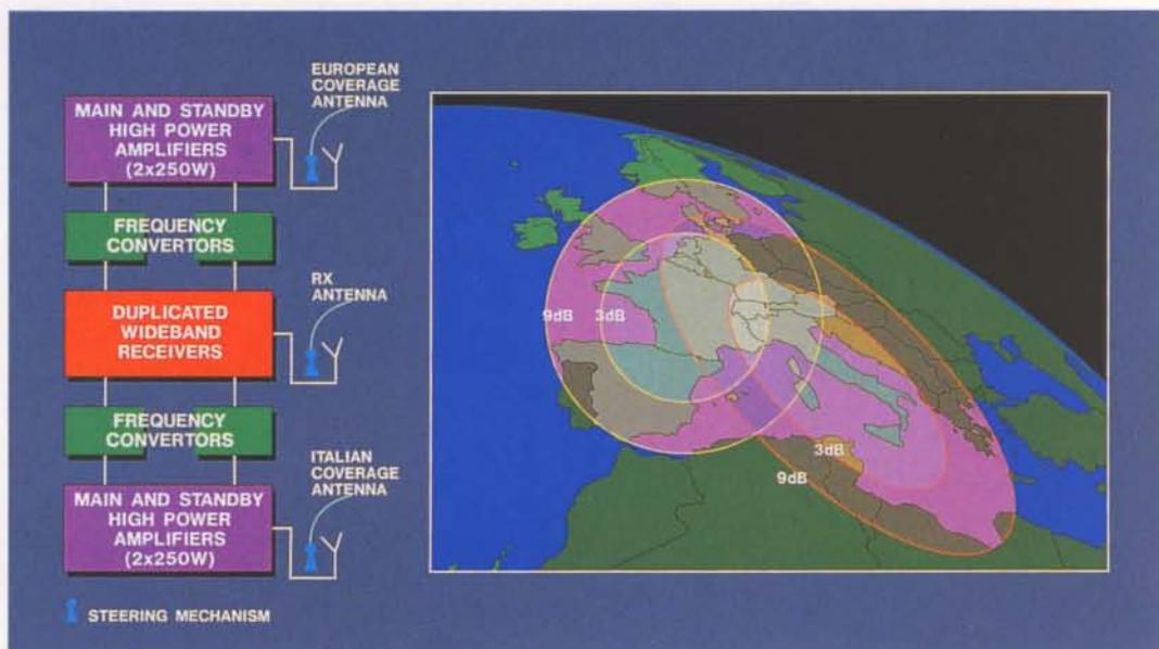
36 MHz when necessary. There are five separate uplink beams to the repeater system and five downlink beams. These use a common feed cluster and a steerable reflector. The receive and transmit sections of the four repeater chains are separated by a 4x4 switch matrix, which can be operated either in a static or dynamic mode. The dynamic mode enables experiments with Satellite-Switched Time-Division Multiple Access (SS-TDMA) to be undertaken.
