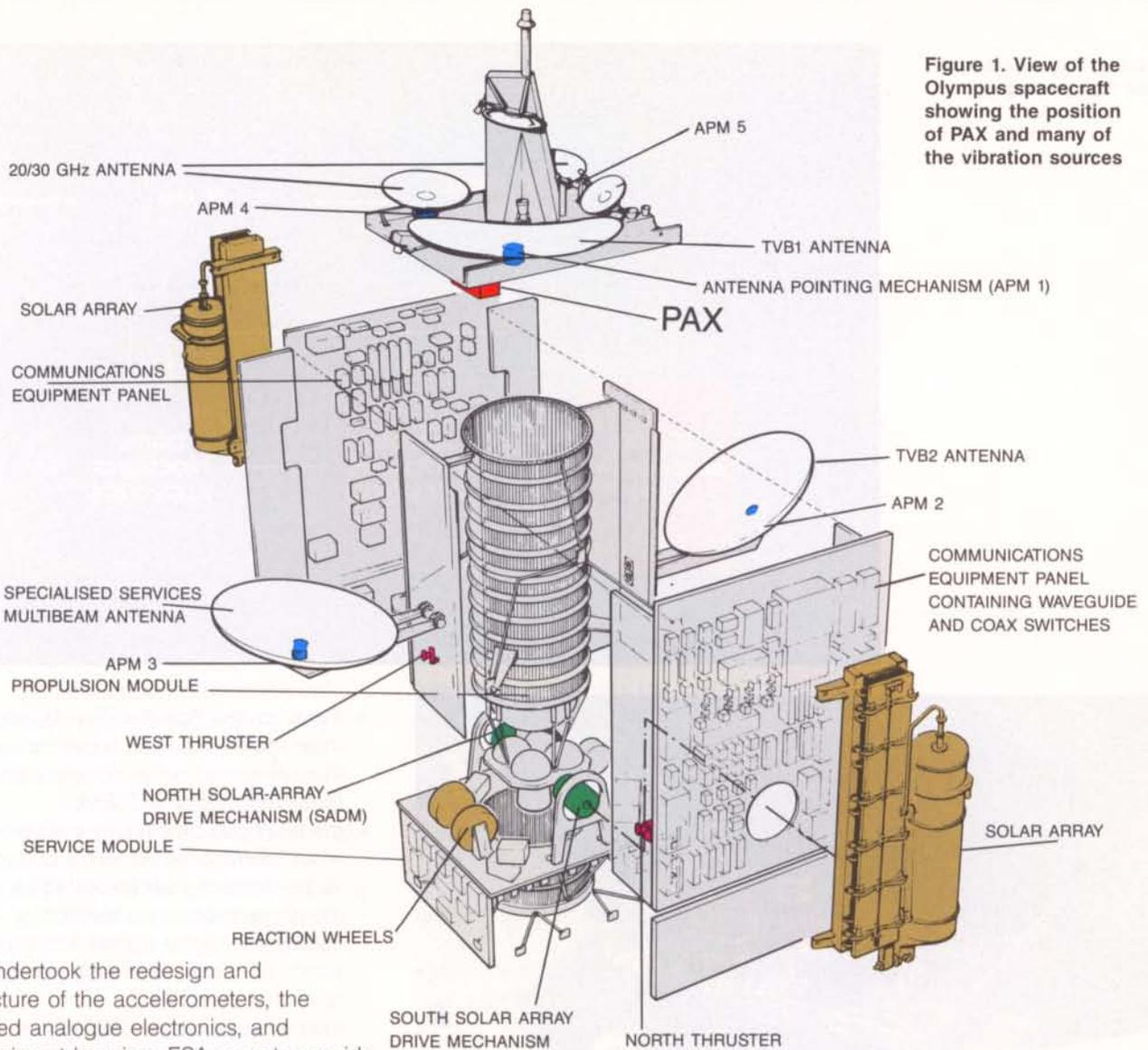
Figure 1. View of the Olympus spacecraft showing the position of PAX and many of the vibration sources
