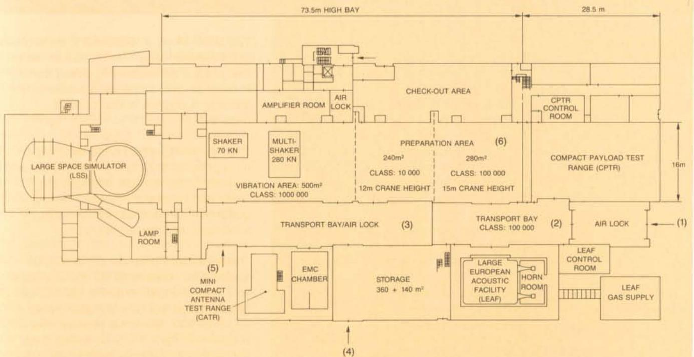
Figure 2. Overall layout of the test and preparation areas
