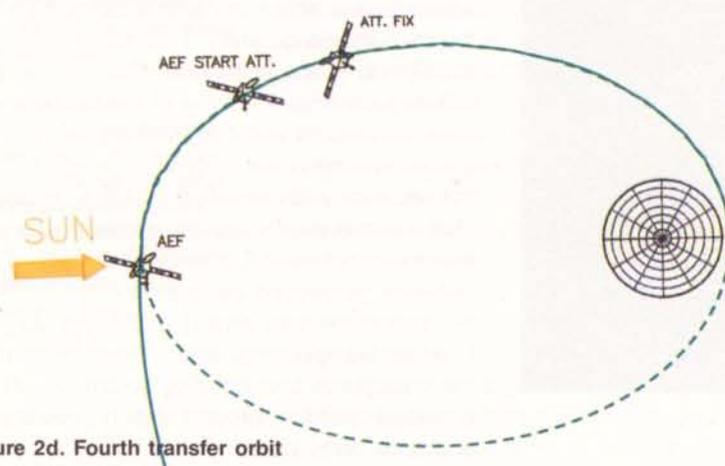
Figure 2d. Fourth transfer orbit
