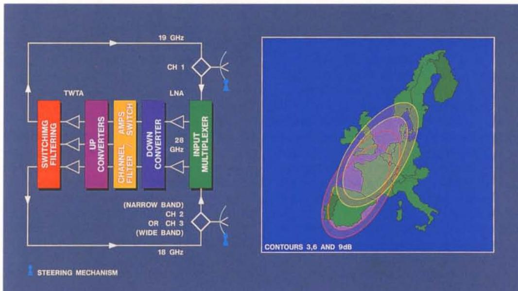
Figure 4. Coverage and simplified schematic of the 30/20 GHz Payload
