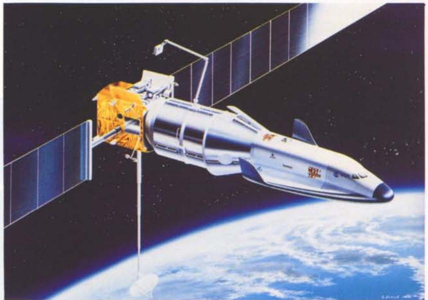
**Figure 9. Artist's impression of Europe's Hermes spaceplane docked with the Columbus Free-Flying Laboratory for servicing purposes**
