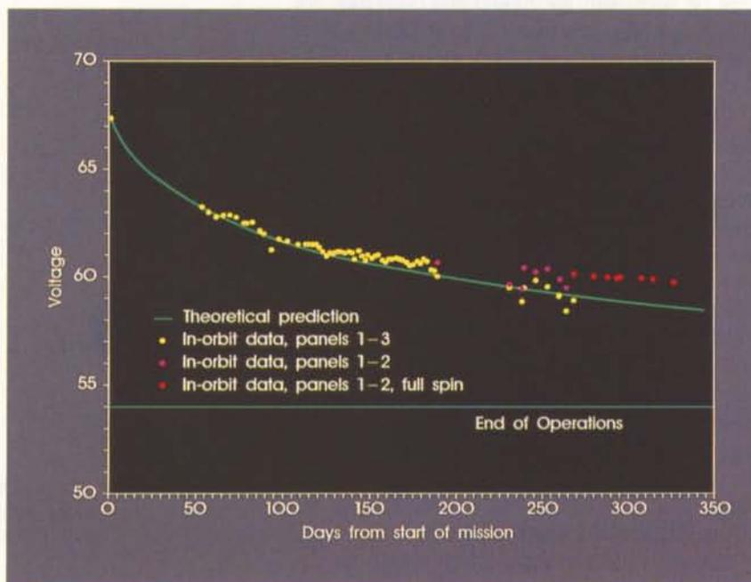
**Figure 5.** The theoretical (green line) and observed (yellow circles) voltages of the Hipparcos solar arrays since launch. Satellite operations can continue as long as the voltage generated exceeds a minimum of about 54 V. Present indications are that a lifetime of more than three years should be achievable.
