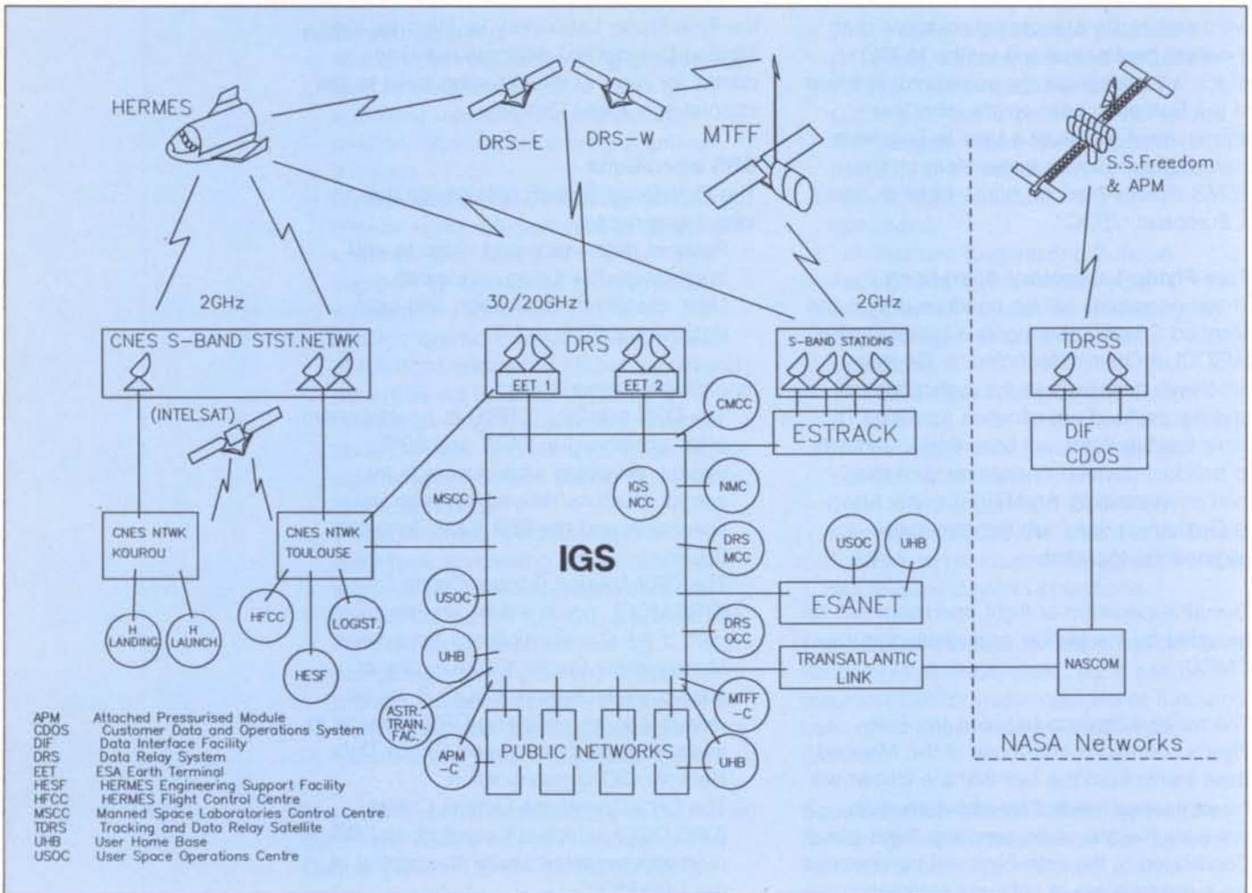
**Figure 1. IOI ground-segment facility interconnections**
