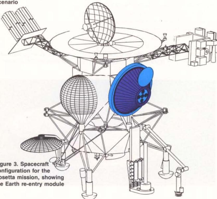
Figure 3. Spacecraft configuration for the Rosetta mission, showing the Earth re-entry module
