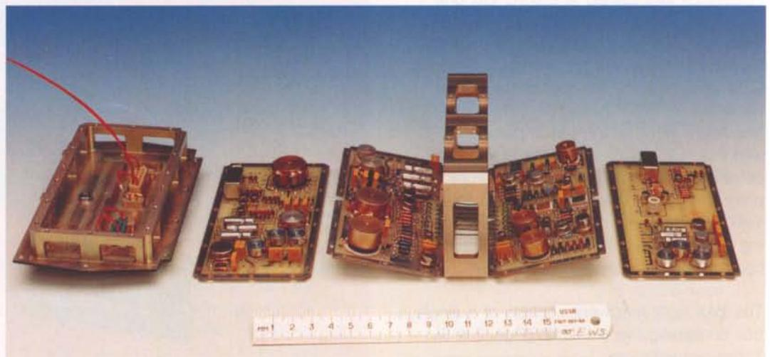
Figure 5. PAX power converter (DC/DC) flight hardware
