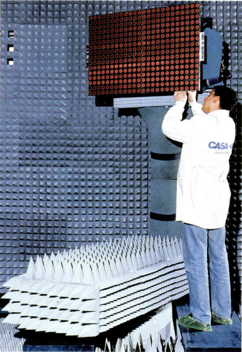
Figure 5. ASAR antenna element breadboard under test
