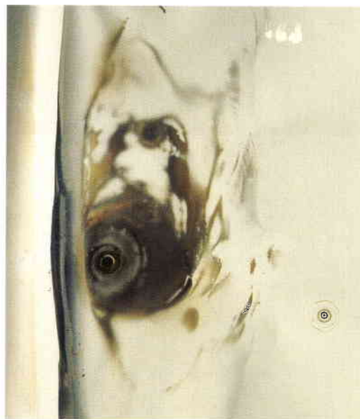
Figure 1. Part of the LDEF surface covered with impact records
