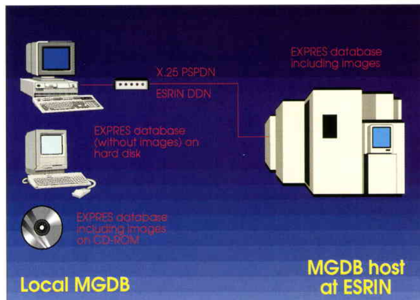
Figure 9. The client-server architecture
