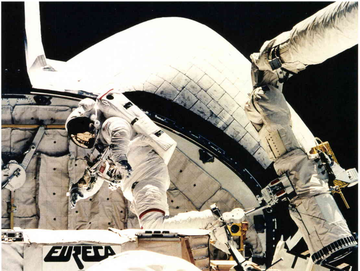
Figure 5. Astronaut David Low, on the end of 'Endeavour's' robotic arm, approaches Eureca, stowed in the Shuttle's cargo bay, to help with the antenna boom latching
