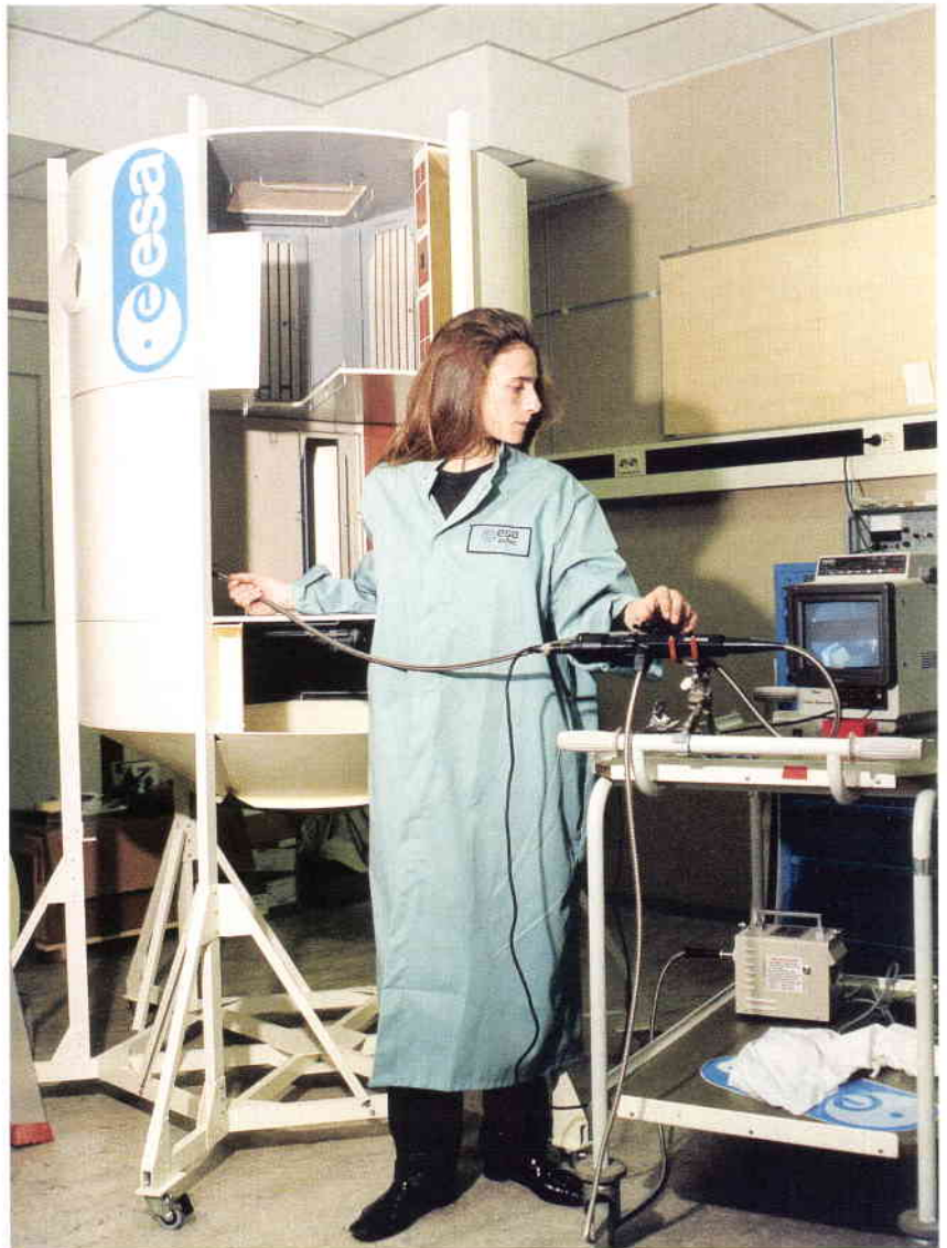
Figure 5. The mock-up — a researcher produces a motion sequence by moving a fibroscope through the mock-up
