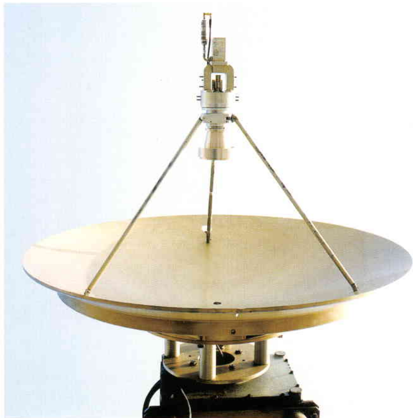
Figure 1. The RA-2 antenna breadboard, with its dual-frequency feed
