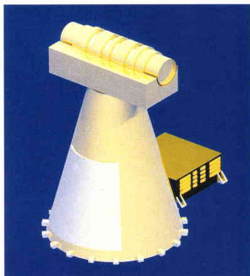
Figure 5. Possible SCARAB configuration for Envisat-1 (Courtesy of J. Pang, ESTEC)
