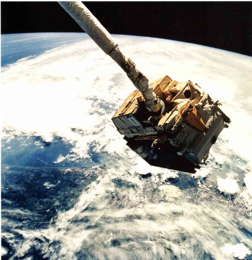
Figure 4. Eureca shortly after being 'grappled' by Space Shuttle 'Endeavour's' robotic arm
