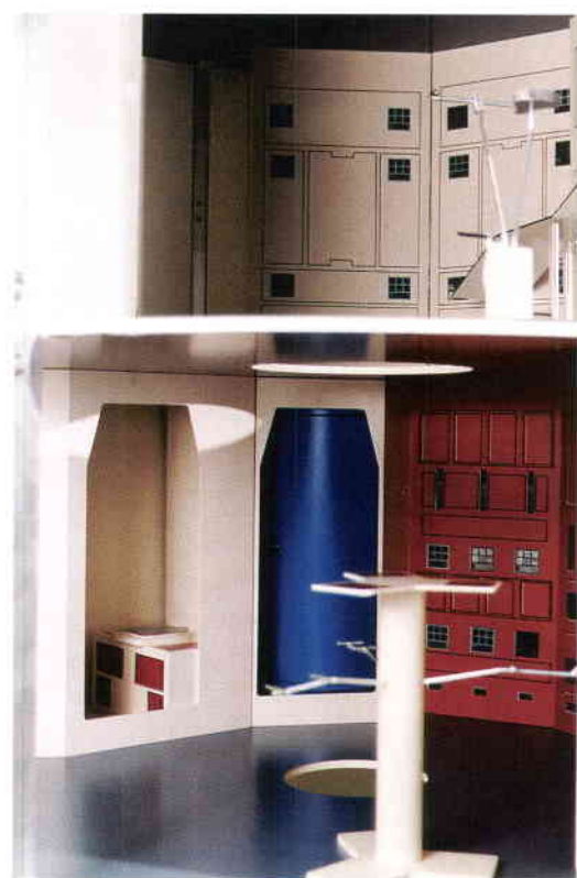
3d. A view of the middle and lower decks of the mock-up. On the middle deck, the exercise equipment is shown. On the lower deck, the wardroom table (foreground) and the galley (in brown), shower booth (in blue) and toilet (left) are shown.
