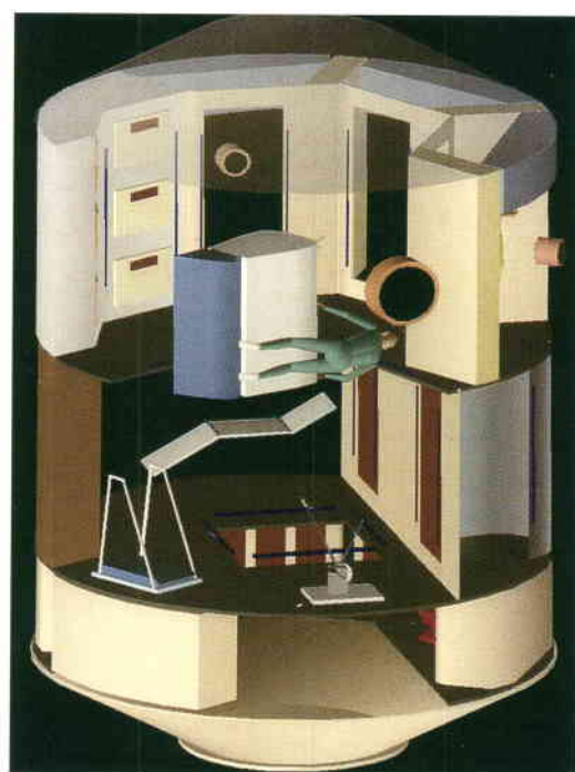
2b. A DYNAMAN view of the configuration. The astronaut is at the wardroom table, which is oriented in a different way than the surrounding environment.
