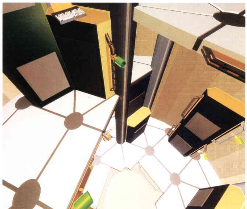
4d. A STAR view down the centre line, showing the modular construction of the half-decks. A portable workstation (keyboard at the top left) gives an idea of the scale.
