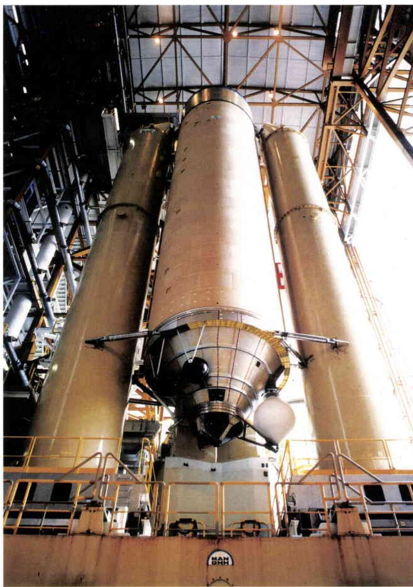
**Figure 12. MDO1 campaign: the cryogenic stage and booster mock-ups in the integration building**
