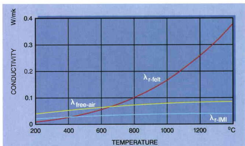
Figure 11. Conductivities of felt- and IMI-type insulations as a function of temperature
