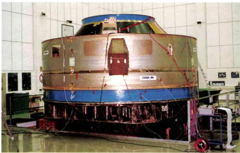
**Figure 8.** The vehicle equipment bay and L9 stage awaiting the combined vibration test
