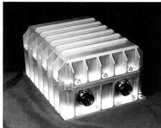
heaters activate below +10°C. During initialization, recording is disabled until heaters can stabilize the internal environment above 0°C. Shock and vibration isolation allow the tape transport assembly to surpass Shuttle launch and landing requirements.
