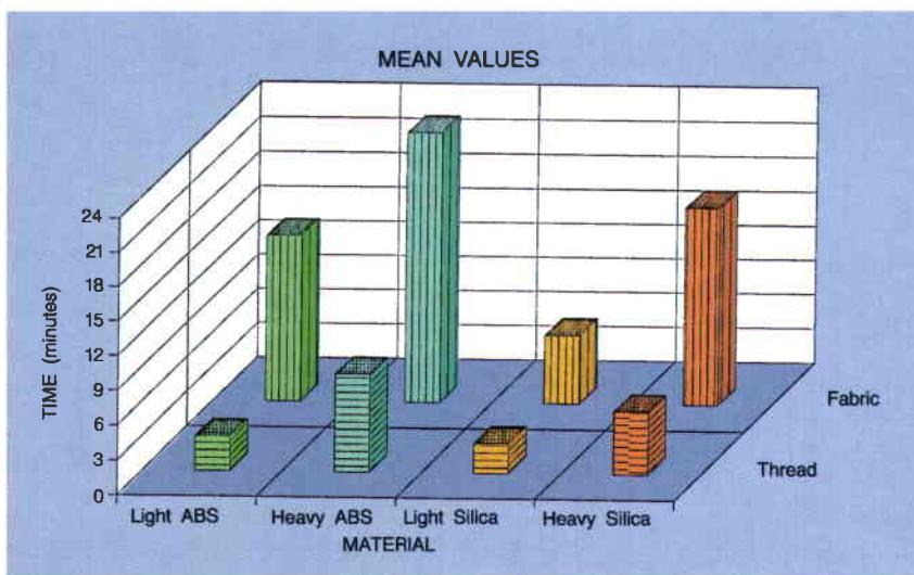
Figure 9. Acoustic performance as a function of component material (time to first failure at 168 dB)
