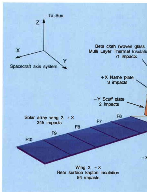
**Figure 2.** The Eureca spacecraft's configuration, and the numbers of impact events recorded on its various components
