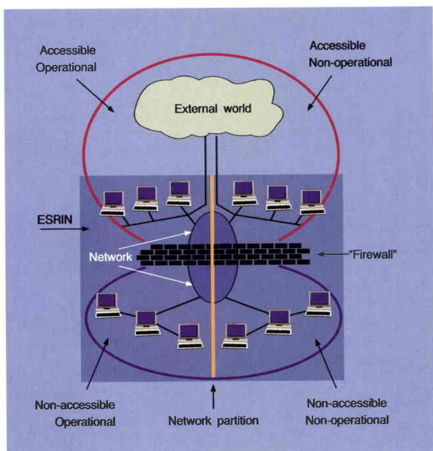
Figure 4. Four categories of network have been created. All host computers offering an operational service, whether they are accessible or non-accessible, are connected to different networks than those used for development or office support (non-operational)
