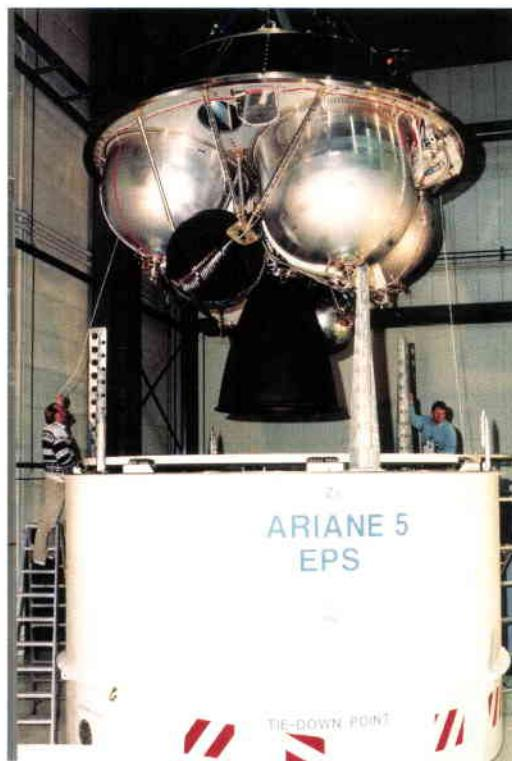
**Figure 11. The L9 stage being installed in its container**
