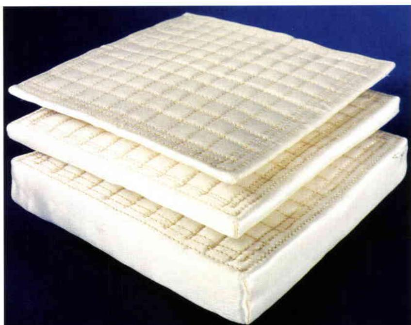
Figure 10. Flexible External Insulation (FEI) blanket sample
