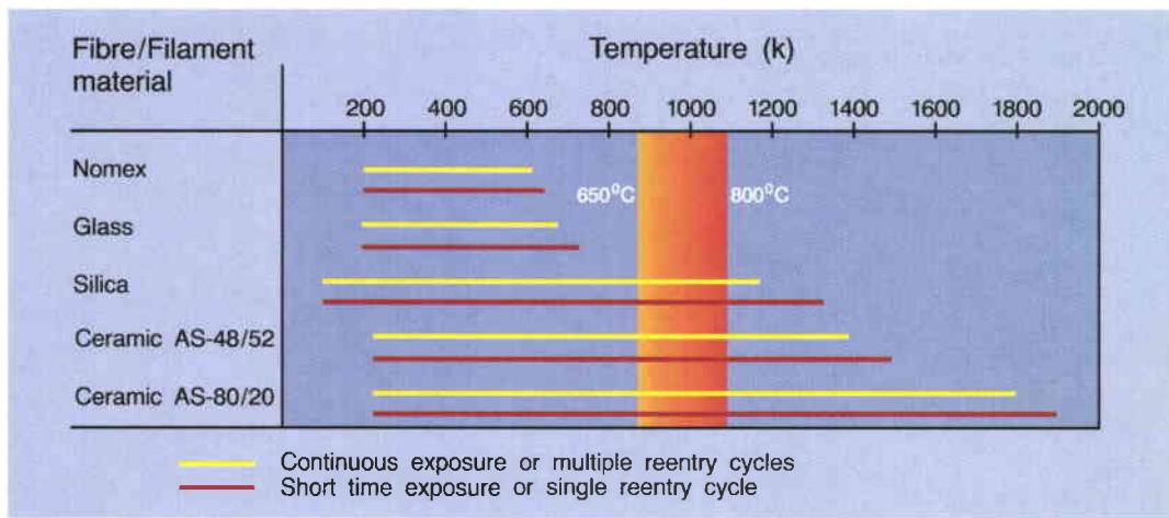
Figure 5. Material/component selection guide
