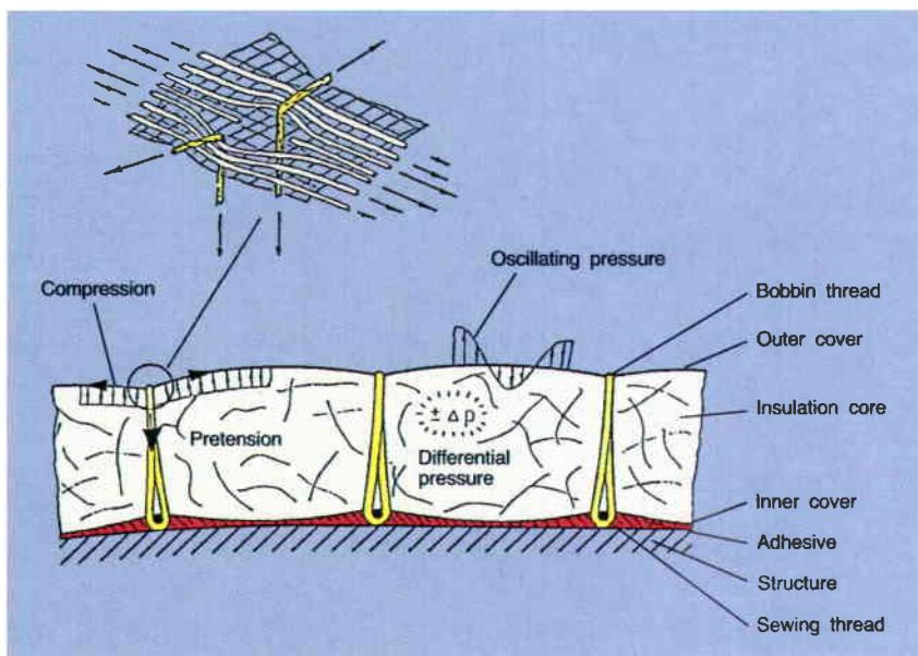
Figure 8. Schematic of the structural load system
