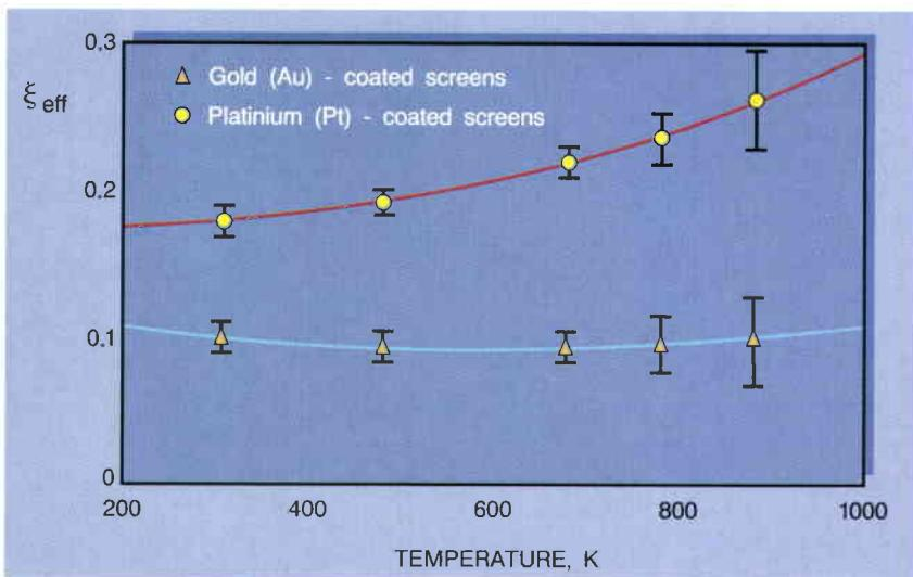
Figure 13. Effective emissivities of gold- and platinum-coated screens (measured at ZAE in Würzburg, Germany)
