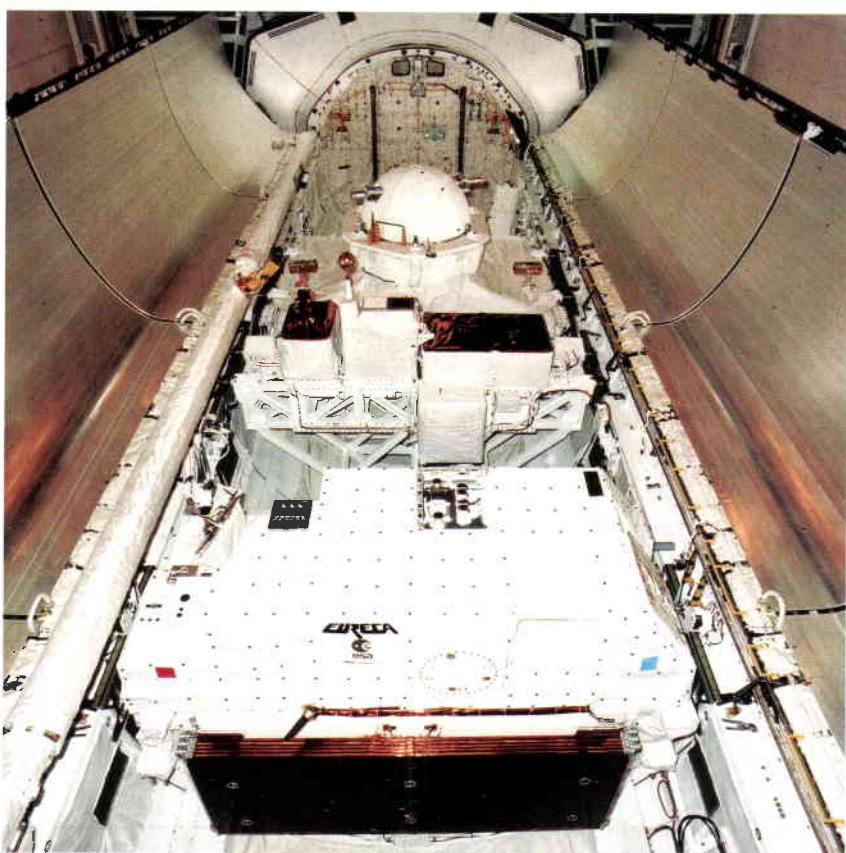
**Figure 1.** The European Retrievable Carrier 'Eureca' in the payload bay of the Space Shuttle prior to launch (STS-46)
