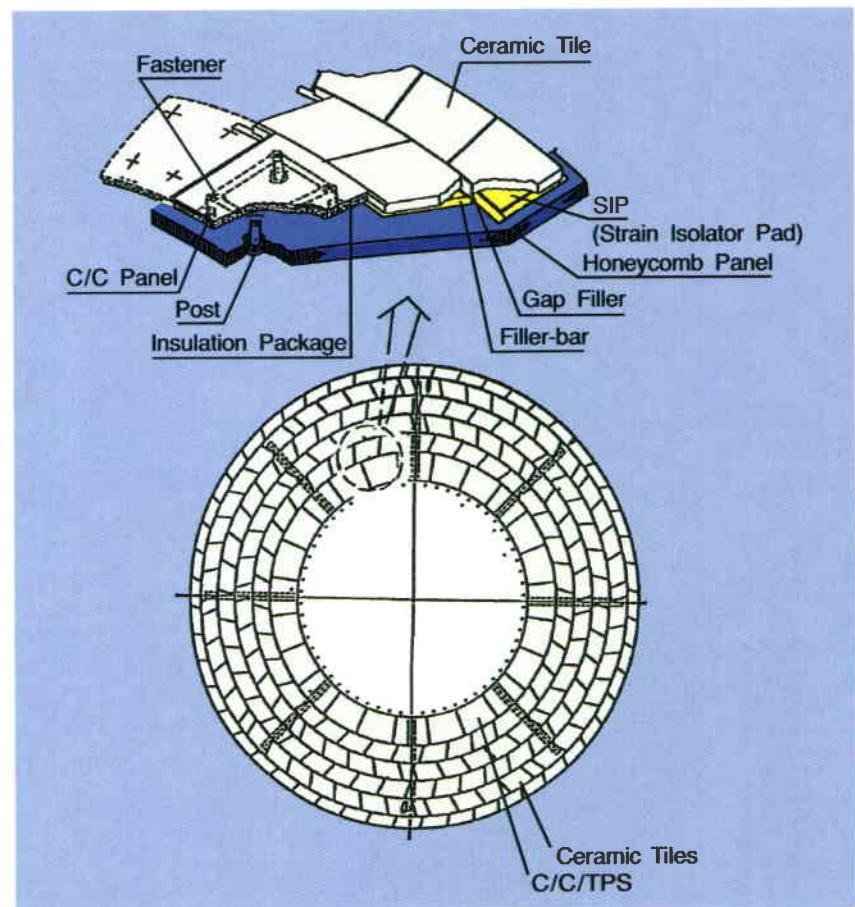
**Figure 1. OREX thermal-protection concept (courtesy of NASDA)**
