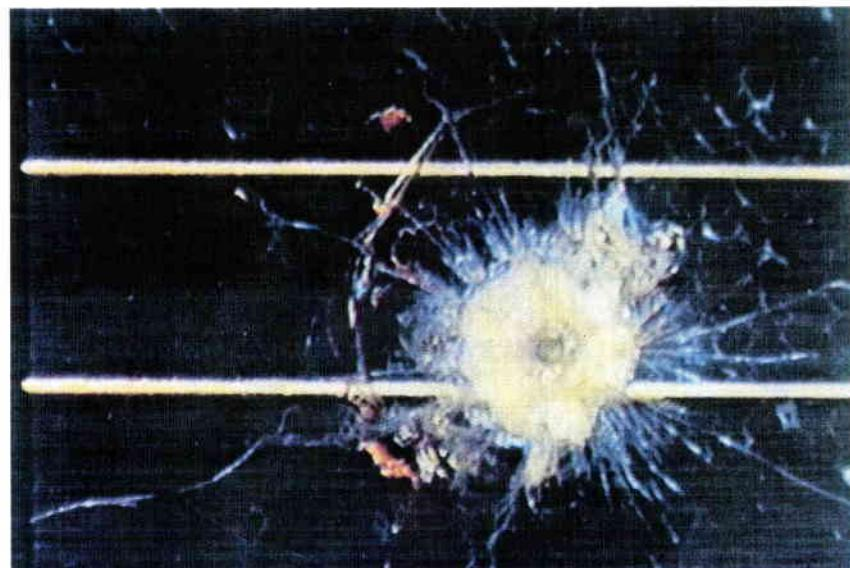
**Figures 5 — 7. Typical solar-cell impact features**
