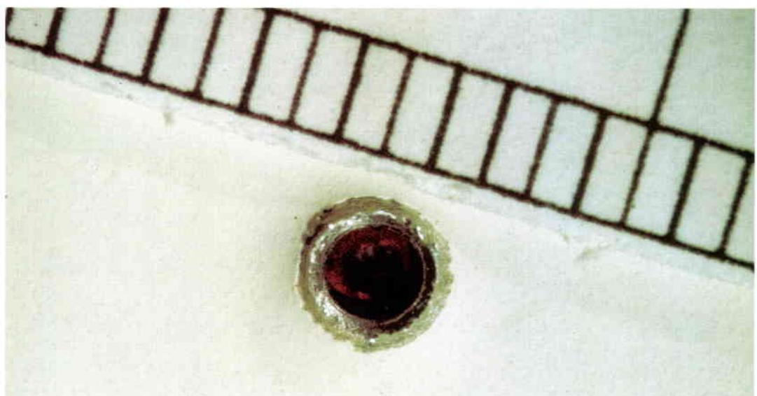
**Figure 4. A 2 mm impact hole in one of the aluminium ESA logo plates**
