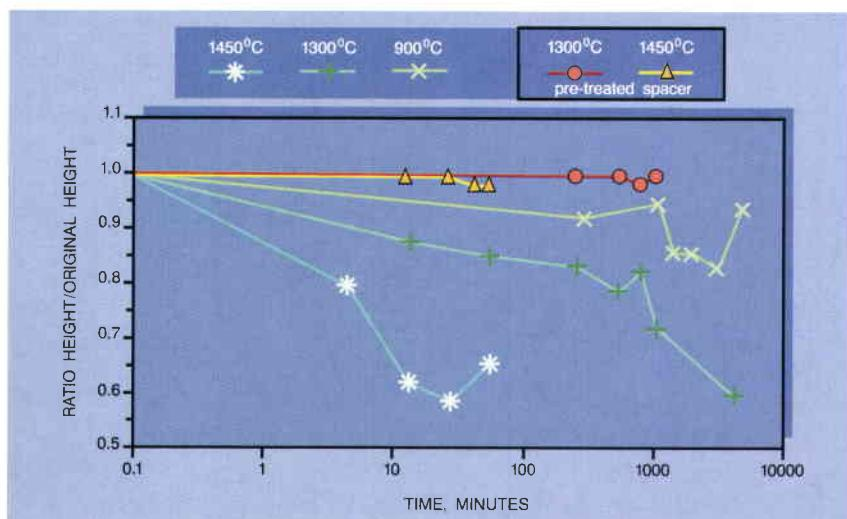
Figure 14. Spacer resilience as a function of mechanical loading before and after manufacturing improvement
