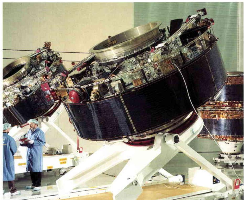
on the instruments prior to them being reintegrated early in 1995 in preparation for delivery. Most sensors on PFM, F2 and F3 will be exchanged, whilst some sensitive components of the F4 sensors may also be included in the refurbishment programme. This programme ensures that only prime-quality detectors will be flown on the mission.
