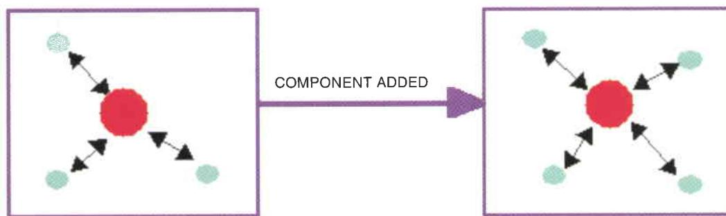
**Figure 2. Client-server communication between software components. The addition of a new component means that only the interface with the new component must be provided.**
