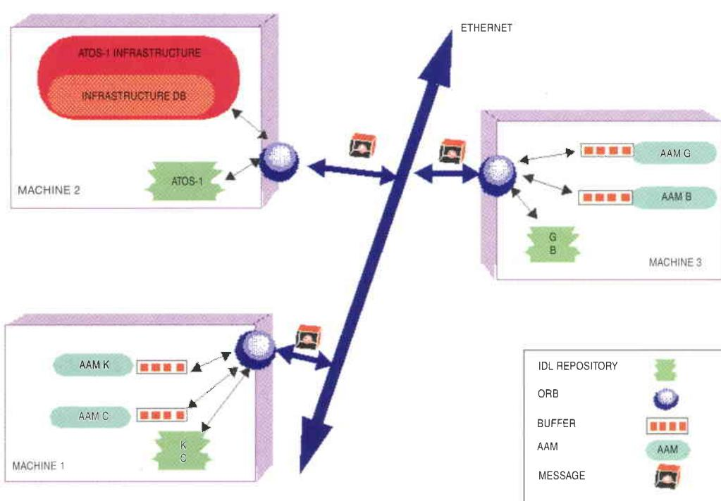
**Figure 8. ATOS architecture based on Common Object Request Broker Architecture (CORBA)**
