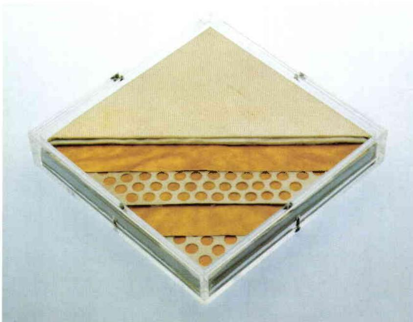
testing has demonstrated the very favourable damping behaviour of the IMI and shingle/IMI systems when exposed to acoustic loads.
