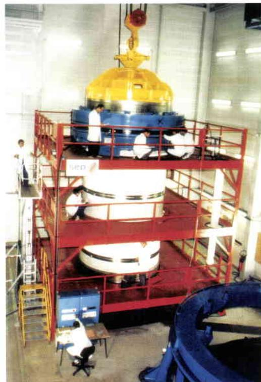
**Figure 2. Preparing for the testing of the booster joints**
