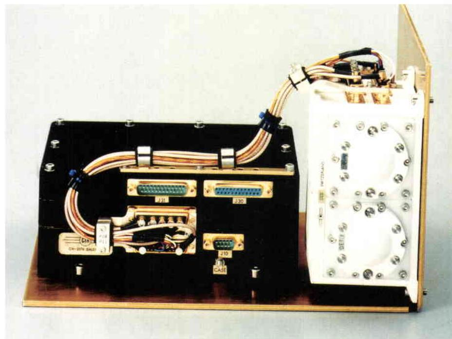
*The Radiation Environment Monitor (REM) in the STRV configuration. The white box is mounted on the outside of the spacecraft with a clear view into space. The REM counts the electrons and protons that penetrate the shielding (two white domes, on right) and reach the silicon detectors*
