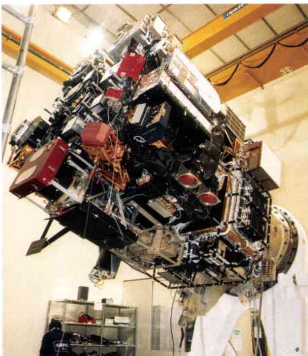
**Figure 2. The SOHO payload module, without thermal blankets, after integration and testing at Matra Marconi Space in Toulouse (F)**
