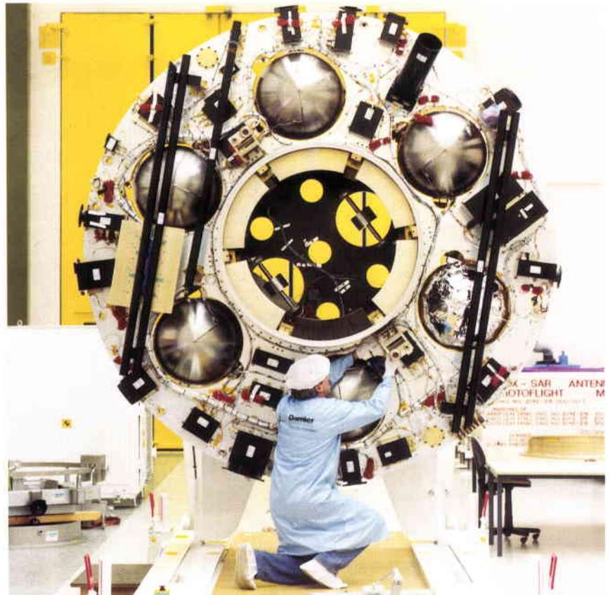
Figure 5. The Cluster Structural Model spacecraft during integration. The six propellant tanks, booms, main platform and central cylinder are visible, together with the harness and mass dummies of the various units
