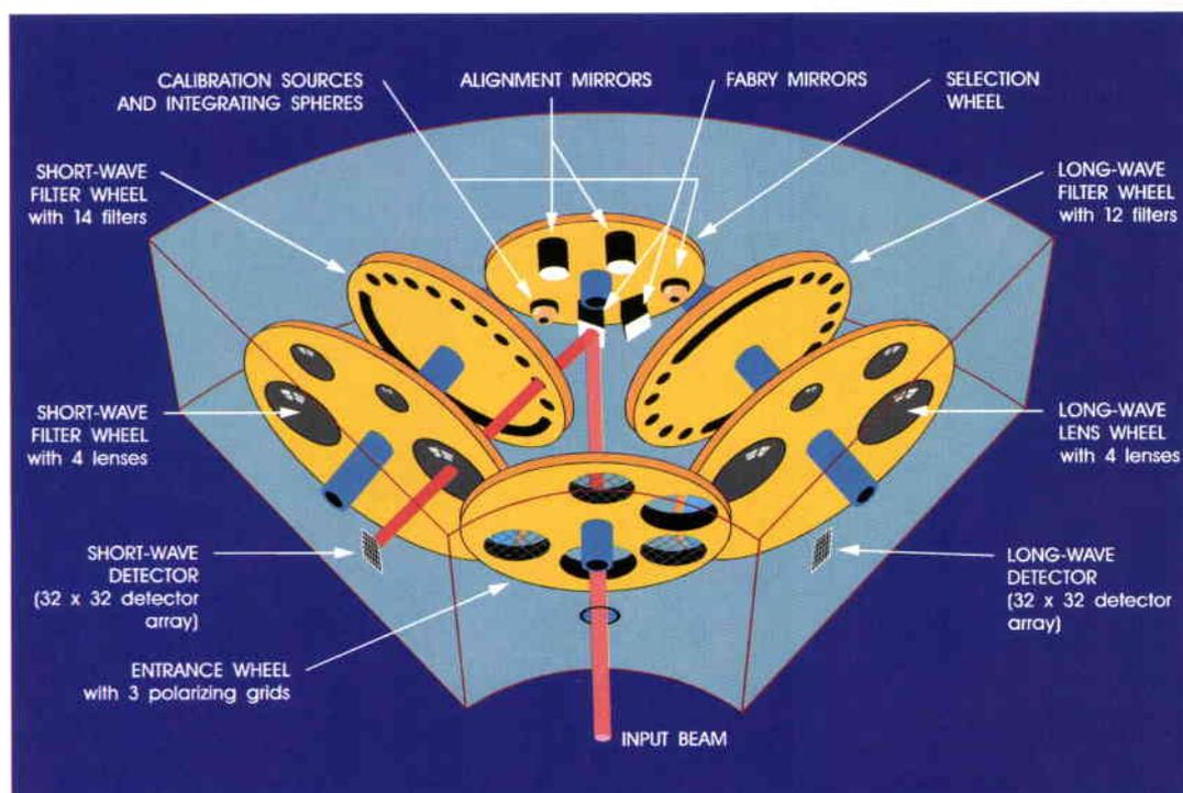
Figure 2. Schematic of the ISOCAM instrument's opto-mechanical design
