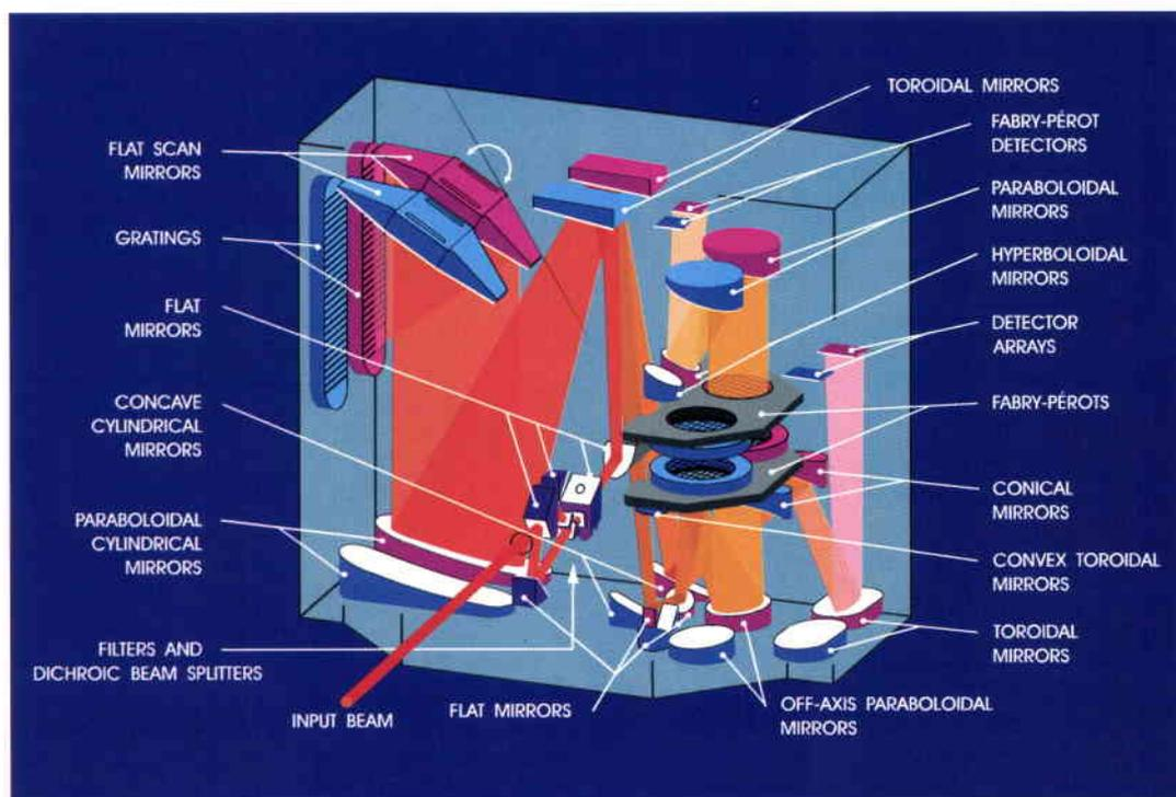
**Figure 4. Schematic of the SWS instrument's opto-mechanical design**
