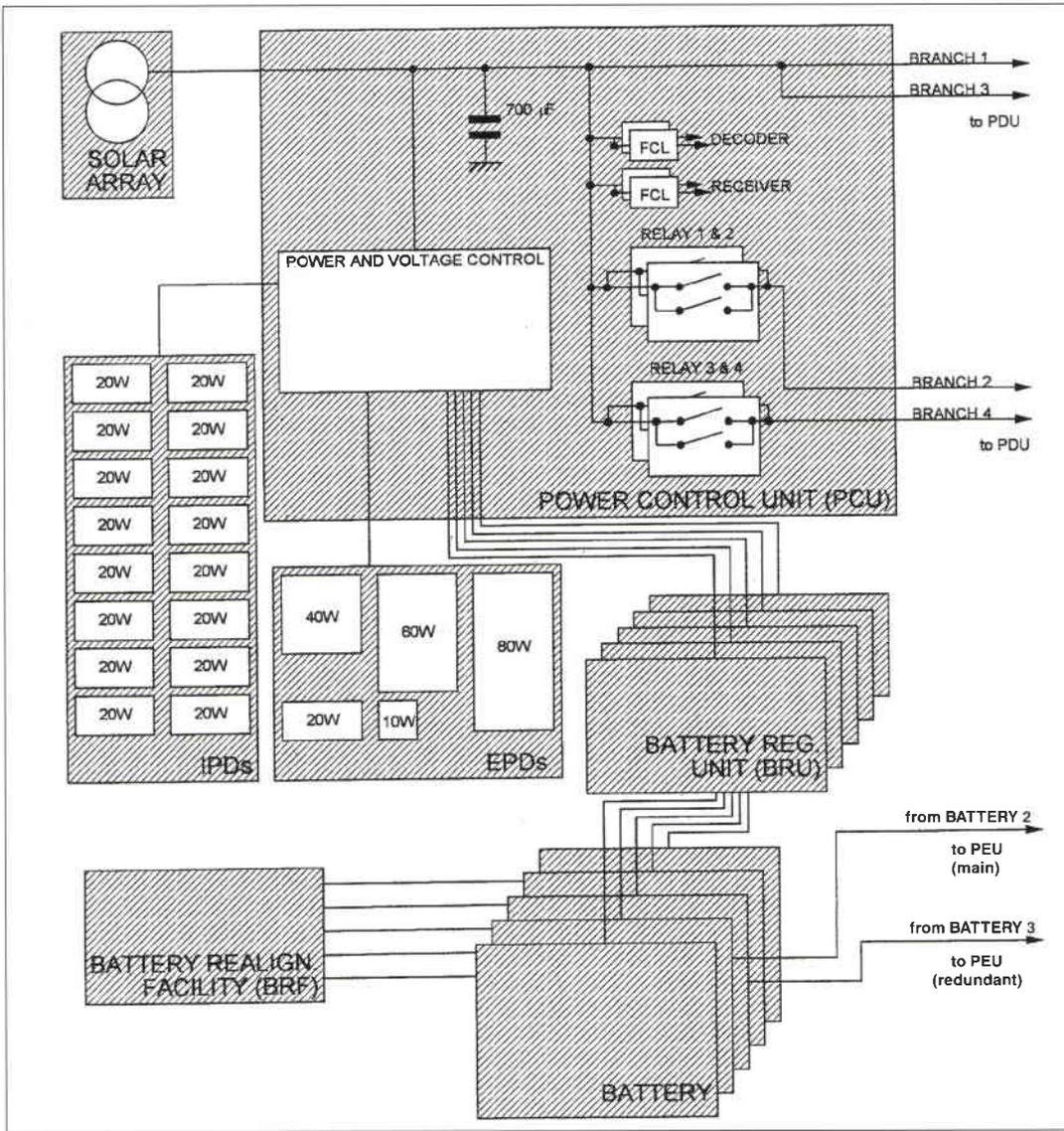
Figure 9. The Cluster power subsystem
