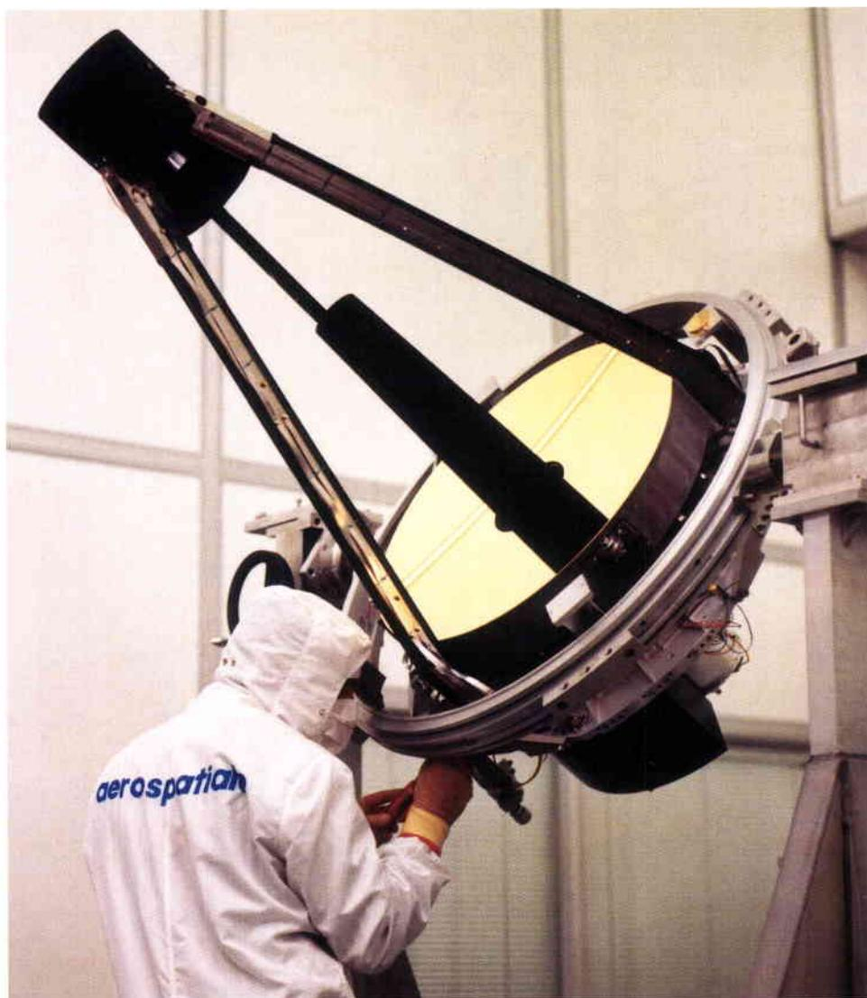
With these viewing constraints, the total stray light falling on the instruments must be less than 10% of the diffuse zodiacal background. This requirement is fulfilled by means of the main baffle with sharp-edged vanes surrounding the telescope, Cassegrain baffles around the secondary mirror and the central hole of the primary, and a gold-coated truncated-cone Sun shade that reflects direct illumination from the Earth back to space (Fig. 4).
