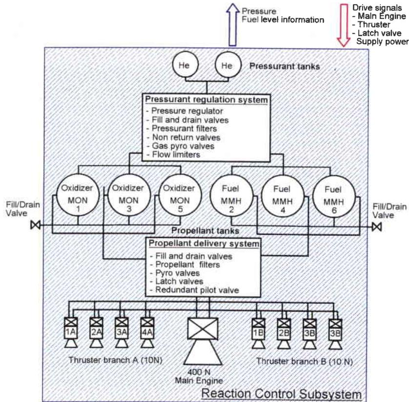
**Figure 6. The Reaction Control Subsystem (RCS)**
