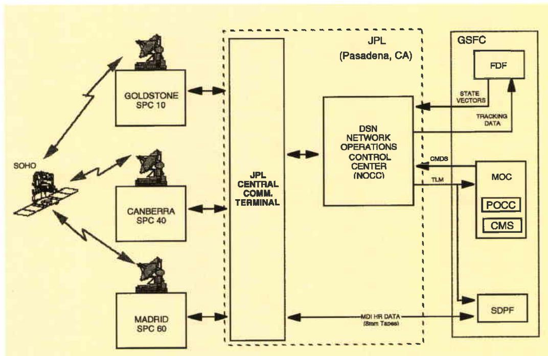
Figure 2. The NASA/JPL Deep-Space Network (DSN) interfacing for SOHO
