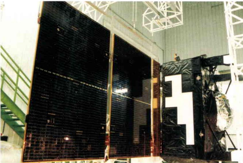
**Figure 3. Deployment testing of SOHO's solar arrays, at Intespace in Toulouse (F)**
