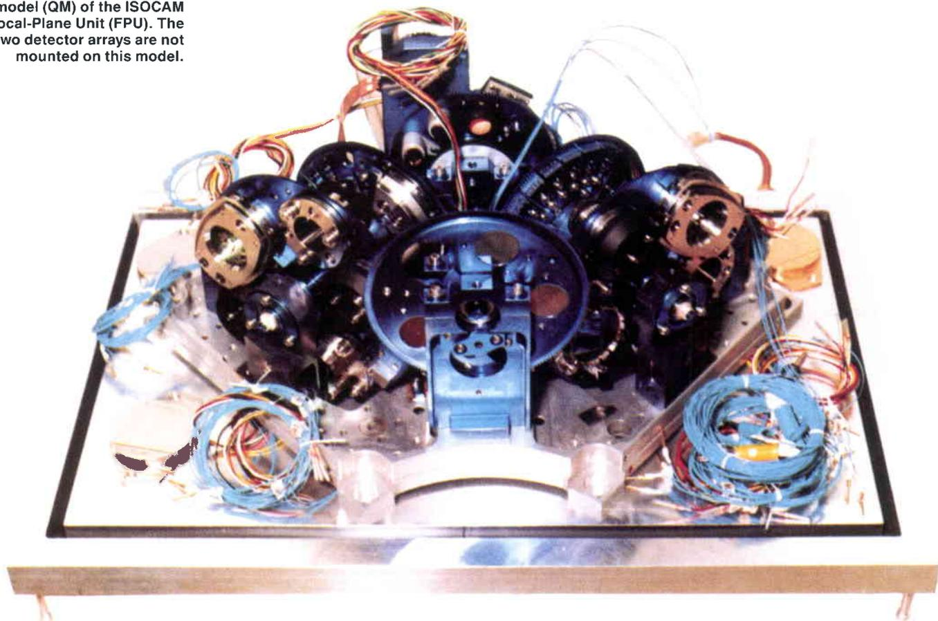
Polarisers allow different orientations of the electromagnetic field vectors of the infrared radiation to be distinguished.
