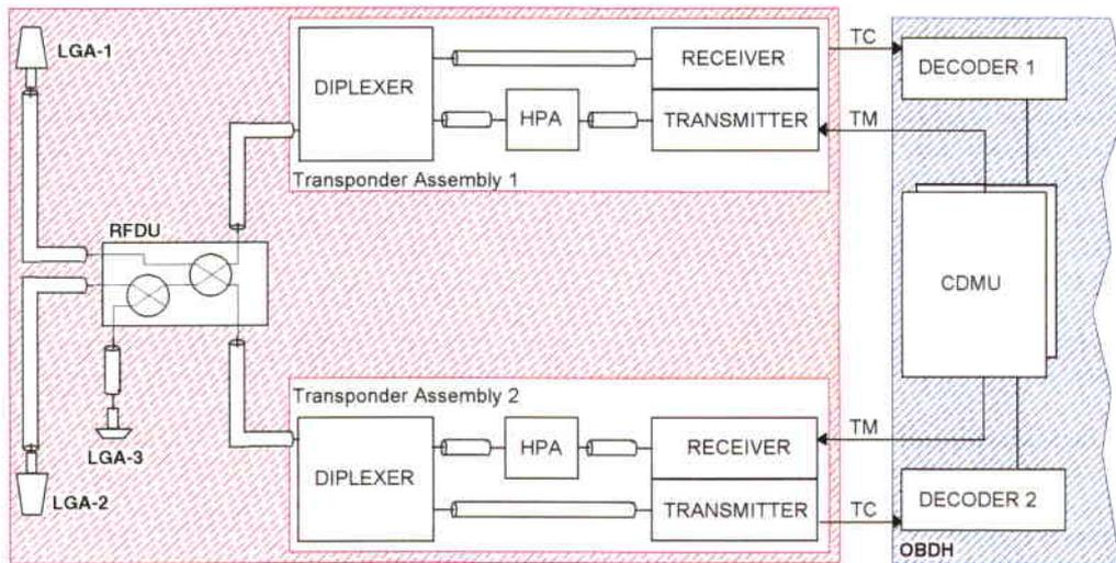
**Figure 12. The Cluster telecommunications subsystem**
