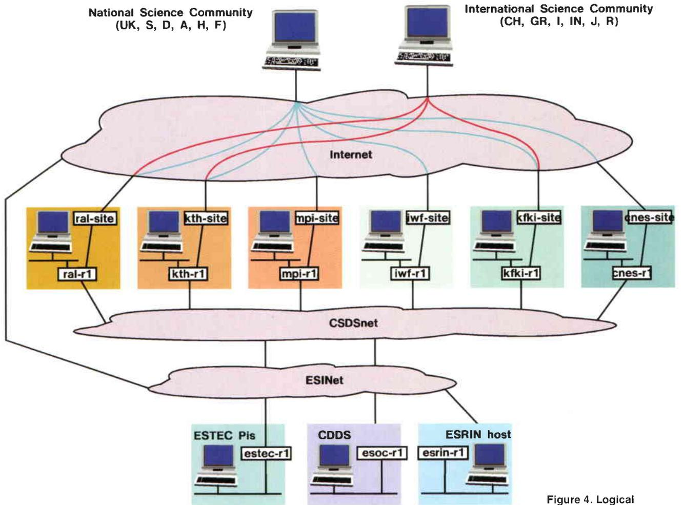
Figure 4. Logical connectivity supported by the CSDSnet
