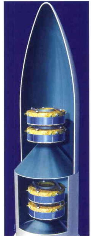
Figure 2. The Cluster launch configuration aboard Ariane-5
