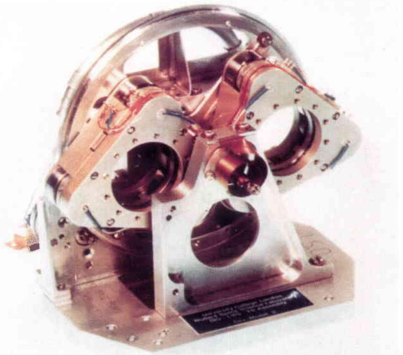
**Figure 6. The two Fabry-Pérot etalons of the LWS mounted on the exchange wheel**
