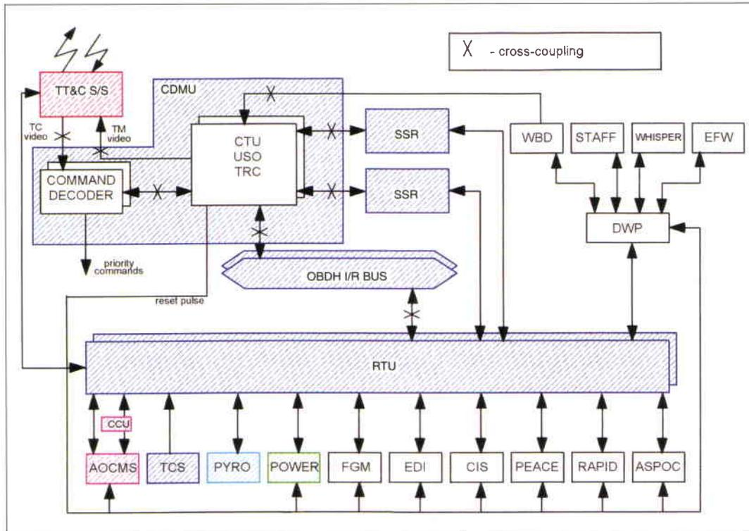
Figure 10. The Cluster onboard data-handling subsystem
