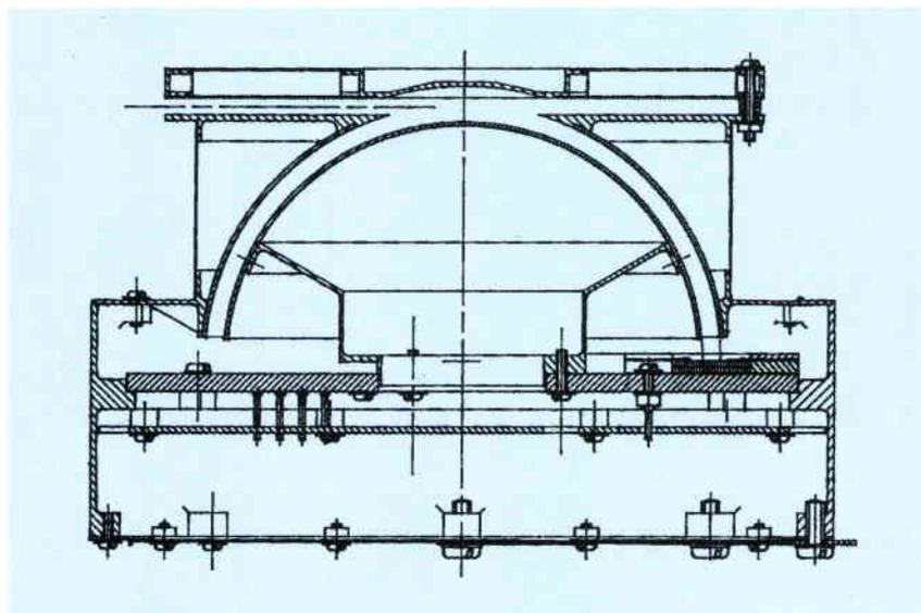
Figure 2a. The original mounting of the PEACE hemispheres
