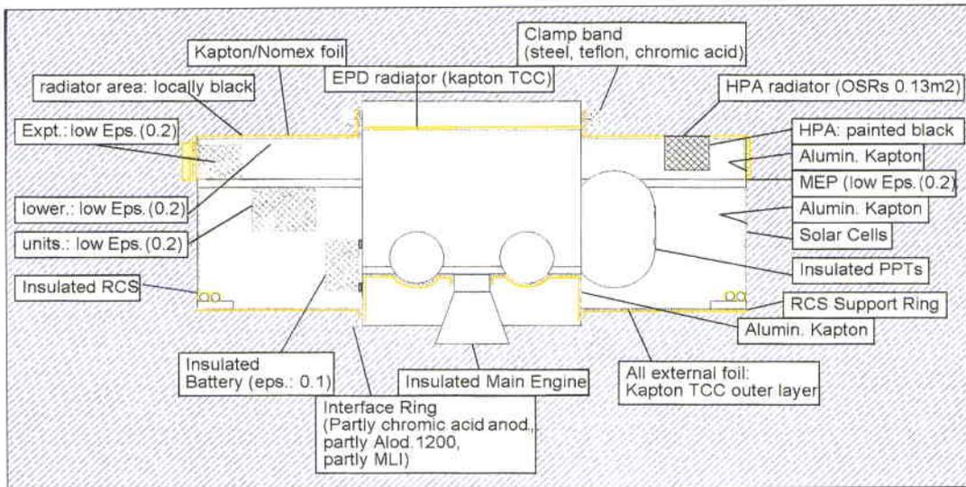
Figure 7. The Cluster thermal-control concept
