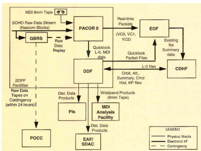
**Figure 5. The Sensor Data Processing Facility (SDPF) interfacing for SOHO**
