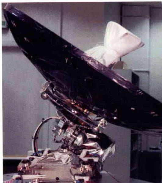
Figure 5. The High-Gain Antenna (HGA) assembly
