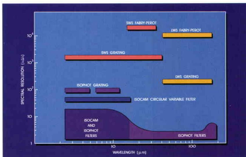
Figure 3. Spectroscopic and photometric capabilities of the ISO scientific instruments.
