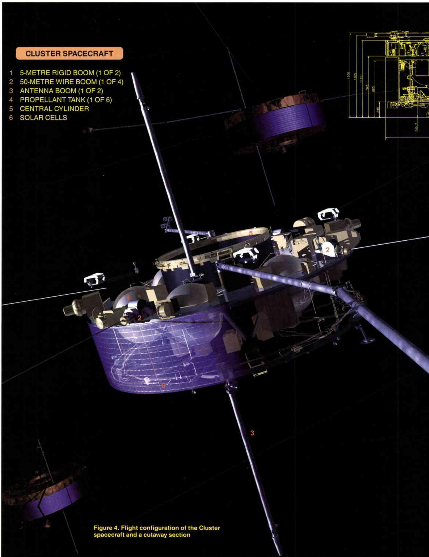
Figure 4. Flight configuration of the Cluster spacecraft and a cutaway section
