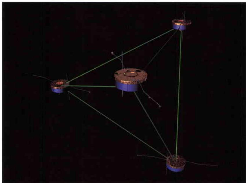
**Figure 3. The tetrahedral formation in orbit. The four Cluster spacecraft are placed in slightly different orbits, which ensures that at a specific point in space they form the vertices of a tetrahedron. This will allow true three-dimensional measurements to be made in the regions of primary scientific interest**
