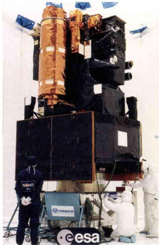
**Figure 1. The SOHO spacecraft in launch configuration prior to acoustic testing at Intespace in Toulouse (F)**
