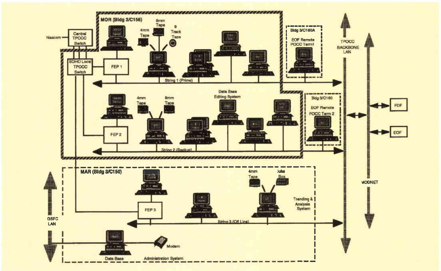
**Figure 4. Baseline architecture of the SOHO Payload Operations Control Center (POCC)**
