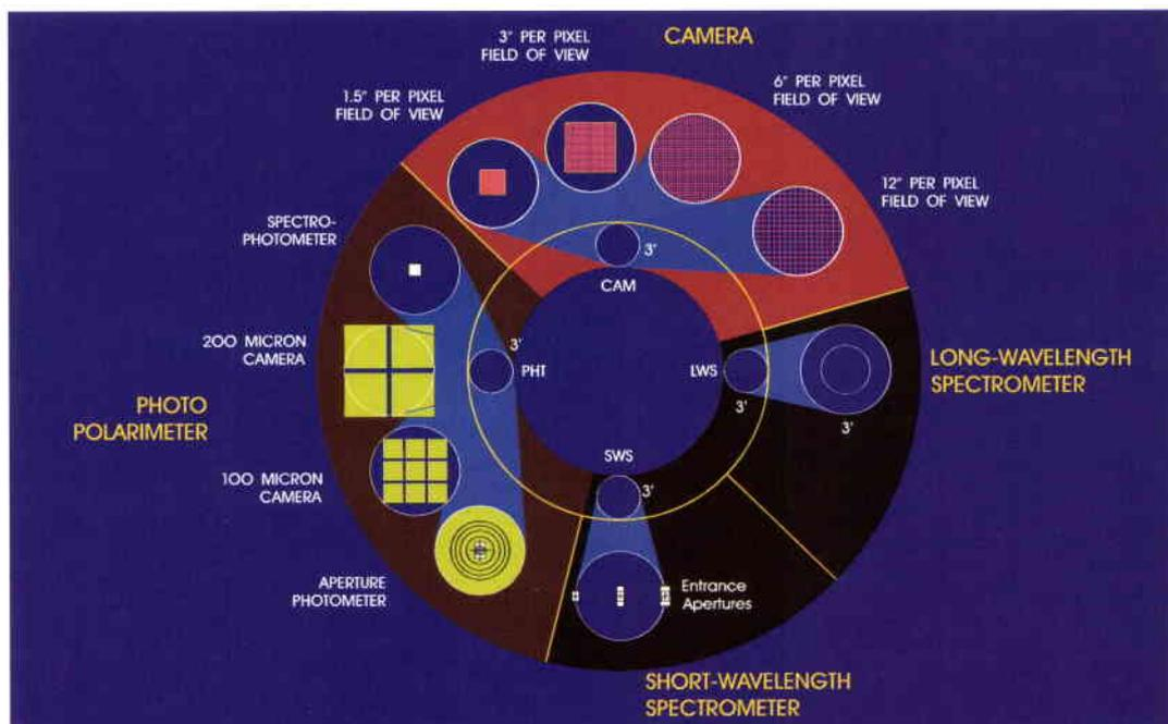
Figure 4. Imaging capabilities of the ISO scientific instruments. Each of the four instruments receives a circular 3 arcmin field of view (drawn to scale in the central part of the figure). The outer ring shows, in expanded scale, more details of the detector fields of view as projected onto the sky.
