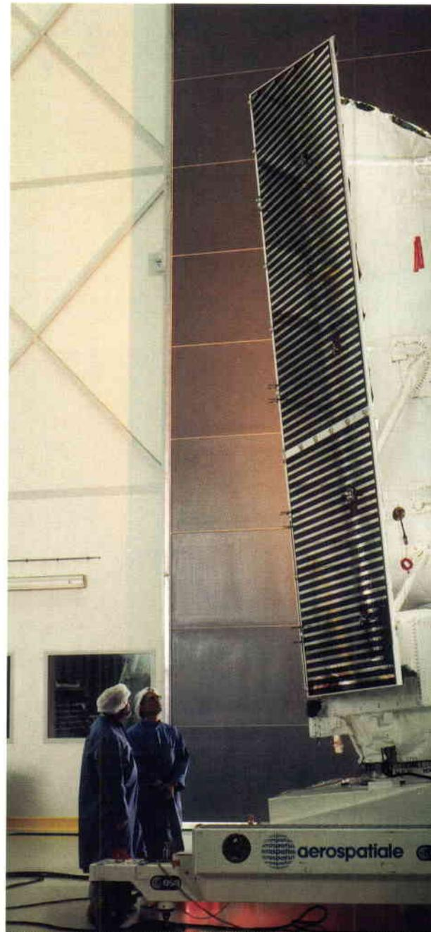
**Figure 6. ISO Payload Module undergoing testing at DASA, Ottobrun**
