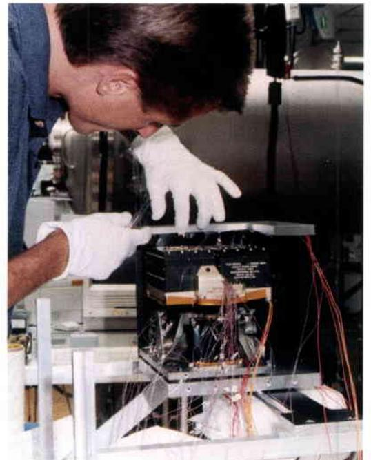
**Figure 4. One of the AOCS fine-pointing Sun sensors**
