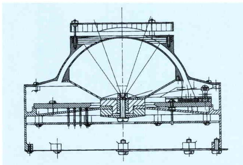
Figure 2b. The final mounting of the PEACE hemispheres
