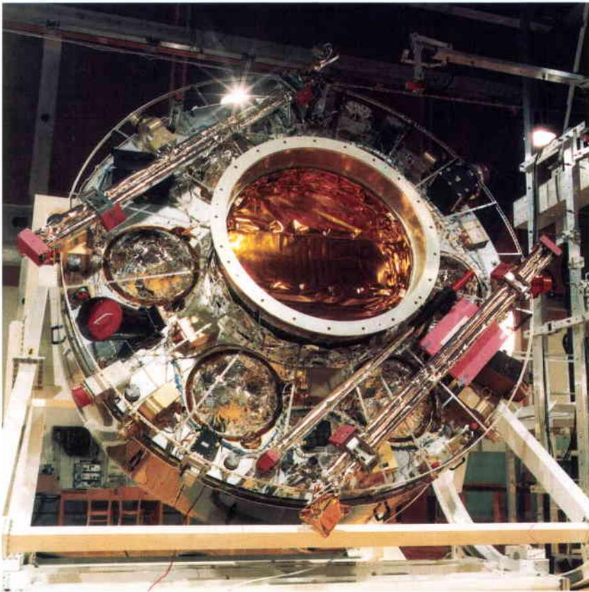
**Figure 1. Top view of a Cluster spacecraft, showing experiment accommodation around the periphery and on the stowed radial booms**
