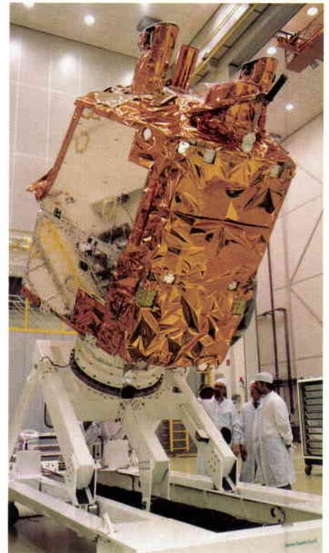
*The protoflight model of SAX, the Italian space agency ASI's X-ray Astronomy Satellite, undergoing final testing in ESTEC's Test Centre, in The Netherlands*
