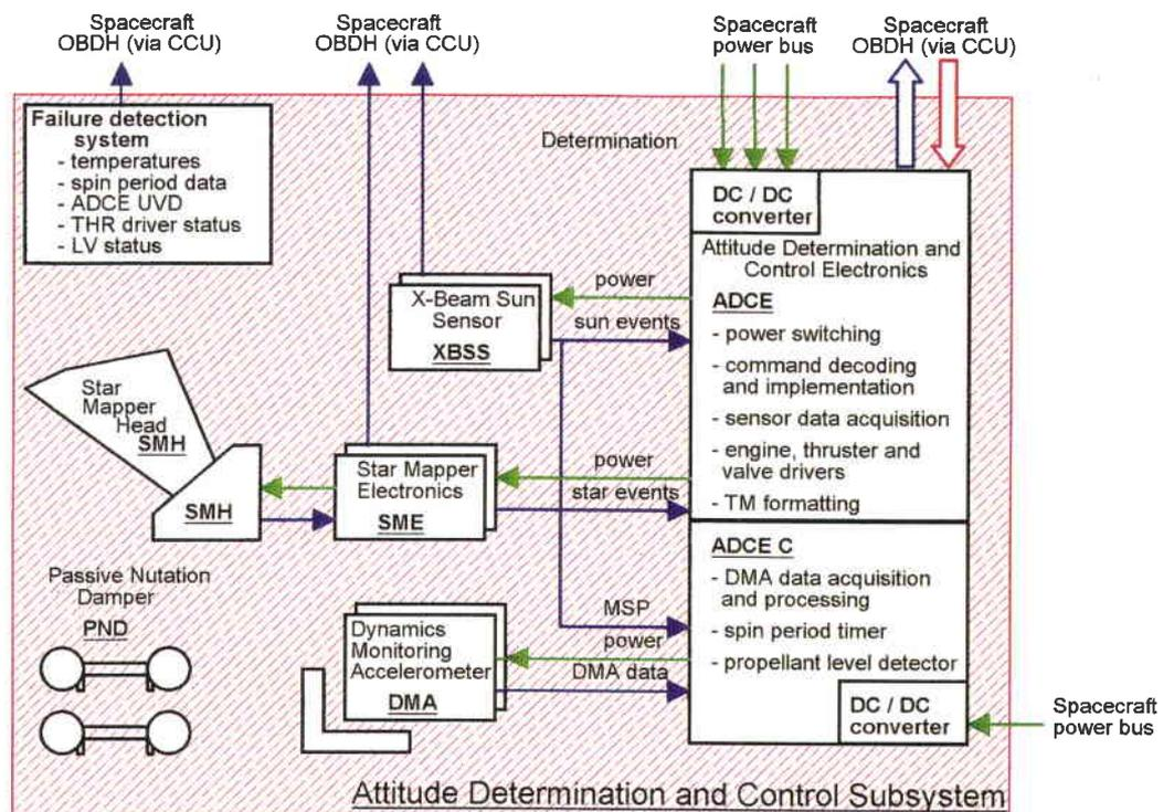
Figure 11. The Cluster attitude determination and control subsystem
