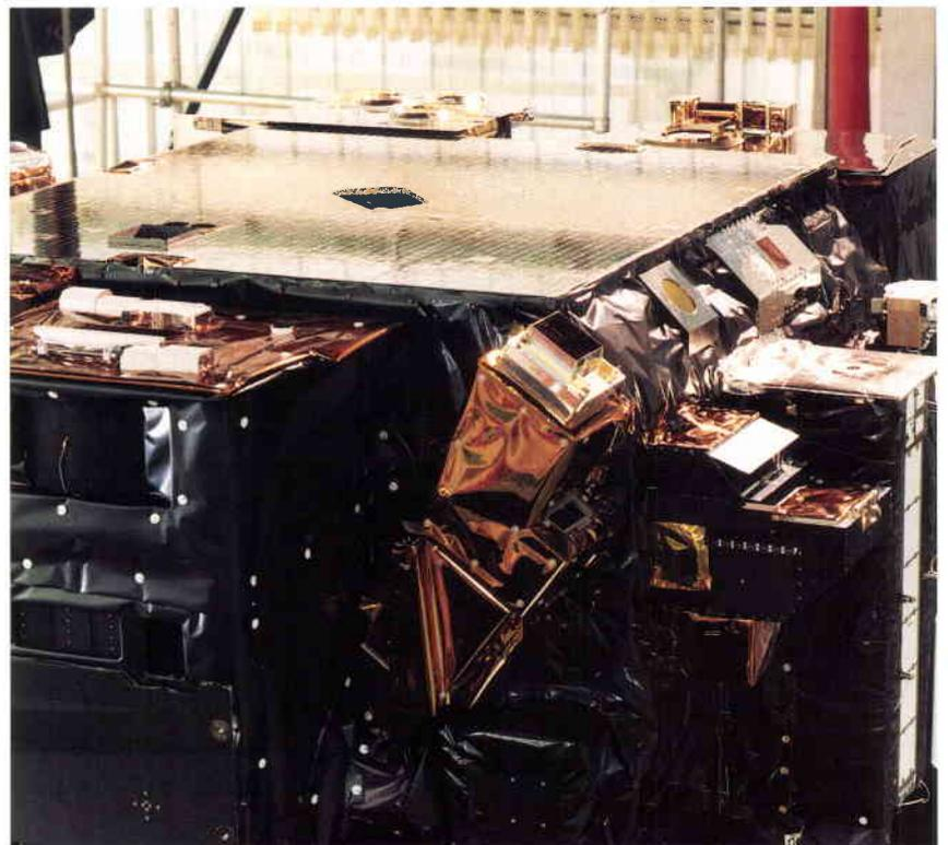
Figure 2. View of the upper face of the SOHO Payload Module prior to thermal-balance/thermal-vacuum testing, showing mainly particle sensors on the right and the OSRs of the Sun shield pierced by the apertures for the Sun sensors
