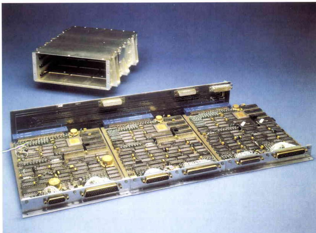
**Figure 7. The three printed-circuit boards of the DWP, including the three T222 transputers**
