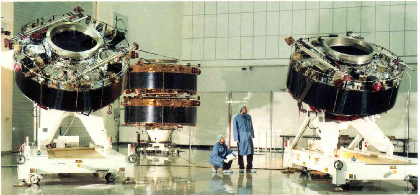
**Figure 1. The four Cluster flight-model spacecraft together for the first time in the cleanroom at IABG, Ottobrunn (D). Two spacecraft are shown complete with thermal hardware and stacked in launch configuration, whilst the other two are 'open' with the payload platform visible**
