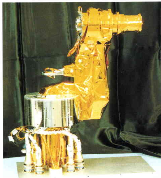
Figure 6a,b. Schematic of the APM (a), and its qualification model (b). (photo courtesy of Alcatel Espacio/Inta)
